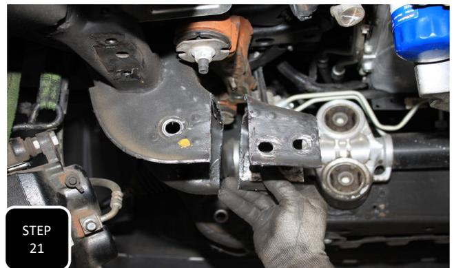
**Step 21** Working with the rearward lower control arm mount on the driver's side, mark a vertical line, 3 inches in from the inner edge where the original cross member was attached. Extend this mark straight up, across, and back down the front of the mount and then using a suitable cutting device, cut this section of the mount off.
