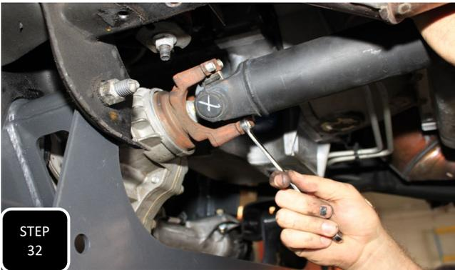
**Step 32** Attach the front driveshaft to the diff using the factory straps and bolts. **NOTE: IT IS NORMAL TO HAVE TO PULL THE DRIVESHAFT TO GET IT TO ATTACH TO THE YOKE.**
