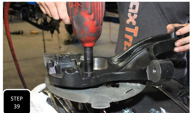
**Step 39** Place the factory hub assembly along with the factory dust shield onto the new steering knuckle and then flip the assembly over and attach the two together using the factory bolts and tighten.
