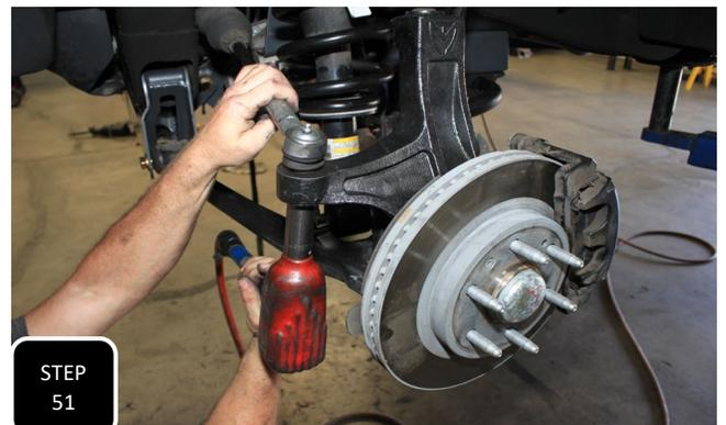
**Step 51** Once both ends are trimmed down, thread them back together and attach the tie rod to the steering knuckle using the factory nut.
