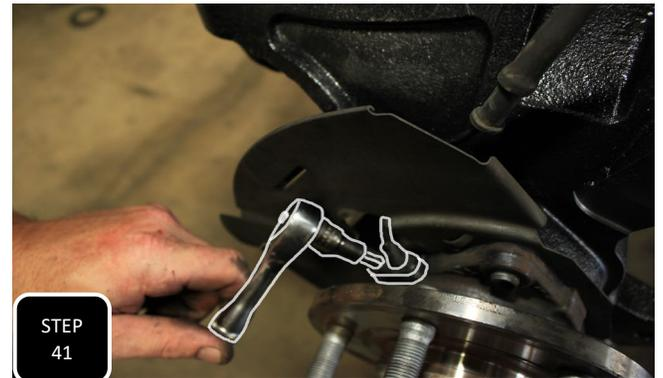
**Step 41** Unclip the ABS line from the frame, right next to where the brake line goes from soft to hard line. Next, use the extra slack gained to guide the ABS sensor down the steering knuckle and attach it to the wheel bearing using the factory bolt.
