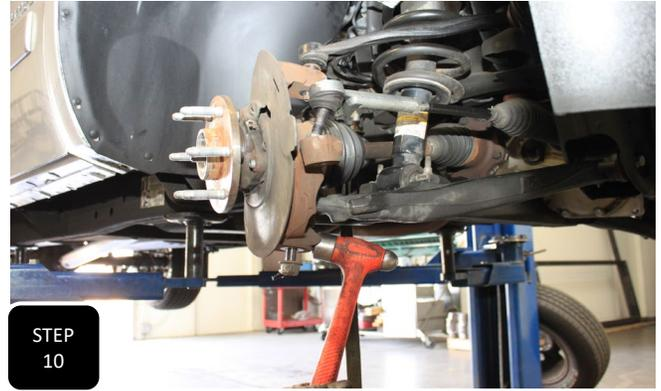
**Step 10** Loosen the lower ball joint nut, but do not remove. Next, hit the side of the spindle, right at the nut, with a hammer to break the ball joint loose. The nut will catch the spindle.
