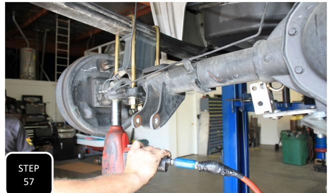
**Step 57** Loosely Install the provided U-bolts, from the top down and snug up the nuts under the factory spring plate. **NOTE: DO NOT FULLY TIGHTEN THE U-BOLTS UNTIL BOTH REAR BLOCKS HAVE BEEN INSTALLED. ONCE BOTH ARE INSTALLED, TORQUE THE U-BOLTS TO 100 FT/LBS.**
