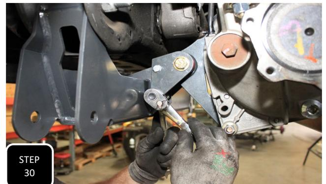
**Step 30** Attach the provided diff mounting ears to the back of the front subframe using the provided M8 hardware and then attach the diff to these ears using the provided 9/16" bolt, nut, and washers. Once all have been loosely installed, then fully tighten the diff ears and dorsal fin bolt. Next, fully tighten all of the diff bolts.
