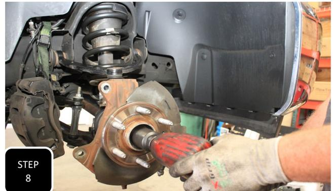
**Step 8** Pry off the dust cap at the end of the hub assembly and then remove the axle retainer nut.
