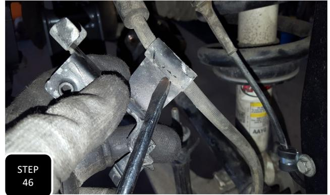
**Step 46** There is a mounting bracket on the middle of the soft brake line that needs to be removed. Very carefully, cut a groove in bracket where it wraps around the line. This will create a weak spot so you can use a flat head screw driver to pry the bracket open and remove it. **NOTE: BE VERY CAREFUL NOT TO CUT ALL THE WAY THROUGH THE BRACKET OR CUT THE LINE ITSELF.**
