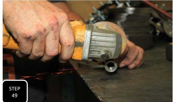
**Step 49** Remove the outer tie rod from the inner tie rod and mark a line 1/2" from the end of the threaded hole and cut this 1/2" section off. **NOTE: MAKE SURE YOUR CUT IS STRAIGHT SO THAT THE JAM NUT TIGHTENS UP PROPERLY.**
