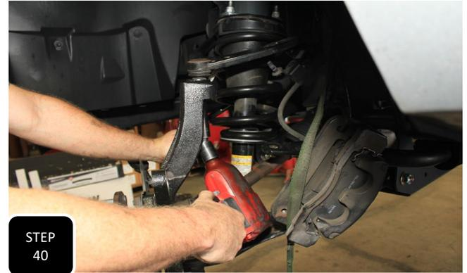
**Step 40** Install the steering knuckle assembly onto the the appropriate side that you are working on with the steering arm of the knuckle facing the front of the truck. Use the factory nuts at the upper and lower ball joints and tighten to factory specs. **NOTE: SLIDE THE AXLE INTO THE HUB BEFORE CONNECTING THE BALL JOINTS.**
