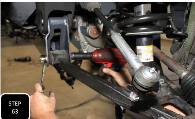
**Step 63** Now that the suspension is settled and the vehicle is sitting at ride height, go back and tighten all of the bolts that were left loose. **NOTE: TIGHTENING THE CONTROL ARM BUSHINGS AND DIFFERENTIAL WHILE THE TRUCK IS AT RIDE HEIGHT WILL ENSURE THE DIFF IS CENTERED AND PROLONG THE LIFE OF THE BUSHINGS.**
