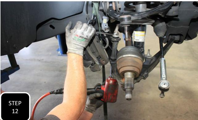
**Step 12** Unbolt the sway bar end link and remove.
