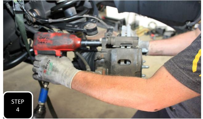
**Step 4** Unbolt the brake caliper and support it, up out of the way. **NOTE: NEVER ALLOW THE BRAKE CALIPER TO HANG BY THE BRAKE LINE.**
