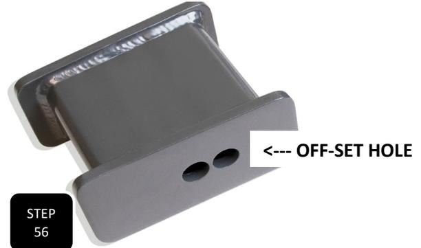
**Step 56** Install the new lift block. The lift block is angled and the short side must face the front of the truck. **NOTE: THE MAX TRAC LIFT BLOCK HAS TWO CENTER PIN HOLES. INSTALL THE CENTER PIN IN THE OFF-SET HOLE, WHICH WILL PUSH THE AXLE 1 INCH FORWARD AND MINIMIZE DRIVELINE PLUNGE.**
