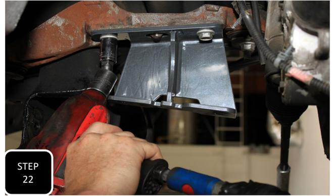
**Step 22** Locate the driver's side diff drop and install it to the factory mount using the factory hardware. The driver's side bracket has the tab that extends past the bracket and an extra hole for the guide nipple in the factory mount. **NOTE: THE SHORT SIDE OF THE MOUNT WILL FACE THE REAR OF THE TRUCK.**
