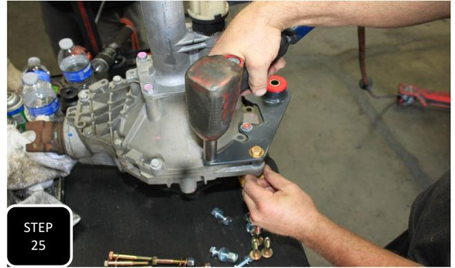
**Step 25** Remove the 4 bolts that the bracket aligns with and then install the bracket using the 4 provided M10-1.5 x 60 bolts and the 1 provided 7/16-14 x 3" bolt, nut, & washer then tighten. **NOTE: THE BRACKET WILL ONLY FIT ONE WAY AND ALWAYS TAKE CAUTION WHEN INSTALLING A STEEL BOLT INTO ALUMINUM THREADS.**
