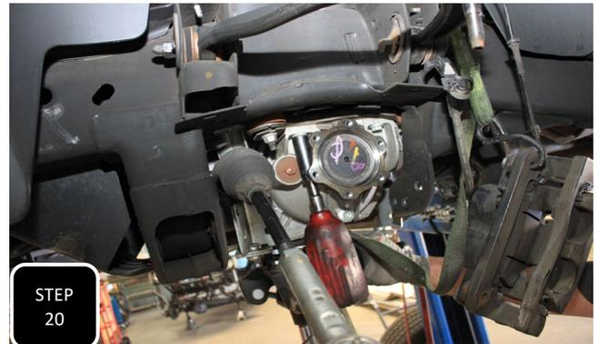
**Step 20** Support the differential with an adjustable jack and then remove all 4 mounting bolts. Slowly lower the diff down making sure that there is nothing else attached to it that could get damaged.
