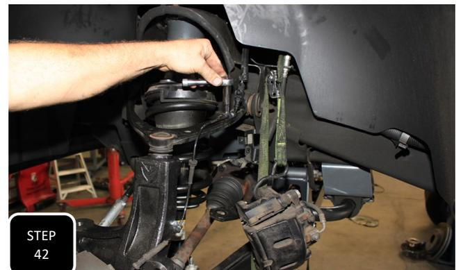
**Step 42** Using the provided loom clamps and factory 6 mm bolts, guide and attach the ABS line up the back side of the neck of the steering knuckle and to the upper control arm.
