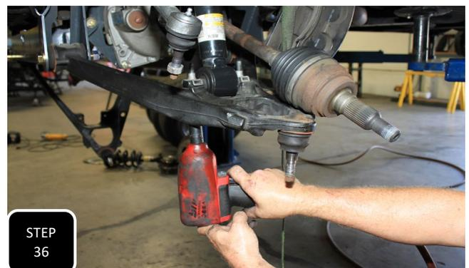
**Step 36** Loosely attach both lower control arms using the provided 5/8" hardware and then swing the arms up and loosely attach them to the bottom of the strut using the factory hardware. **NOTE: DO NOT FULLY TIGHTEN THE LOWER CONTROL ARM BUSHINGS UNTIL THE TRUCK IS BACK ON THE GROUND AT RIDE HEIGHT.**
