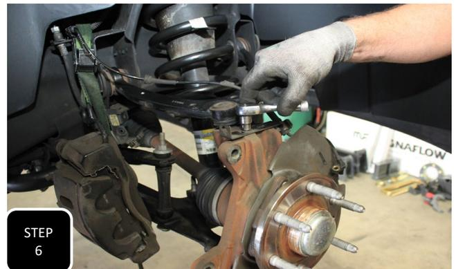
**Step 6** Unbolt the ABS sensor from the rotor and then the guide bracket from the top of the spindle. Support the ABS sensor out of the way so that it does not get damaged during the install.
