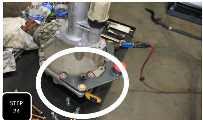
**Step 24** Take the differential and stand it upright on the driver's side axle flange. The breather port will leak a little if at a high point or a lot if at a low point. Place a vacuum cap over the breather for no fluid loss. Locate the provided dorsal fin diff bracket and line it up with the front side of the diff to see which bolts need to be removed.
