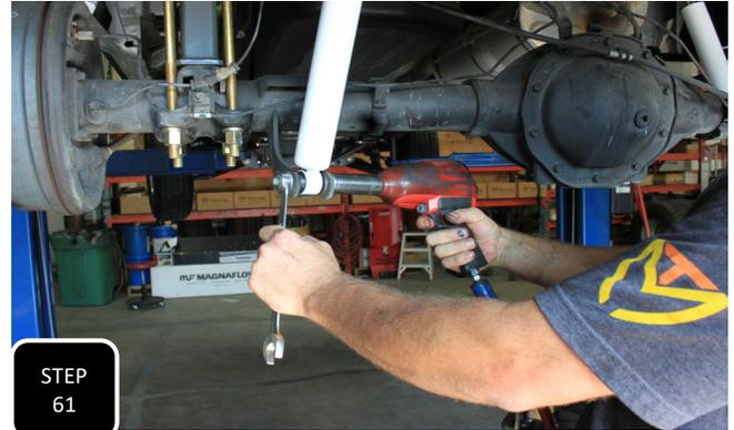
**Step 61** Install the new longer shocks using the factory hardware and tighten. **NOTE: MAX TRAC SHOCKS MUST BE MOUNTED WITH THE BODY AT THE AXLE AND THE SHAFT AT THE FRAME OR THEY WILL NOT WORK PROPERLY. FOX SHOCKS WILL MOUNT THE OPPOSITE, WITH THE BODY ON THE FRAME AND SHAFT AT THE AXLE.**
