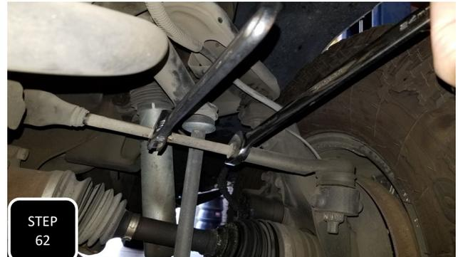
**Step 62** Install the new wheels and tires, then move the truck forward and back about 10 feet while moving the steering back and forth to settle the suspension. Next, adjust the vehicles toe alignment close to straight so that the vehicle is safe to drive to the alignment shop.
