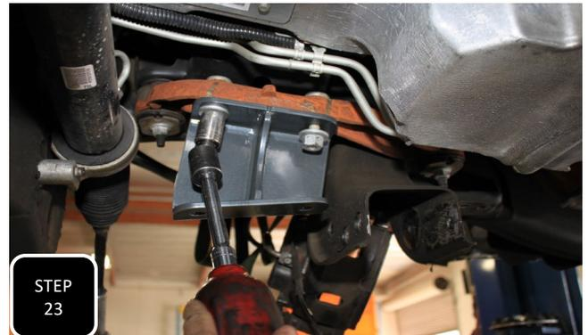
**Step 23** Locate and install the passenger side diff drop and attach it to the factory mount using the factory nuts, then tighten. **NOTE: THE SHORT SIDE OF THE MOUNT WILL FACE THE REAR OF THE TRUCK.**
