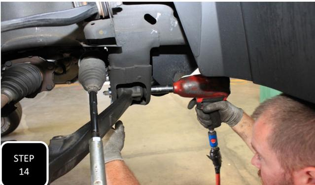
**Step 14** Unbolt both lower control arm mounting bolts and remove the lower control arm.
