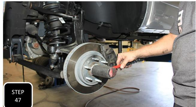
**Step 47** Install the axle retainer nut on both sides and torque to factory specs. Next, re-install the factory dust cap by tapping it into place with a mallet or dead blow hammer.
