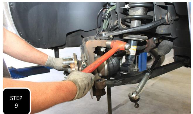
**Step 9** Loosen the upper ball joint nut, but do not remove. Hit the side of the spindle, right at the ball joint, with a hammer to break the ball joint loose. The nut will catch the spindle.
