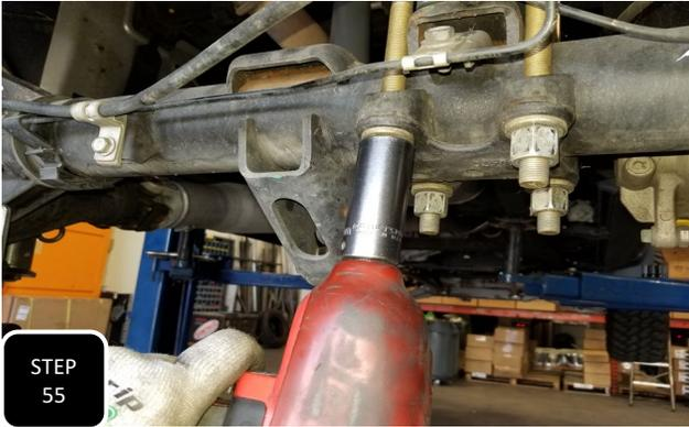
**Step 55** Working on one side at a time, remove the U-bolts and lower the axle down so that you have room to remove the factory lift block and insert the new one.
