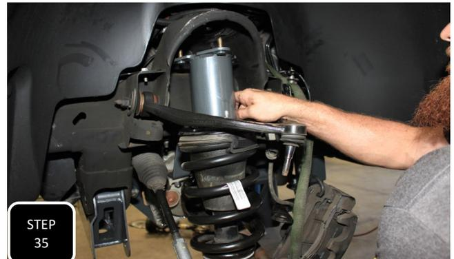
**Step 35** Locate the two struts and attach the strut spacer to the top using the factory nuts. Next, loosely install both sides using the provided nuts. **NOTE: THE SPACERS WILL ONLY FIT ONE WAY AND DO NOT FULLY TIGHTEN THE NUTS AT THE FRAME AT THIS TIME.**
