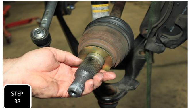
**Step 38** Slide the outer CV spacer onto the end of both axles with the chamfered I.D. side facing inward. The outer CV spacer is the 2 3/4" gold ring with a chamfered I.D. on one side.
