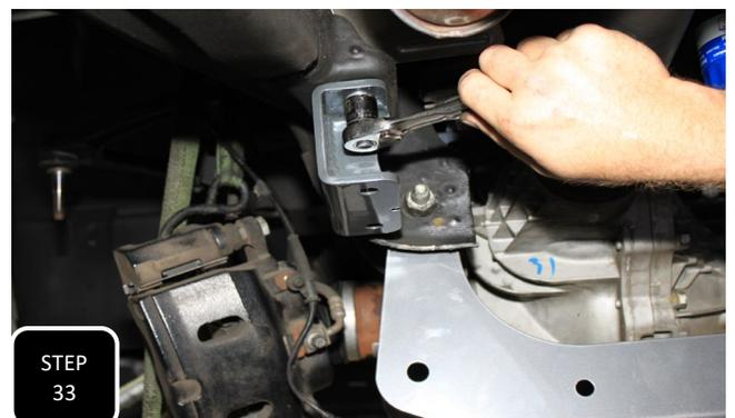
**Step 33** Install the sway bar drop down brackets using the supplied M10 bolts and washers. The open end of the bracket will face the inside of the truck and the bracket needs to swoop towards the rear of the truck.
