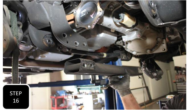
**Step 16** Unbolt the 4 bolts attaching the cross member to the rearward lower control arm mount and remove the cross member.
