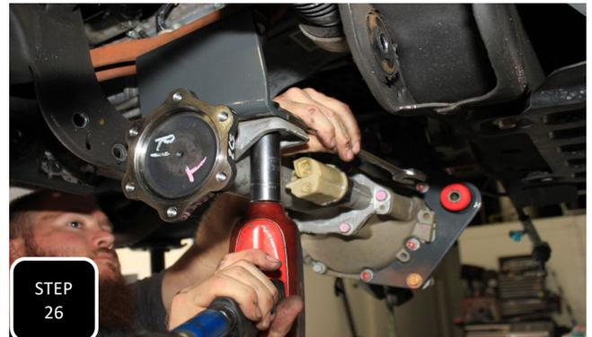
**Step 26** Place the differential back onto the adjustable jack and align it with the recently install diff drop brackets. Next, loosely attach the diff using the provided 1/2" bolts on the driver's side and 9/16" bolts on the passenger side. **NOTE: THE DIFF WILL GET FULLY TIGHTENED WHEN THE WHOLE FRONT END IS BACK TOGETHER.**
