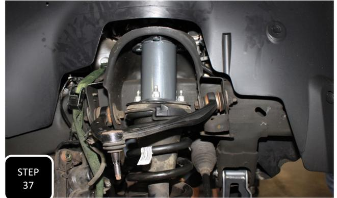
**Step 37** Fully tighten the upper mounting nuts and the lower mounting bolts for both struts.
