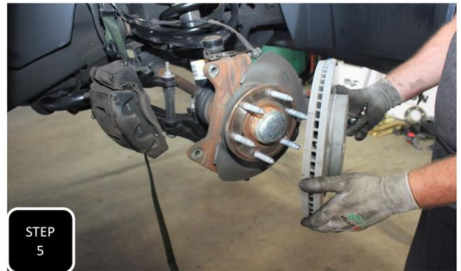
**Step 5** Unbolt the rotor retainer bolt and then remove the rotor. **NOTE: THE ROTOR SHOULD JUST POP OFF. IF IT DOES NOT JUST POP OFF, YOU WILL NEED TO HIT THE WHEEL MOUNTING SURFACE OF THE ROTOR WITH A HAMMER UNTIL THE RUSTY BOND IS BROKEN AND THE ROTOR POPS OFF.**
