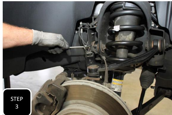
**Step 3** Separate the ABS line from the brake line bracket at the upper control arm and then unbolt the bracket from the control arm.
