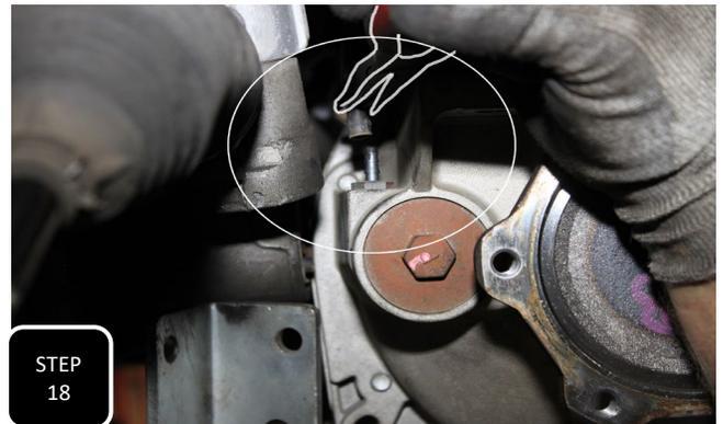
**Step 18** Remove all 4 bolts attaching the driveshaft to the front differential and then support the driveshaft up and out of the way. Next, detach the breather hose on the driver's side, top of the differential housing.
