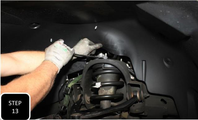
**Step 13** Remove the 3 nuts attaching the strut to the frame and the two bolts attaching the strut to the lower control arm, then remove the strut.
