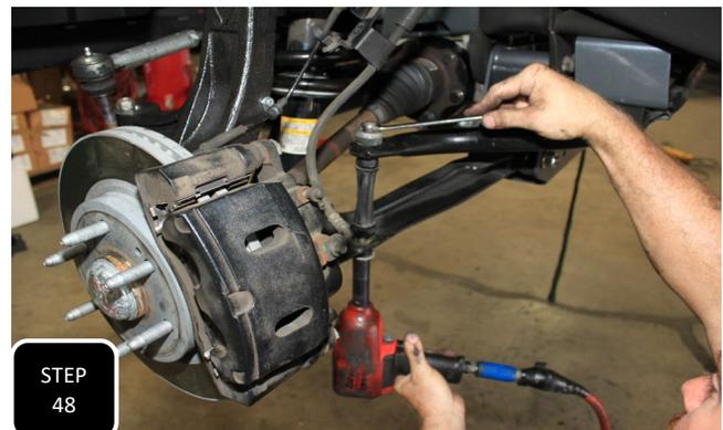
**Step 48** Assemble the sway bar end links onto the truck and then tighten them up until the nut bottoms out.
