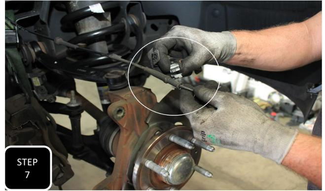
**Step 7** Separate the clip attaching the ABS line to the bracket you just removed from the top of the spindle and then open the clip and separate the ABS line from the clip.
