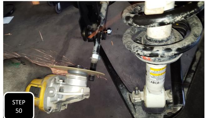
**Step 50** Mark a line 9/16" in from the threaded end of the inner tie rod and cut this section off. **NOTE: MAKE SURE TO CLEAN UP THE END SO THAT THE OUTER TIE ROD CAN THREAD BACK ON PROPERLY.**
