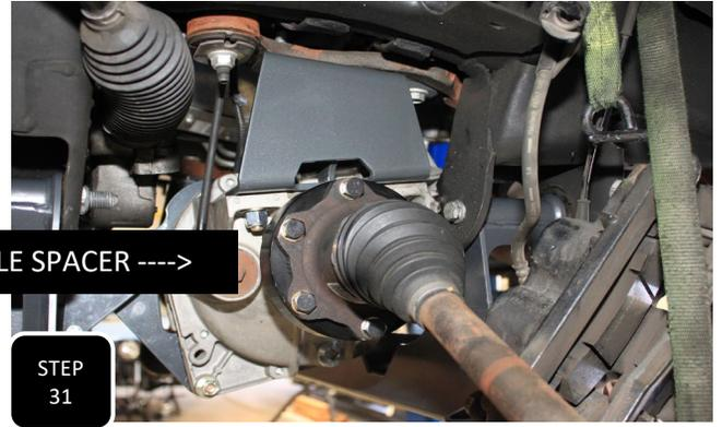
**Step 31** Using the provided M10 hardware, re-install both front axles with the aluminum spacers between the diff and axle.
