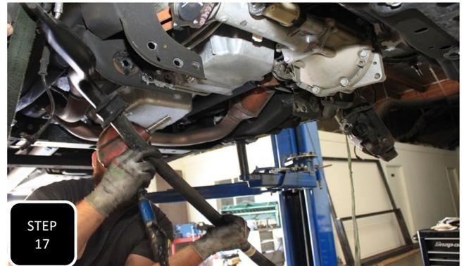
**Step 17** Unbolt the 4 bolts attaching the sway bar to the frame and remove the sway bar. **NOTE: TAKE NOTE THAT THE ENDS OF THE SWAY BAR SWOOP UPWARD. YOU WILL FLIP THIS OVER SO THEY SWOOP DOWNWARD WHEN THE SWAY BAR IS RE-INSTALLED.**
