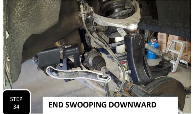
**Step 34** The ends of the sway bar originally swooped upward. The sway bar will now get re-installed with the ends swooping downward, the opposite of how they were. Use the factory bolts along with the provided nuts and washers to attach the sway bar to the drop down brackets and tighten.
