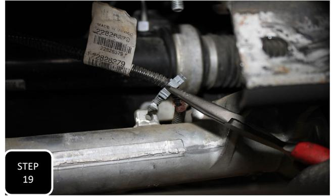
**Step 19** Unplug the wiring at the differential and separate the wire guide clip. Move the wiring up out of the way so that it does not get damaged during the install.
