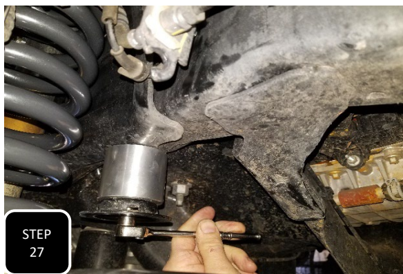
Step 27 Locate the provided bump stop extensions and install them between the bump stop mounting cup and the frame using the supplied M8-1.25 x 75mm bolts and torque to 18 ft/lbs. Next, spray some WD-40 on the bump stop and pop it back into the mounting cup.
