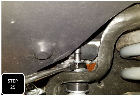
Step 25 Tighten up both ends of both front shocks.
