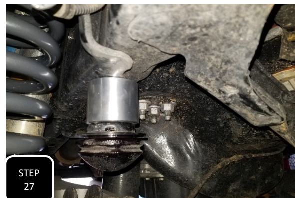
Step 27 Locate the provided bump stop extensions and install them between the bump stop mounting cup and the frame using the supplied M8-1.25 x 75mm bolts and torque to 18 ft/lbs. Next, spray some WD-40 on the bump stop and pop it back into the mounting cup.
