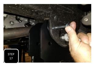
**Step 17** Loosely install the 4 link bracket using the factory M18 bolt at the large hole and the provided 3/8-16 x 4 1/2" bolt at the small hole. **NOTE: SOME MODELS HAVE A FACTORY BRACKET TO WHICH THIS HOLE IS SHIFTED FURTHER THAN THE RANGE OF OUR SLOTTED HOLE. THAT IS FINE, JUST OMIT INSTALLING THIS BOLT. IT IS JUST FOR REFERENCE**
