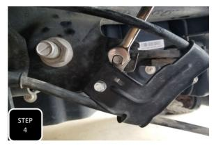
**Step 4** On the driver's side near the front spring hanger is a bolt on E-brake bracket. Unbolt this and install the provided extension bracket using the factory bolt at the frame and the provided M8 bolt, nut, and washers at the bracket.
