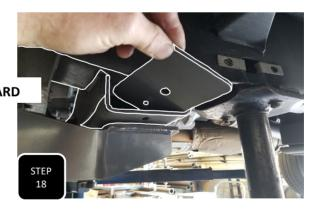
**Step 18** Locate the flat plate labeled DS and slide it into the cross member above the back of the 4 link bracket. Line up the hole and loosely attach the plate and bracket together using the provided M12-1.5 x 40 socket head allen bolt. **NOTE: THE DRIVER'S SIDE IS THE LONGER PLATE**
