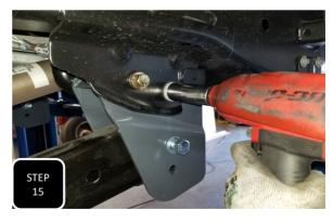
**Step 15** Repeat steps 11-14 on the passenger's side and then tighten the bolts attaching the bracket to the frame, the M18 bolt gets torqued to 200 ft/lbs, the 3/8" to 50 ft/lbs and the M12 socket head bolt to 50 ft/lbs. The radius arm bolts will not get tightened until the truck is on the ground at ride height.
