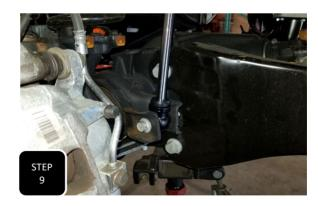
**Step 9** Loosely attach the new shock to hold the axle, then move the jack to the passenger side and repeat steps 7-9. **NOTE: THE SHOCKS WILL HOLD THE AXLE AS YOU MOVE THE JACK AND CONTINUE THROUGH THE INSTALL.**
