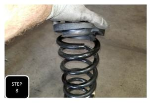
**Step 8** Lower down the axle and remove the coil. Separate the rubber isolator and save for use on the new coils.
