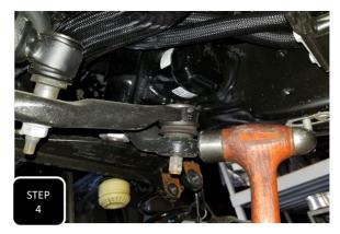
**Step 4** Remove the castle sleeve and cotter pin over the drag link nut. Next, remove the nut and break the joint loose by hitting the side of the pitman arm with a hammer. **NOTE: NEVER HIT THE ROD END ON THE THREADS.**
