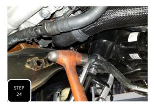
**Step 24** Using a 46mm socket, remove the pitman arm mounting nut. Next, apply tension to the arm using a pitman arm puller or a suitable 3 jaw puller. Hit the side of the pitman arm, right at the steering shaft, with a hammer a few times, very hard and then tighten down the puller some more. Proceed doing this until the pitman arm separates from the steering box. **NOTE: BE CAREFUL NOT TO DAMAGE THE STEERING BOX OR STEERING SHAFT.**
