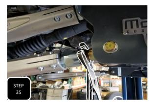
**Step 35** Tighten down all 4 of the M8 pinch bolts and then cinch down the two jam nuts on the rod ends. **REPEAT STEPS 21-32 ON THE OTHER SIDE.**
