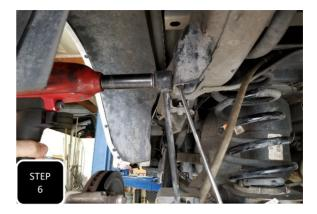
**Step 6** Unbolt the sway bar end links from the frame on both sides and spin them out of the way. Next, unbolt the air bags from the axle and lower the axle.
