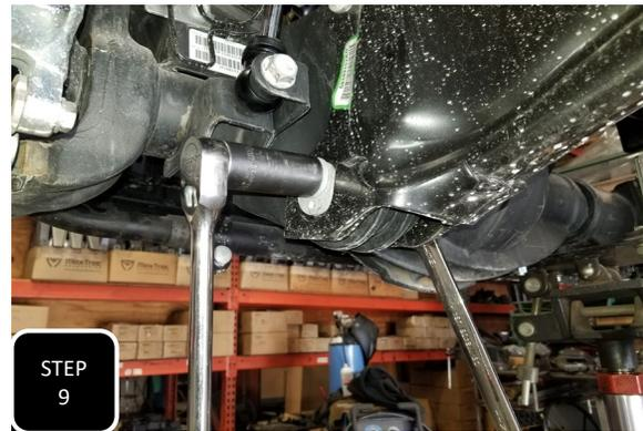
**Step 9** Loosen all 3 radius arm mounting bolts on both sides, but do not remove them.
