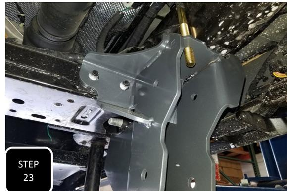
**Step 23** Locate the appropriate side 4link bracket so that when installed the Max Trac logo faces outward and the 2 holed side bracket faces inward. Loosely install the bracket using the factory radius arm bolt at the main hole, slide the two cross member bolts forward, and align the U-bolt with the top holes.
