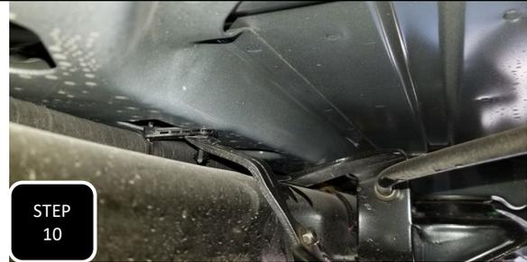
**Step 10** For the driver's side, you will need to create space between the wire harness on top of the frame and the module on the inside of the frame by prying the christmas tree retainer clips from the frame.
