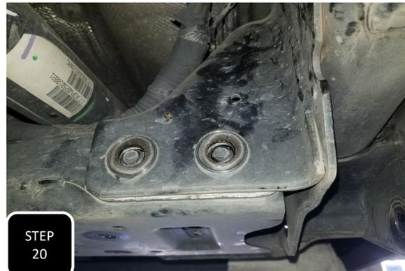
**Step 20** Remove the mounting nuts for the cross member just inside the radius arm bracket and push the bolts back so that the heads are not sticking out of the cross member.
