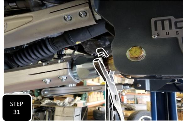
**Step 31** Tighten down both lower arm, M8 pinch bolts and then cinch down the two jam nuts on the rod ends.
