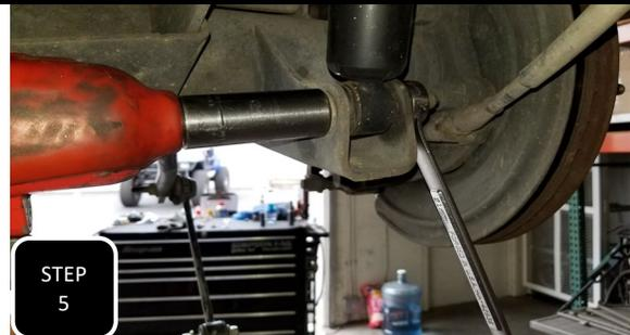
**Step 5** Install the new shocks and tighten using factory hardware at the bottom. **NOTE: MAXTRAC SHOCKS ARE A TWIN TUBE SHOCK THAT NEEDS TO BE FULLY CYCLED BEFORE INSTALL SO FULLY COMPRESS THEM & LET THEM REBOUND ABOUT 2-3 TIMES.**
