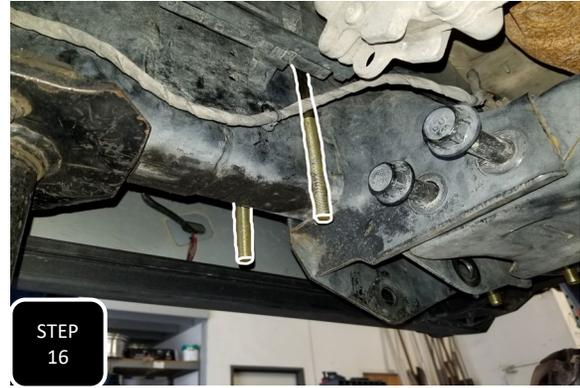
**Step 16** For the passenger side, slide the supplied U-bolt over the frame, just behind the cross member behind the factory radius arm bracket and allow it to hang vertically.
