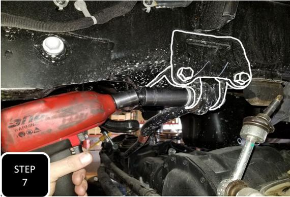
**Step 7** Remove the bolt attaching the trac bar to the bracket on the frame and separate. Allow the trac bar to rest on the axle.
