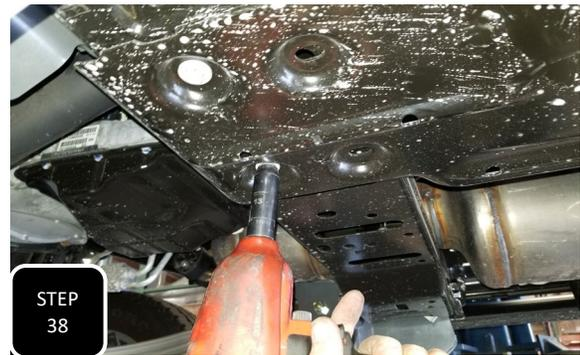
**Step 38** Re-attach the brake line brackets to the top of the axle and ensure that the brake lines are not tight when the suspension is at full droop. Next, re-install the skid plate under the transfer case and tighten.
