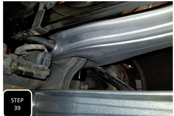
**Step 39** Re-install the wheels and tires then lower the truck to the ground. Once at ride height, tighten down the links to the axle. All 4 bolts will get torqued to 200 ft/lbs. **NOTE: IF INSTALLING THE RADIUS ARM KIT YOU WILL ALSO TIGHTEN THE BOLT AT THE FRAME BRACKET NOW, 6 BOLTS TOTAL FOR RADIUS ARM BRACKETS.**
