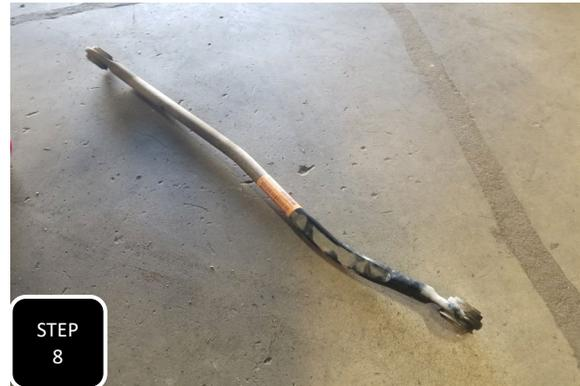
**Step 8** Unbolt the trac bar from the axle and completely remove the trac bar. Save the hardware for re-installation.
