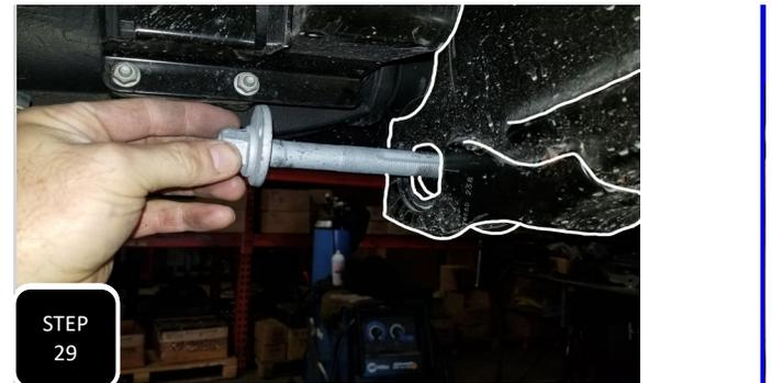
**Step 29** Loosely attach the links to the axle using the provided M18 bolts. After the first link is attached, you will want to remove one of the radius arm bolts, at the axle, on the other side so that the axle can be slightly rotated to attach the second link.
