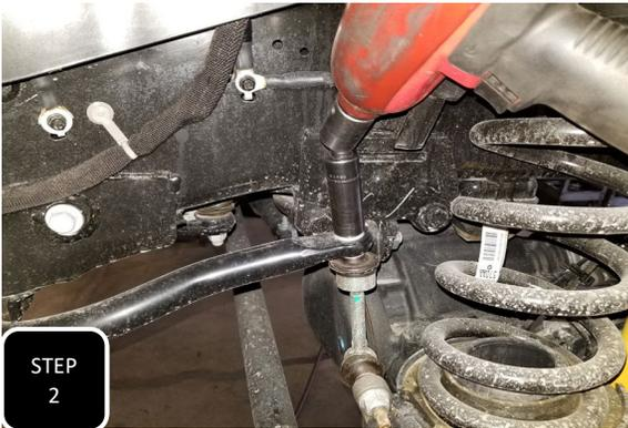
**Step 2** Unbolt the sway bar from both end links and save the nut for re-installation.
