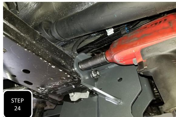
**Step 24** First snug up the U-bolt nuts, then the cross member bolts, and lastly the original radius arm bolt. Once all is snug and the bracket is up in place, go back and torque all bolts to factory specs. The U-bolt should get torqued to 100 ft/lbs.
