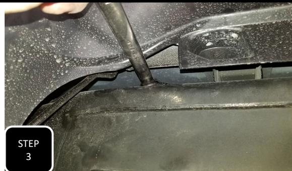
**Step 3** The top of the shock on Ram 2500's is a standard stem that is hidden behind the plastic wheel well liner. Using a knife, cut a clean opening for access to the stem nut and remove the shock.
