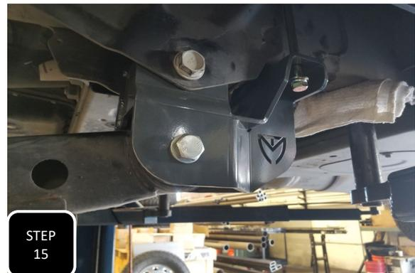
**Step 15** Loosely install the radius arm using the factory bolts at the axle and the provided M18 x 130 bolt at the bracket.
