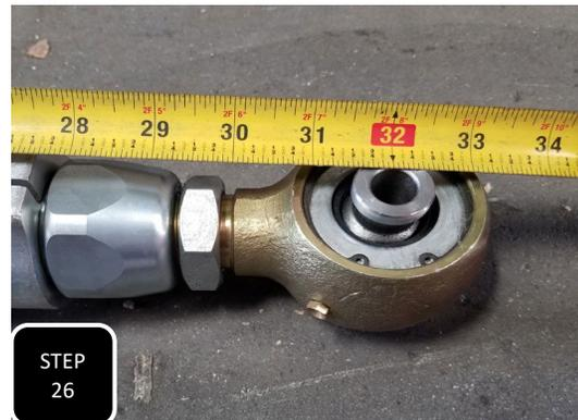
**Step 26** Adjust the upper links to 28.5" (the shorter link) and the lower links to 31 5/8" (the longer link). Now locate the links for the side that you are working on first. The driver's side links, when installed will have the Max Trac logo facing upright and the two pinch bolts facing outward when installed. **NOTE: THE ROD ENDS ARE NOT PRE-GREASED AND REQUIRE GREASE FOR PROPER FUNCTION.**
