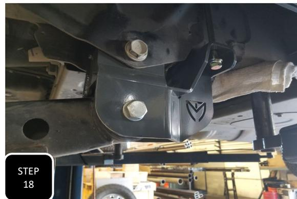
**Step 18** Loosely install the radius arm using the factory bolts at the axle and the provided M18 x 130 bolt at the bracket.
