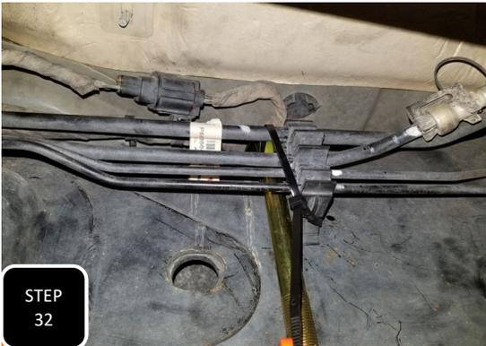
**Step 32** Use the supplied zip tie to attach the fuel line assembly to the U-bolt.
