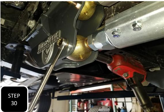
**Step 30** Tighten down the frame side bolts of the links completely and the axle side only hand tight. The axle side will get fully tightened when the truck is back on the ground at ride height. Torque the rod end bolts to 100 ft/lbs.
