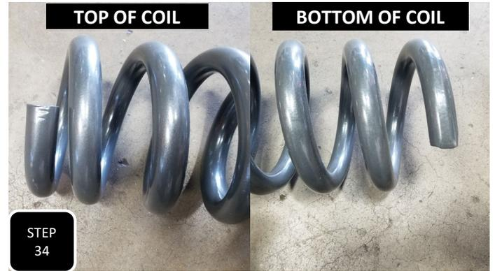
**Step 34** Place the rubber isolator on top of the new coil and install the coil. Make sure the nipple on the isolator aligns with the hole in the coil bucket then jack up the axle so that pressure is applied and re-attach the shock. **NOTE: THE COIL NEEDS TO BE INSTALLED WITH THE FLATTER SIDE FACING UPWARD AND THE PART # RIGHT SIDE UP.**
