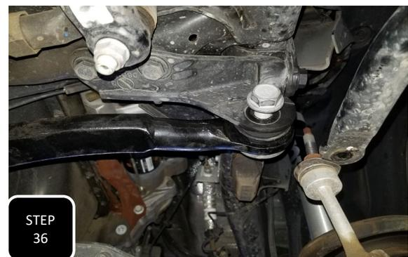
**Step 36** Loosely install the new adjustable trac bar using the factory hardware. The stamped arc in the trac bar needs to be towards the frame so that the trac bar clears the diff. Do not fully tighten the bolts yet. **NOTE: USE THE ADJUSTABILITY OF THE TRAC BAR FOR EASE OF INSTALLING THE BOLTS, BUT DON'T WORRY ABOUT FINAL ADJUSTMENTS UNTIL THE TRUCK IS ON THE GROUND AT RIDE HEIGHT.**
