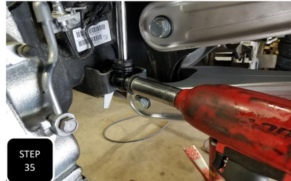
**Step 41** Repeat steps 33-34 on the other side and then tighten the top and bottom of both shocks.
