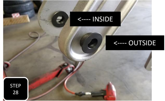
**Step 28** Loosely attach both links to the 4link bracket first using the provided 9/16" bolts and then install the provided machined, hat looking, sleeves on the other end of the link with 1 hat inside the clevis and 1 hat on the outside.
