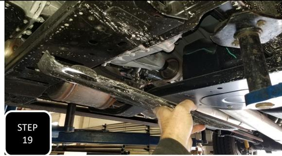
**Step 19** Unbolt and remove the skid plate under the transfer case and set aside to be re-installed later.
