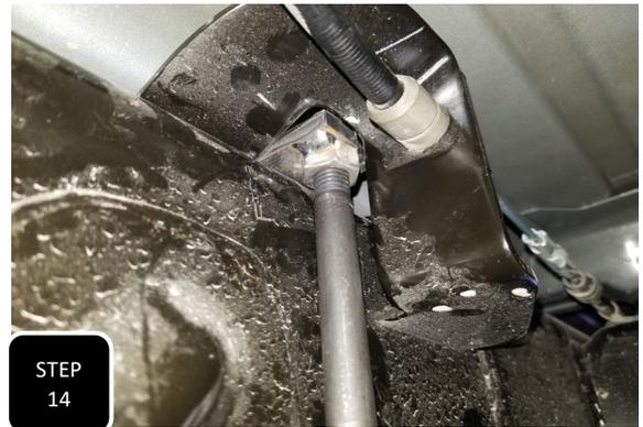
**Step 14** Loosely attach the provided 1/2-13 x 9" bolts, washers, and lock washers to the nut plate on top of the frame. Push the bracket up tight to the frame and torque the factory bolt to factory specs and the 1/2" bolts to 90 ft/lbs.
