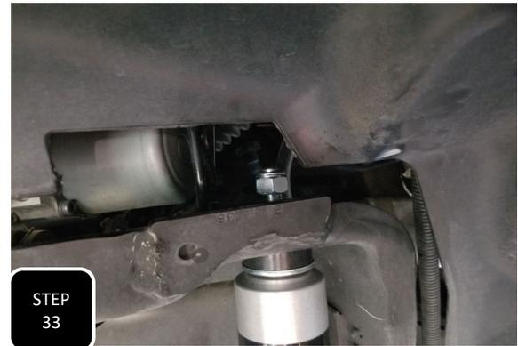
**Step 33** Move the jack to the driver's side of the axle and apply pressure. Remove the nut at the top of the shock and lower the axle to make room for the new coil.
