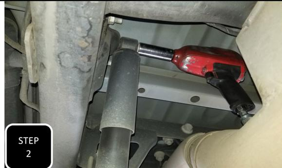
**Step 2** The top of the shock on Ram 3500's is a standard loop with a bushing. Remove the nut and then the shock.
