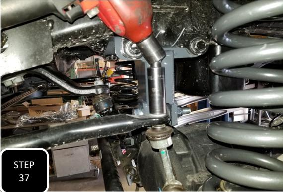
**Step 37** Attach the sway bar to the factory end links and tighten using the factory nuts.
