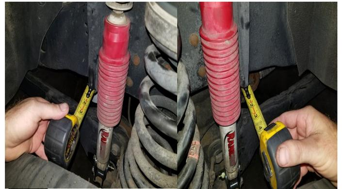
**Step 41** Loosen up the bolts for the clamps on the trac bar. Next. Find consistant measurement spots between each front tire and the frame, then adjust the trac bar until your measurements on both sides are equal then tighten down the clamp bolts.
