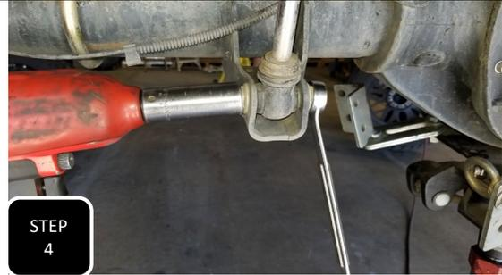
**Step 4** Install the new shocks and tighten using factory hardware. Max Trac shocks need to be installed with the shaft of the shock at the frame and the body at the axle. Fox shocks get installed opposite of that. **NOTE: MAXTRAC SHOCKS ARE A TWIN TUBE SHOCK THAT NEEDS TO BE FULLY CYCLED BEFORE INSTALL SO FULLY COMPRESS THEM & LET THEM REBOUND ABOUT 2-3 TIMES.**
