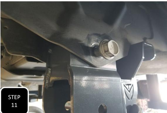
**Step 11** Loosely install the radius arm drop down bracket using the factory bolt.
