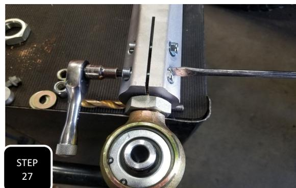
**Step 27** The upper links will not require any further adjustment so tighten down the pinch bolts now. Use a flat head screw driver, wedged between the nut and wall of the hole, to hold the nut from spinning. **NOTE: THE GAP BETWEEN THE UPPER ARM AND FRAME WILL BE VERY TIGHT AND MAKE IT VERY DIFFICULT TO TIGHTEN THESE PINCH BOLTS AFTER THE ARM IS INSTALLED.**
