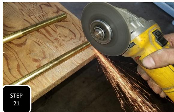
**Step 21** Locate the provided 9" long, square U-bolts for the 4link brackets, mark a cut line 1/2" down the threads of "only" one side, then cut that leg off the U-bolt on that line so that it is 1/2" shorter.
