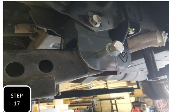
**Step 17** Loosely install the radius arm drop bracket using the factory bolt and push the bracket up tight against the frame, then tighten the U-bolt first. Next, torque the factory bolt to factory specs and the U-bolt to 100 ft/lbs.
