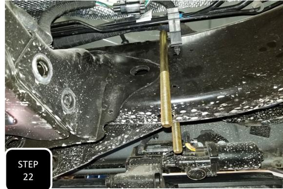
**Step 22** Working at the front of the cross member, pry the plastic fuel line guide bracket away from the frame and install the provided U-bolt over the frame from the top down with the shorter leg of the U-bolt on the inside of the frame.
