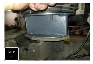
**Step 9** Remove the lower mounting nuts on both air bags, lower the axle and then install the air bag spacers under the air bags with the short side of the spacer facing the front of the truck. The round plate on the spacer will face up and attach to the air bag while the side of the spacer with the flat sides will bolt up to the axle.
