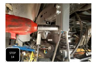
**Step 14** Attach the sway bar drop down bracket to the factory sway bar bracket using the provided 7/16" hardware and tighten. Next, attach the sway bar end link to the new bracket using the factory hardware and tighten. Repeat on other side.
