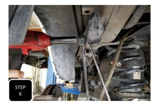
**Step 6** Unbolt the sway bar end links from the frame on both sides and spin them out of the way.
