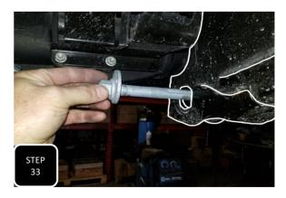
**Step 33** Loosely attach the links to the axle using the provided M18 bolts. After the first link is attached, you will want to remove one of the radius arm bolts, at the axle, on the other side so that the axle can be slightly rotated to attach the second link.
