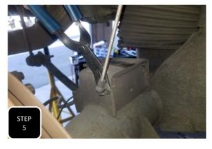
**Step 5** Disconnect the sensor rods from the axle using a suitable pry tool. The plastic rod end will pop off of the metal mounting ball with a good amount of pry force.
