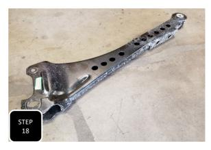
**Step 18** Starting with the passenger side, remove the previously loosened radius arm bolts and then remove the radius arm. **NOTE: ONLY REMOVE ONE RADIUS ARM AT A TIME.**
