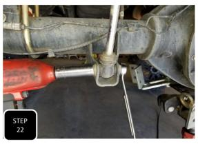
**Step 22** Install the new shocks and tighten. Max Trac shocks need to be installed with the shaft of the shock at the frame and the body at the axle. Fox shocks get installed opposite of that.
