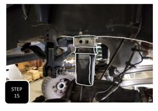
**Step 15** Attach the new bump stop bracket to the frame using the provided 1/2" bolts and then attach the factory bump stop cup to the new bracket using the provided 3/8" bolts, nuts, & washers. Next, spray some WD-40 onto the provided bump stop and pop it into the factory cup. **NOTE: JACKING UP THE AXLE AND USING IT TO PRESS THE BUMP STOP IN THE CUP WILL MAKE THIS MUCH EASIER.**
