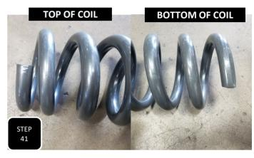
**Step 41** Place the rubber isolator on top of the new coil and install the coil. Make sure the nipple on the isolator aligns with the hole in the coil bucket then jack up the axle so that pressure is applied and re-attach the shock. **NOTE: THE COIL NEEDS TO BE INSTALLED WITH THE FLATTER SIDE FACING UPWARD AND THE PART # RIGHT SIDE UP.**
