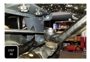
Step 39 Attach the tie rod to the pitman arm from the bottom up and tighten.
