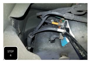
**Step 4** Locate the air ride valve block on the passenger side frame rail and crack open the two lines leading to the rear air bags to bleed the air out of them. Once the bags have been deflated, tighten up both fittings.
