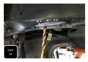
**Step 14** Drill out the holes in the frame using a 7/16" drill bit and then tap both holes using a 1/2-13 thead tapper.
