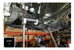
**Step 7** Now that both coils are removed, loosen all 3 radius arm mounting bolts on both sides, but do not remove them.
