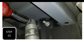
**Step 15** Jack up the rear of the truck and support under the frame with jack stands. Apply pressure to the rear diff with an adjustable jack and remove both rear shocks.
