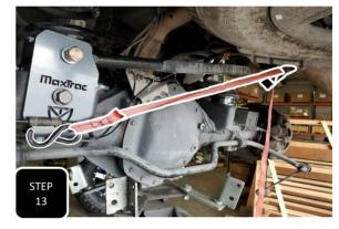
**Step 13** Use a rachet strap to pull the axle over and align the trac bar with the hole in the new bracket then loosely attach with the provided square plates and M14 bolt.
