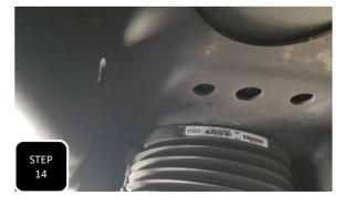
**Step 14** Install the wheels/tires and lower the vehicle down to the ground, but with the lift still holding the weight of the vehicle. First, ensure that the top of the air bag is properly aligned in the guide hole of the frame and then, second, turn the ignition on and allow the air bags to fill up before lowering the lift completely to the ground.
