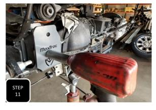
**Step 11** Tighten down the 3/8" bolt at the bottom of the trac bar bracket. The easiest way to hold the head of the bolt tight is to wedge a flat head screw driver down against the head. Next, tighten down the bolt in the original trac bar mounting hole.
