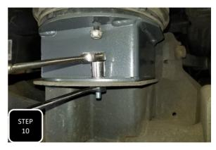
**Step 10** Tighten down the studs at the air bags using the factory nuts. Next, attach the spacers to the axle using the provided M8 bolts, nuts and washers then tighten.
