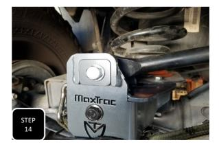
**Step 14** The plates with the off-center hole will get installed with the bolt towards the passenger's side for the 8" lift. Its only off-set to the drive side for the 4" & 6" lift. **NOTE: DO NOT TIGHTEN UNTIL THE TRUCK IS ON THE GROUND AT RIDE HEIGHT.**
