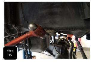
**Step 15** Using a suitable cuting device, cut the welds of the factory bump stop cup and then hit it with a hammer to break it loose. **NOTE: TRY NOT TO DAMAGE OR DISTORT THE CUP AS IT NEEDS TO BE RE-USED.**
