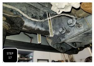
**Step 17** On the passenger side, slide the supplied U-bolt over the frame, just behind the cross member behind the factory radius arm bracket and allow it to hang vertically.
