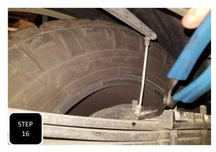
**Step 16** Unbolt both air bag bolts on the side you are working on and then disconnect the sensor rod from the spring plate by popping the socket off of the mounting ball.
