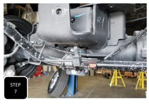
**Step 7** Disengage the guide clip attaching the brake line to the bottom of the trac bar bracket and pull down a bit so it is out of the way.
