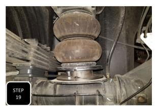
**Step 19** Before jacking up the axle and seating the block/air bag spacer, insert the new mounting bolts into the bottom plate from the top down and get the nut started on factory stud. **NOTE: WITH THE 1.5" REAR LIFT, THERE WILL NOT BE ROOM TO INSERT THE NEW BOLT WHEN THE STUD IS COMPLETELY INSERTED.**
