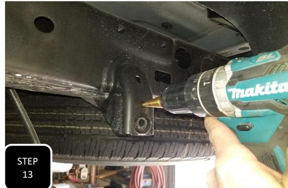
**Step 13** Loosely attach the sway bar drop down bracket to the factory bracket on the frame and mark the upper hole for drilling. Remove the bracket and drill a 7/16" hole on your mark. **NOTE: USING A STEP BIT WILL SPEED UP THE DRILLING.**
