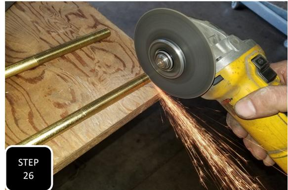
**Step 26** Locate the provided 9" long, square U-bolts for the 4link brackets, mark a cut line 1/2" down the threads of "only" one side, then cut that leg of the U-bolt on that line so that it is 1/2" shorter.
