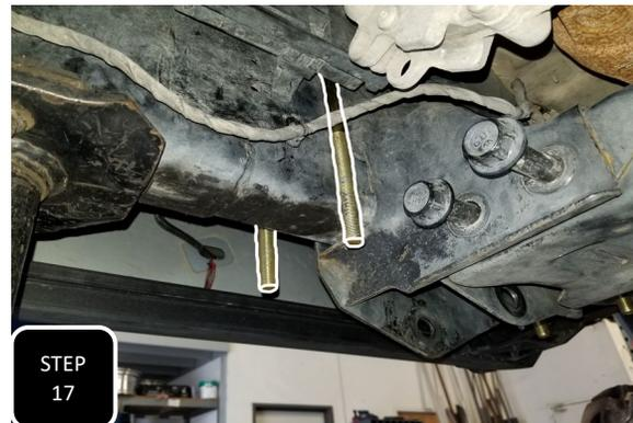
**Step 17** On the passenger side, slide the supplied U-bolt over the frame, just behind the cross member behind the factory radius arm bracket and allow it to hang vertically.
