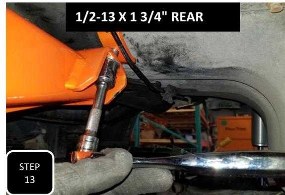
**Step 13** Slide the trac bar attachment plate between the oil pan and the cross member and loosely attach with the provided 1/2-13 x 1 1/2" bolt at the front and 1/2-13 x 1 3/4" bolt at the rear. Next, tighten down all 4 mounting bolts.
