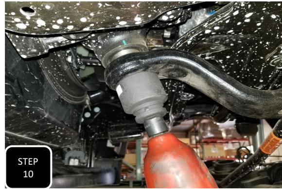
**Step 10** Apply a conservative amount of thread locker to the threads of the pitman arm nut then install the new, drop down pitman arm facing the same direction as the original one came off and torque to factory specs which is about 350 ft/lbs.
