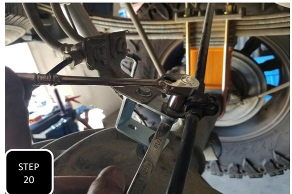
**Step 20** Attach the brake line bracket and E-brake cable guide to the top holes of the provided bracket using the provided 1/4" bolts, nuts, & washers.
