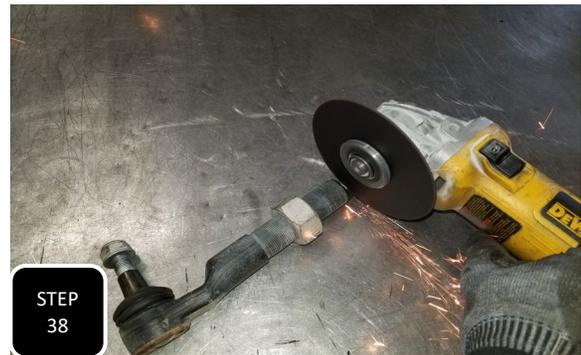
**Step 38** Loosen the clamp on the tie rod and remove the rod end. Using a suitable cutting device, cut off the half circle end piece after the threads and then thread the rod end back into the sleeve, leaving the rod end pointing upward now instead of downward like it was from the factory.
