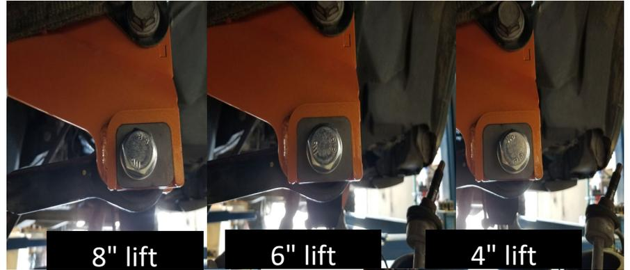
**Step 37** Slide the trac bar up into the new drop down bracket and loosely attach it using the provided M18 hardware and square plates with off-set hole. Install the plate so that the bolt is off-set to the passenger side of the truck. **NOTE: DO NOT FULLY TIGHTEN THIS BOLT UNTIL THE TRUCK IS ON THE GROUND AT RIDE HEIGHT.**
