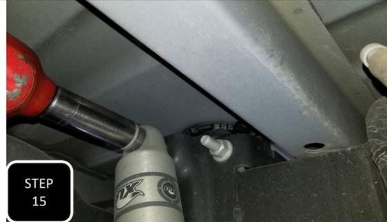
**Step 15** Jack up the rear of the truck and support under the frame with jack stands. Apply pressure to the rear diff with an adjustable jack and remove both rear shocks.
