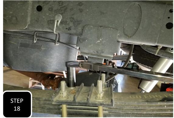
**Step 18** Install the provided U-bolts and loosely attach until both lift blocks have been installed. Next, torque the U-bolts to 100 ft/lbs.
