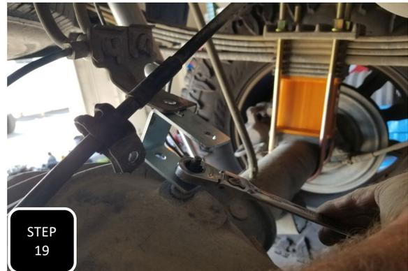
**Step 19** Unbolt the brake line bracket and E-brake loom clamp on top of the differential and attach the provided brake line bracket using the factory stud and nut.
