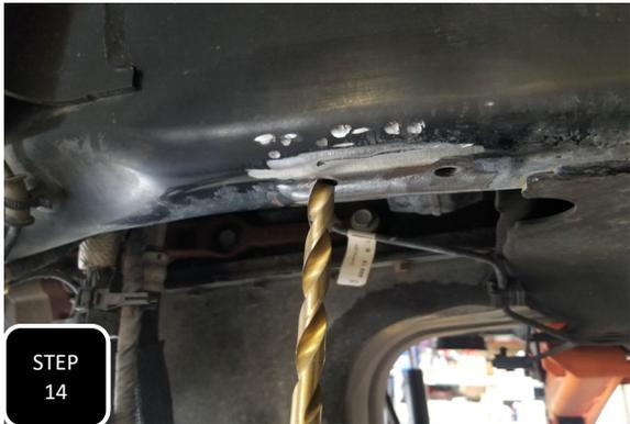
**Step 14** Drill out the holes in the frame using a 7/16" drill bit and then tap both holes using a 1/2-13 thread taper.
