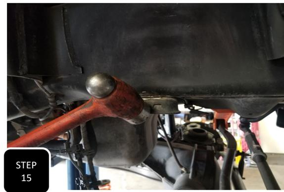
**Step 15** Using a suitable cutting device, cut the welds of the factory bump stop cup and then hit it with a hammer to break it loose. **NOTE: TRY NOT TO DAMAGE OR DISTORT THE CUP AS IT NEEDS TO BE RE-USED.**
