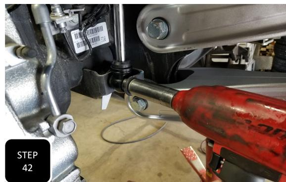
**Step 42** Repeat step 41 on the other side and then tighten the top and bottom of both shocks.
