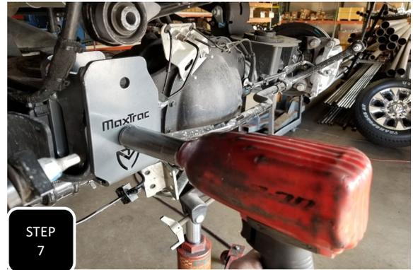
**Step 7** Loosely attach the trac bar bracket to the coil mount on the axle using the provided 3/8" hardware and then start the tightening process by tightening down the main trac bar bracket bolt to factory specs.
