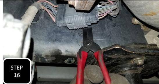
**Step 16** On the drivers side, unclip the wire guide from the inside of the frame and on the passenger side unclip the wire harness clip from the inside of the frame.
