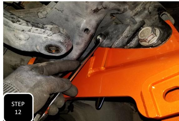
**Step 12** Loosely install the new trac bar bracket into the factory trac bar bracket using the factory bolt. Next, install the provided 7/16" bolt, nut and washer into the small tab mount further up the factory mount. **NOTE: DO NOT FULLY TIGHTEN EITHER BOLT AT THIS TIME.**
