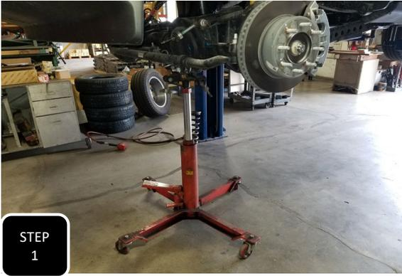
**Step 1** Jack up the front end of the vehicle and support under the frame rails with jack stands. Keep an adjustable jack under the axle for height adjustment.
