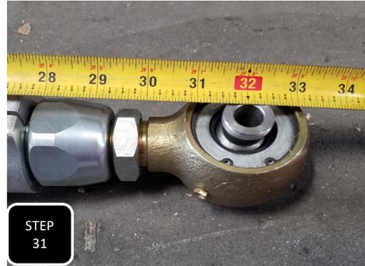
**Step 31** Adjust the upper links to 28.5" (the shorter link) and the lower links to 32" (the longer link). Now locate the links for the side that you are working on first. The driver's side links, when installed will have the Max Trac logo facing upright and the two pinch bolts facing outward when installed. **NOTE: THE ROD ENDS ARE NOT PRE-GREASED AND REQUIRE GREASE FOR PROPER FUNCTION.**
