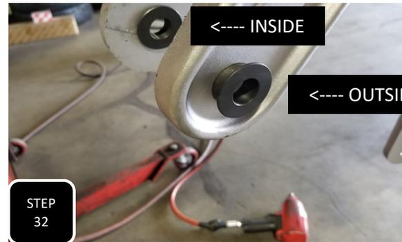
**Step 32** Loosely attach both links to the 4link bracket first using the provided 9/16" bolts and then install the provided machined, hat looking sleeves on the other end of the link with 1 hat inside the clevis and 1 hat on the outside.
