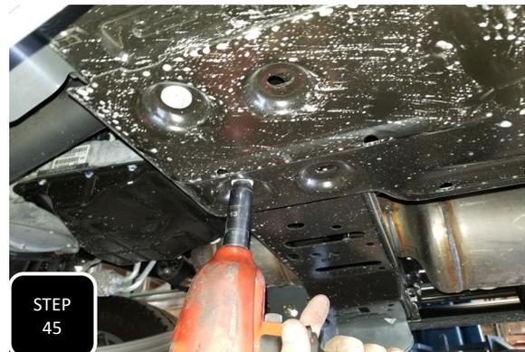
**Step 45** Re-attach the brake line brackets to the top of the axle and ensure that the brake lines are not tight when the suspension is at full droop. Next, re-install the skid plate under the transfer case and tighten.
