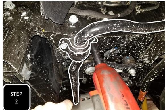
**Step 2** Unbolt the sway bar from both end links and the frame on both sides and remove.
