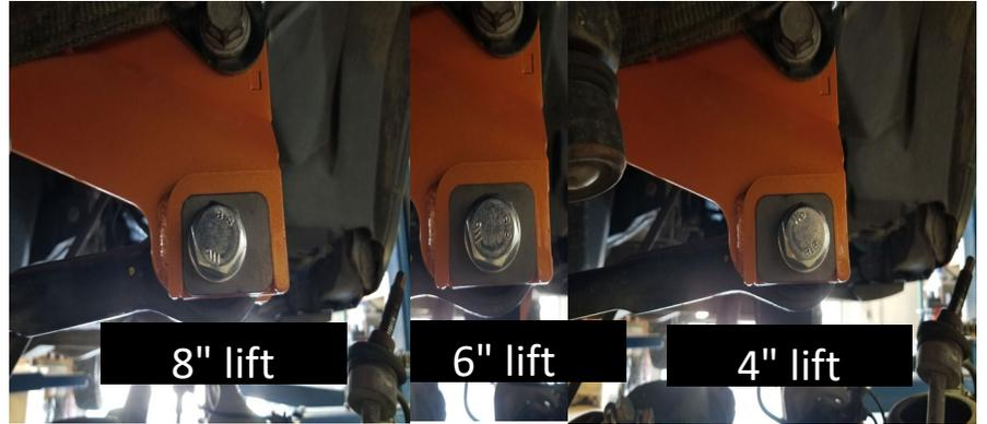
**Step 37** Slide the trac bar up into the new drop down bracket and loosely attach it using the provided M18 hardware and square plates. For the 4" lift, you will use the square plates with the off-center hole off-set to the driver's side. For the 6" lift, you will use the square plates with the centered hole. **NOTE: DO NOT FULLY TIGHTEN UNTIL THE TRUCK IS ON THE GROUND AT RIDE HEIGHT.**
