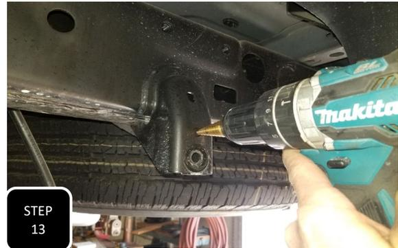
**Step 13** Loosely attach the sway bar drop down bracket to the factory bracket on the frame and mark the upper hole for drilling. Remove the bracket and drill a 7/16" hole at your mark. **NOTE: USING A STEP BIT WILL SPEED UP THE DRILLING.**
