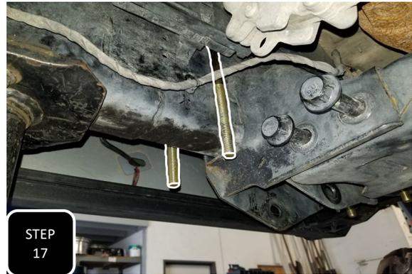
**Step 17** For the passenger side, slide the supplied U-bolt over the frame, just behind the cross member behind the factory radius arm bracket and allow it to hang vertically.
