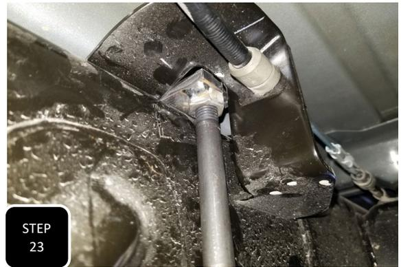
**Step 23** Loosely install the radius arm drop down bracket into the original mount using the factory bolt and then loosely attach the provided 1/2-13 x 9" bolts, washers, and lock washers to the nut plate on top of the frame. Push the bracket up tight to the frame and torque the factory bolt to factory specs and the 1/2" bolts to 90 ft/lbs.
