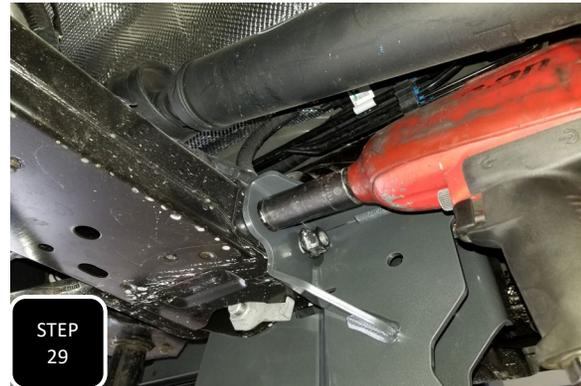
**Step 29** First snug up the U-bolt nuts, then the cross member bolts, and lastly the original radius arm bolt. Once all is snug and the bracket is up in place, go back and torque all bolts to factory specs. The U-bolt should get torqued to 100 ft/lbs.
