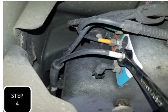
**Step 4** Locate the air ride valve block on the outside of the passenger side frame rail and crack open the two lines leading to the rear air bags to bleed the air out of them. Once the bags have been deflated, tighten up both fittings.
