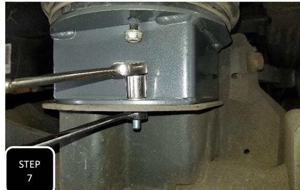
**Step 7** Tighten down the studs at the air bags using the factory nuts. Next, attach the spacers to the axle using the provided M8 bolts, nuts and washers then tighten.
