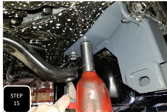
**Step 15** Install the new trac bar bracket using the original bolts along with the provided M14-2.0 nylock nuts. Make sure all the bolts are started in their threaded holes, then first, get all of the vertical bolts to a hand tight, then fully tighten the two horizontal bolts, and lastly tighten down the vertical bolts to factory spec.
