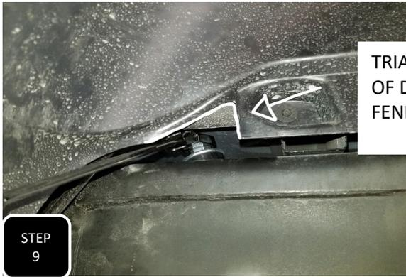
TRIANGULAR NOTCH CUT OUT OF DRIVER'S SIDE PLASTIC FENDER WELL FOR ACCESS TO
