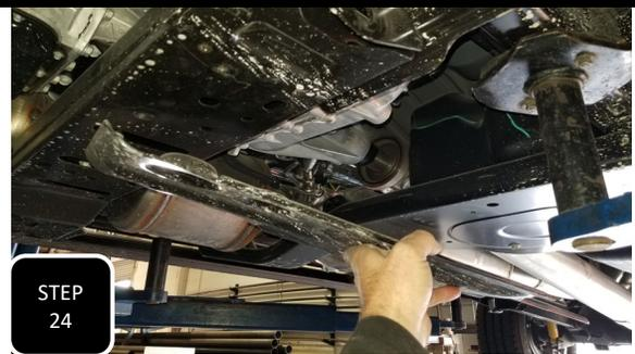
**Step 24** Unbolt and remove the skid plate under the transfer case and set aside to be re-installed later.
