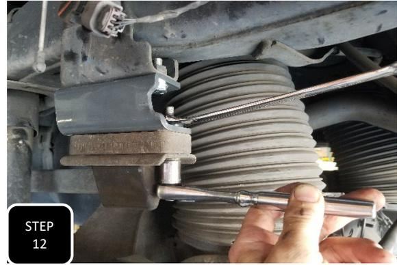
**Step 12** Unbolt the factory bump stops along with the 1" spacers. Next, install the bump stop extension brackets with the notched edge facing the back of the truck and the open end facing inward using the provided bolts and washers. Next, attach the factory bump stops along with the factory 1" spacer to the new bracket using the factory bolts and provided nuts/washers. Once everything is loosely attached, tighten it up.
