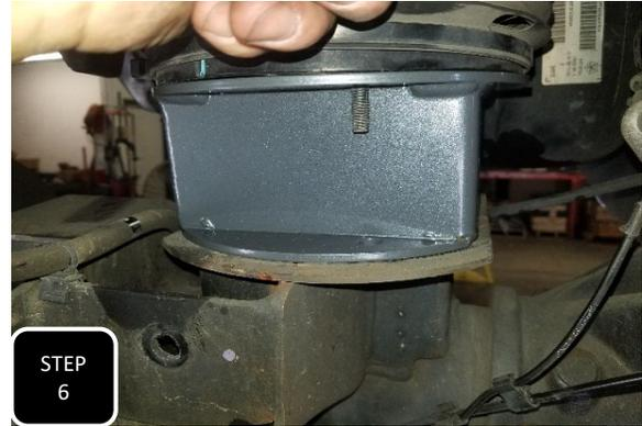
**Step 6** Remove the lower mounting nuts on both air bags, lower the axle and then install the air bag spacers under the air bags with the short side of the spacer facing the front of the truck. The round plate on the spacer will face up and attach to the air bag while the side of the spacer with the flat sides will bolt up to the axle.
