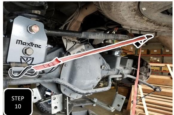
**Step 10** Use a ratchet strap to pull the axle over and align the trac bar with the hole in the new bracket then loosely attach with the provided square plates and M14 bolt.
