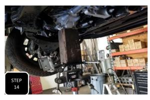
**Step 14** Place an adjustable jack under the front differential for support and height adjustment.
