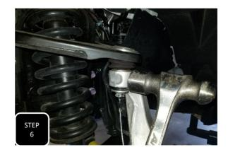
Step 6 Remove the retainer clip from the upper ball joint nut and then loosen, but do not remove the nut. Next, hit the side of the spindle, right at the upper ball joint, with a hammer to break the ball joint loose. The nut will catch the spindle then separate and allow the spindle to swing down. **NOTE: BE CAUTIOUS NOT TO DAMAGE THE BRAKE LINE OR ABS LINE.**
