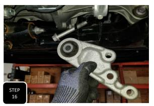
**Step 16** Loosen up all 4 bolts for the passenger side, front diff mount and remove the mount.
