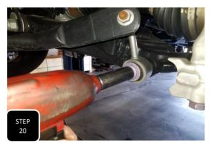
**Step 20** Lower the truck down to the ground and re-install the sway bar end links using the factory hardware. **NOTE: HAVING THE TRUCK ON THE GROUND AT RIDE HEIGHT MAKES INSTALLING THE SWAY BAR ENDS LINKS MUCH EASIER.**
