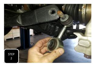
**Step 2** Unbolt the sway bar end link at both ends and remove the link. Next, move to the other side and remove that end link too.
