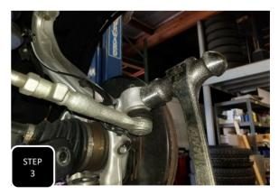
**Step 3** Remove the cotter pin at the tie rod and then remove the nut. Next, break the tie rod loose by hitting the side of the spindle, right at the tie rod, with a hammer. This will break the wedge fit and allow you to separate the tie rod.
