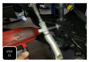
Step 21 With the truck now on the ground at ride height, torque the lower strut bolts to 80 ft/lbs.
