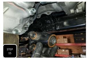
**Step 15** Loosen up all 3 bolts for the driver's side, front diff mount and remove the mount.
