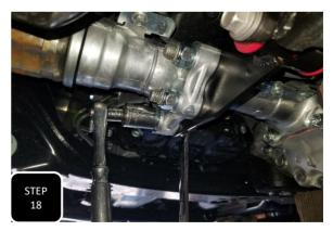
**Step 18** Loosely install the new pass side diff mount using the factory bolt/nut at the frame and the factory bolts along with the provided nuts/washers at the diff. **NOTE: THE BRACKET WILL ALIGN ON THE DRIVER'S SIDE OF THE MOUNT ON THE DIFF.**
