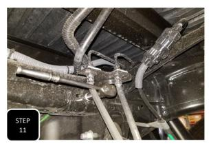
**Step 11** Re-attach the ABS line brackets and the brake line bracket using the factory bolts and tighten.
