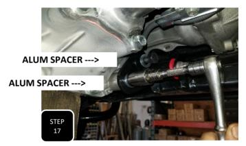
**Step 17** Lower the diff about 1 inch and then loosely install the new drive side diff mount using the provided M14 bolts and 1" aluminum spacers between the mount and diff. You will re-use the factory bolt and nut at the frame.
