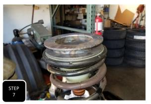
**Step 7** Install the spacer on top of the coil with the centering nipple inside of the bump stop housing.
