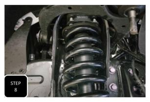
**Step 8** Place the spacer on top of the strut and tighten down using the factory nuts. The 4 bolt pattern is not symetrical and the spacer will align with the part # facing outward. Next, re-install the strut assembly. **NOTE: SINCE THE STRUT ASSEMBLY IS NOW TALLER, IT WILL BE MORE DIFFICULT TO INSTALL AND REQUIRE PUSHING THE LOWER CONTROL ARM DOWNWARD TO CLEAR THE LOWER MOUNTING BOX.**
