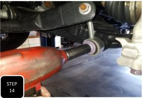
**Step 14** Lower the truck down to the ground and re-install the sway bar end links using the factory hardware. **NOTE: HAVING THE TRUCK ON THE GROUND AT RIDE HEIGHT MAKES INSTALLING THE SWAY BAR ENDS LINKS MUCH EASIER.**
