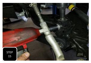
**Step 15** With the truck now on the ground at ride height, torque the lower strut bolts to 80 ft/lbs.
