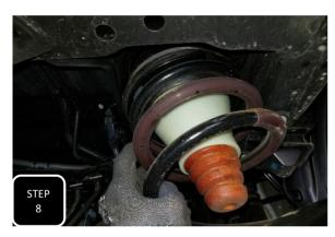
**Step 8** Re-install the springs back into the truck and make sure the bottom of the coil indexes properly on the coil seat.
