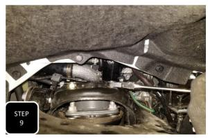
**Step 9** Loosely install the struts lower mounting bolt but do not tighten. Next, attach the top of the strut to the frame using the provided flange nuts and tighten. **NOTE: THE LOWER BOLT WILL GET TIGHTENED WHEN THE TRUCK IS BACK TOGETHER AND SITTING AT RIDE HEIGHT.**
