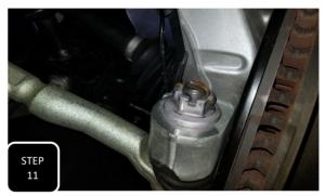
**Step 11** Re-attach the tie rod from the bottom-up, using the factory nut and torque to 60 ft/lbs. Next, re-install the factory cotter pin.
