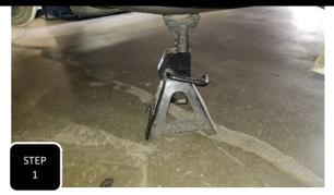
**Step 1** Jack up the rear of the truck and support under the frame rails with jack stands. Keep an adjustable jack under the differential for height adjustment.
