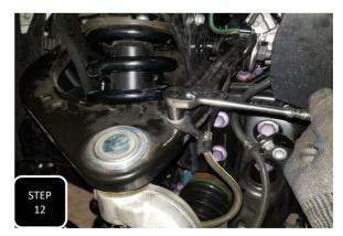
**Step 12** Re-attach both the brake line mounting bracket and the ABS line guide brackets using the factory bolts and tighten.
