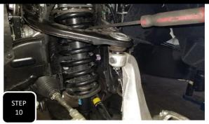
**Step 10** Place a floor jack under the lower control arm and jack up a few pumps to get the coil to compress. Next, pull down on the upper control arm and place a pry bar above it to aid in prying down on the UCA while lining up the spindle with the ball joint. Once aligned, attach the UBJ nut and tighten to 80 ft/lbs. **NOTE: IT IS POSSIBLE FOR THE AXLE TO POP OUT OF THE CV JOINT WHILE EXTENDED, SO MAKE SURE THE AXLE PROPERLY PLUNGES INTO THE CV BEFORE ATTACHING THE UCA.**
