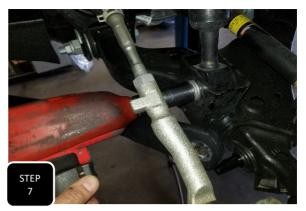
**Step 7** Remove the 4 nuts at the top of the strut and then the single bolt at the bottom of the strut. Next, push down on the lower control arm and remove the strut assembly.
