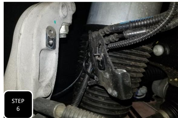
**Step 6** Air ride models will have a body position sensor attached to the upper ABS sensor bracket which gets removed just as step 5 shows. Unbolt this and the ABS sensor then move and hang safely out of the way.
