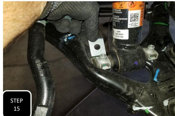
**Step 15** Unbolt the two bolts attaching the strut to the lower control arm and then insert the provided 1019AR-1 spacer plates between the strut's barpin and the control arm.
