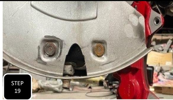
**Step 19** If your truck has a factory big brake kit then the factory dust shield will have an opening at the bottom and two studs sticking through the back side. The studs will need to be cut down flush on the back side of the dust shield or they will contact the face of the lowering spindle, pushing the dust shield outward, and causing the dust shield to rub against the rotor.
