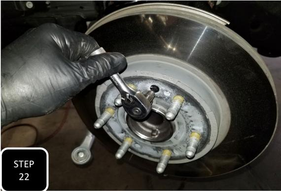
**Step 22** Attach the rotor by tightening the factory retainer bolt and then install the brake caliper using the factory bolts and tighten.
