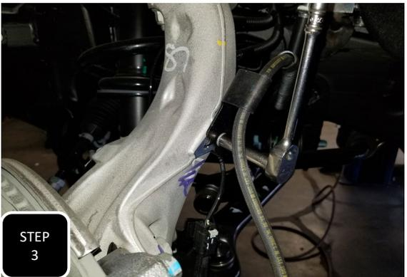
**Step 3** Unbolt the brake line guide bracket from the side of the neck of the spindle and separate.
