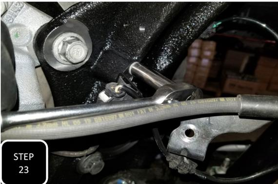
**Step 23** Attach the brake pad sensor wire to the neck of the spindle using the factory M6 bolt and then do the same with brake line bracket using the factory M6 bolt and tighten.
