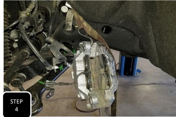
**Step 4** Unbolt both brake caliper mounting bolts and support the brake caliper up out of the way. **NOTE: NEVER ALLOW THE BRAKE CALIPER TO HANG BY THE BRAKE LINE.**
