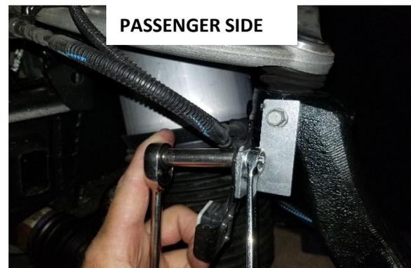
**Step 26** Attach the provided 1019AR-P bracket to the neck of the spindle using the factory M6 bolt and tighten. Next, attach the factory body position sensor to the bracket using the provided M6 bolt, nut & washers, then tighten.
