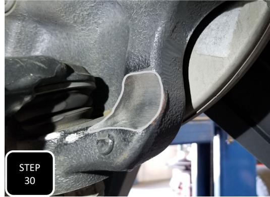
**Step 30** Using a 4.5" angle grinder with a flap disk or grind wheel, clearance this marked strike zone about 1/8" deep at the area of the contact point and smoothly transition your grind up and down.
