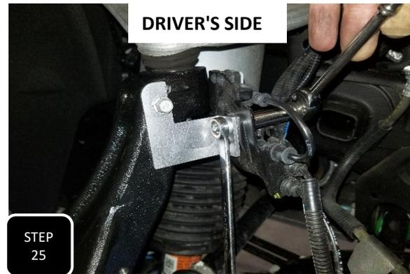
**Step 25** Models with air ride will attach the provided 1019AR-D bracket to the neck of the spindle using the factory M6 bolt and tighten. Next, attach the factory body position sensor to the bracket using the provided M6 bolt, nut & washers, then tighten.
