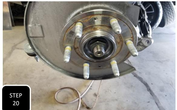
**Step 20** 4wd models will need to re-attach the axle to the wheel bearing using the factory nut and tighten to factory specs.
