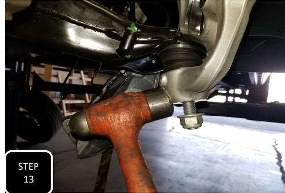
**Step 13** Loosen the nut attaching the lower ball joint to the spindle, but do not remove. Next, hit the side of the spindle, right at the ball joint, with a hammer, to break it loose and the nut will catch the spindle. Then remove the spindle. **NOTE: NEVER HIT THE BALL JOINT ON THE THREADS.**
