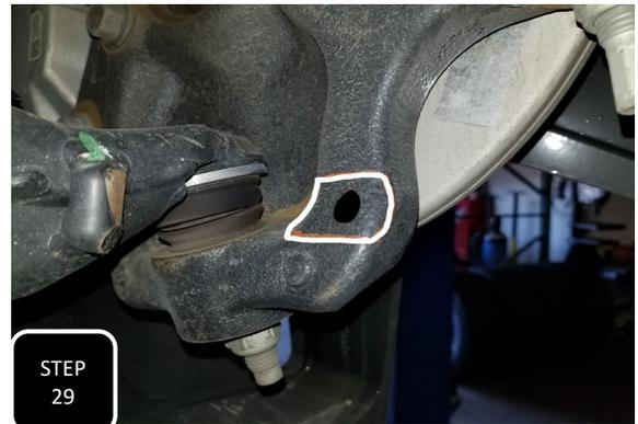
**Step 29** Start first by driving the truck and cycling the steering a few times to full turn so that a contact mark is left in the strike zone. Next, put the truck up in the air and mark about a 1.5" vertical area around the impact mark. This will be the area to clearance.
