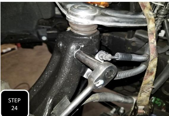
**Step 24** Attach the last guide bracket for the ABS and brake pad wires to the back side of the upper ball joint boss on the spindle using the factory M6 bolt and tighten.
