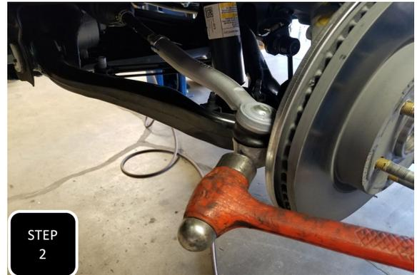
**Step 2** Unbolt the nut attaching the outer tie rod to the spindle and break loose by hitting the side of the spindle with a hammer, right at the tie rod. **NOTE: NEVER HIT THE TIE ROD ON THE THREADS.**
