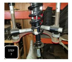
Step 7 First take note of the relationship between the strut top and lower clevis. This reference will help during reassembly. Compress the coil using a strut compressor and remove the nut at the center of the strut top. NOTE: IF THE THREADS HAVE ANY RUST, SPRAY WITH WD-40 AND LET SOAK FOR A FEW MINUTES.
