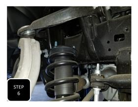
**Step 6** Un-bolt the strut at the top by removing all 3 nuts and remove the strut.
