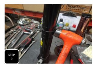
Step 9 Slide the snap ring retainer over the snap ring. If the retainer does not slide over the ring, then tap the ring with a hammer to fully seat it and then install the retainer. NOTE: THE RETAINER MUST GO COMPLETELY OVER THE SNAP RING AND FULLY SEAT OR YOUR SUSPENSION COULD FAIL.
