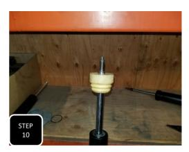
Step 10 Install the provided lower coil seat and then transfer over the factory bump stop.
