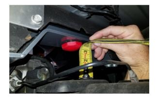
AT A 6" DROP, YOU WILL HAVE ABOUT A 3" GAP BETWEEN THE AXLE AND BUMP STOP AT RIDE HEIGHT.
