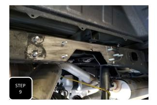
**Step 9** Using a power drill and 9/16" drill bit, drill out all 12 of your marked holes on each frame rail and then test fit the inner bolt plate. Enlarge or correct your holes until all 8 bolts slide through the holes and allow the inner plate to sit flat against the inside of the frame.
