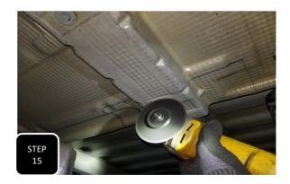
**Step 15** This marked section of heat shield will now need to be cut out using a suitable cutting device such as a cut off wheel.
