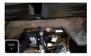
**Step 6** Using a suitable cutting devise such as a plasma cutter or a cut off wheel, cut out the notched section and clean up the edges with a sander. Test fit the C-notch and clearance as necessary until it fits flush to the frame.
