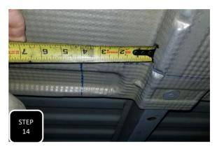
**Step 14** Locate the heat shield on the pass side of the truck above the rear differential. Draw a straight line 4 inches from the edge and as long as about 5 inches in front and behind the bed rib. Next, measure and draw a line 4 inches from the bed rib towards the front of the truck and 3.5 inches from the rib towards the rear of the truck.
