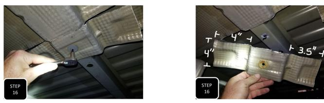
Step 16 Once all the way cut out, remove the mounting bolt in the cut area and remove the cut section of heat shield.
