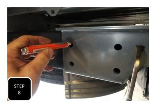
**Step 8** Clamp the C-notch to the frame and either mark the holes for drilling or more preferably, use a transfer punch to mark the 8 side holes and 4 holes underneath the frame.
