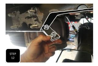
**Step 12** Slide the -3 and -4 nut plates into the bottom of the frame. The plate with the nuts that are closer together will go into the cut out towards the front of the truck and the other towards the rear of the truck.
