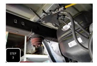
**Step 3** Unbolt the brake line guide bracket located on the inside of the driver's side frame and hook it out of the way with a bungy cord or strap.
