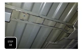
**Step 18** Using a suitable cutting device such as a cut off wheel, completely cut out and remove this section of bed rib above the rear differential.
