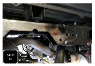
**Step 10** Smooth out any chunky spots of the factory under coat and then spray paint all raw surfaces of the factory frame for rust prevention.
