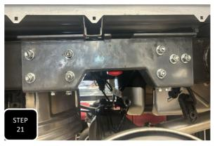
**Step 21** We have not been able to officially fit our C-notch to a long bed, but have had customer's whom have taken it upon themselves to do so. From what we know, the reference bed rib is in a different location on the long beds so an additional notch will need to be cut out of the supplied frame support to properly align the notch with the axle.
