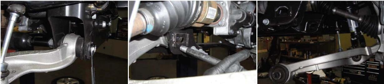
9. Remove upper strut mounting bolts, then remove strut assembly from vehicle.
