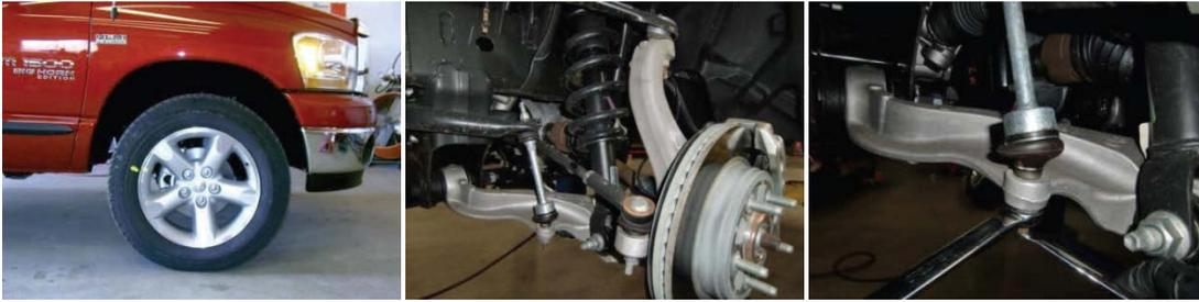
3. Remove lower strut mounting nut
