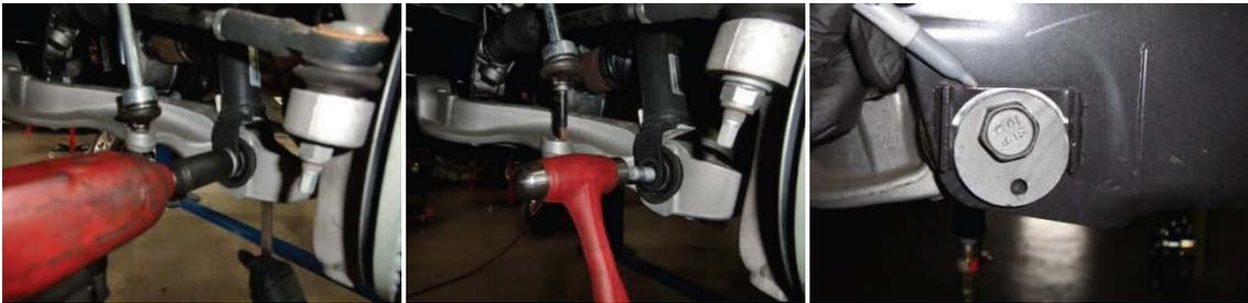
6. Loosen alignment cams and bolts.
