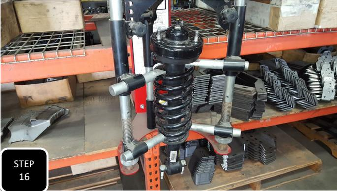
**Step 16** Because the strut spacer has a rotated bolt pattern, you will now need to compress the coil and rotate the bottom of the shock 180 degrees so that the angled bar pin is once again angled inward.
