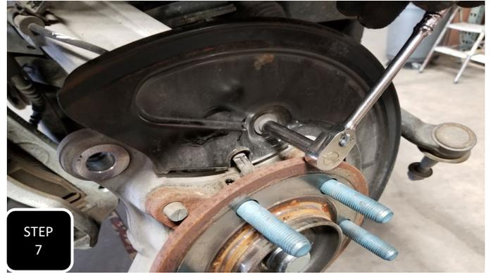
**Step 7** Unbolt the ABS sensor and position it out of the way. The top bolt of the dust shield will need to be removed for the ABS wire to clear and the sensor to be separated from the spindle.
