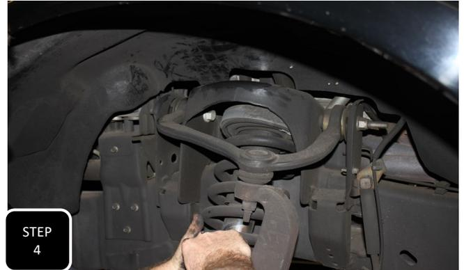
**Step 4** For 2004-2013 trucks, unbolt the 3 nuts at the top of the strut and the one bolt at the bottom of the strut then remove the strut. **Skip to step 12 for strut spacer install.**
