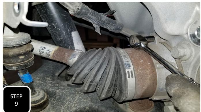
**Step 9** For 4wd models, you will also need to remove the 3 hub actuator bolts on the back side of the spindle.
