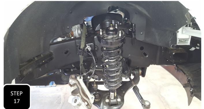
**Step 17** Push down on the lower control arm with your knee or a pry bar while also lifting up on the upper control arm so that the studs on the top of the strut clear the tower. **NOTE: THIS WILL BE TOUGHER THAN THE REMOVAL BECAUSE THE STRUT IS NOW LONGER.**
