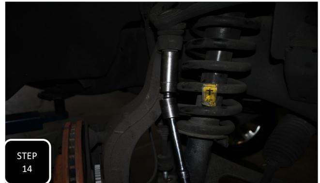
**Step 14** Support the spindle so that the brake line does not get stretched out while installing the lower strut bolt. Next, place a floor jack under the lower control arm and jack it up to compress the coil so that you can re-attach the upper control arm to the spindle and tighten.
