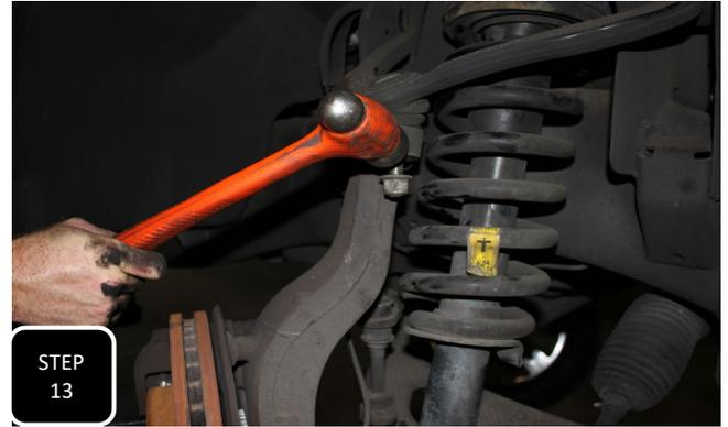
**Step 13** For 2004-2013 models you can loosely attach the top of the strut to the frame, then you will need to loosen the upper ball joint nut and then brake the ball joint loose by hitting the side of the spindle with a hammer. **NOTE: NEVER HIT THE BALL JOINT ON THE THREADS.**
