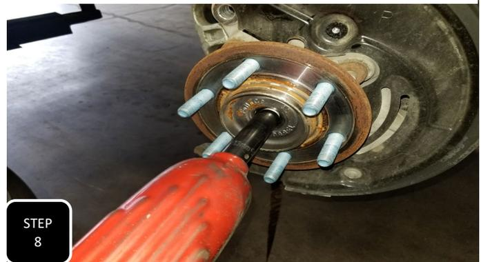
**Step 8** For 4wd models, you will need to remove the dust cap at the middle of the wheel bearing and then remove the axle retainer nut.
