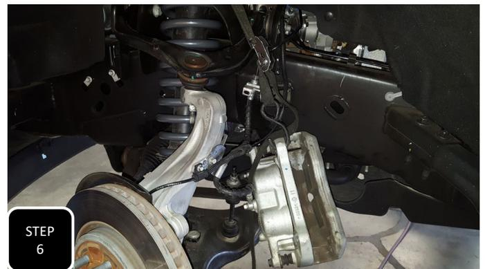
**Step 6** Unbolt the brake caliper from the spindle and support it out of the way. **NOTE: NEVER ALLOW THE CALIPER TO HANG BY THE BRAKE LINE.**
