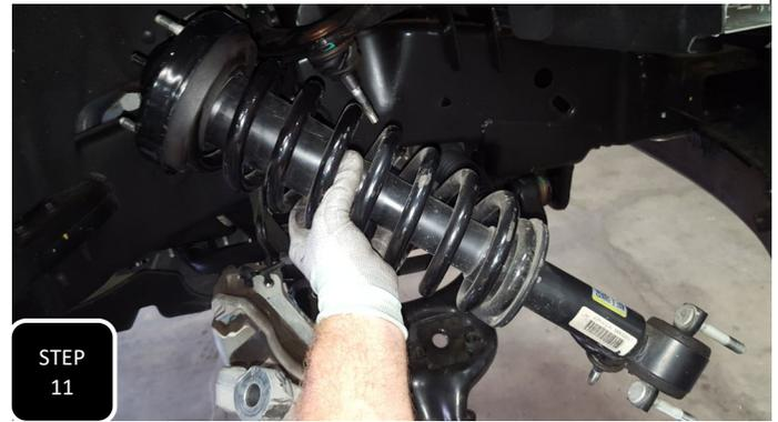
**Step 11** Push down on the lower control arm with your knee or a pry bar while also lifting up on the upper control arm so that the studs on the top of the strut clear the tower and you can remove the strut.
