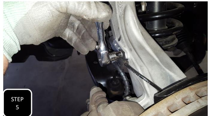
**Step 5** For newer models the whole spindle will need to come off to safely install the spacers so start by unbolting both the Brake line and ABS line from the neck of the spindle and separate.
