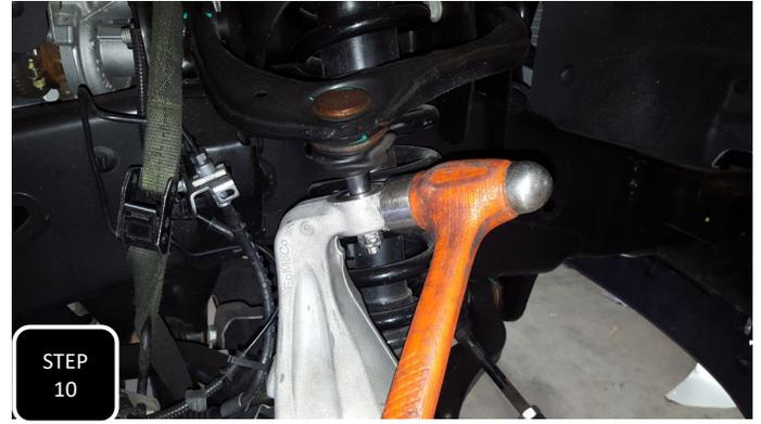
**Step 10** All models, unbolt both the upper and lower ball joints, but do not remove the nuts. Hit the side of the spindle, right at each ball joint, with a hammer to break them loose. The nuts will catch the spindle. Then remove the nuts and the spindle.
