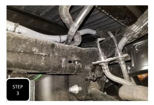
**Step 3** Unbolt the mounting bracket for the brake lines at the frame and separate. **NOTE: THIS WILL ALLOW FOR MORE SLACK IN THE LINES DURING THE INSTALL.**
