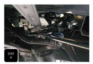
**Step 9** Lower the truck back to the ground and re-attach the shocks. **NOTE: THE REAR COILS ARE VERY TOUGH TO COMPRESS AND WILL LIFT THE TRUCK OFF OF THE CAR LIFT. LOWERING THE TRUCK TO THE GROUND ALLOWS THE WEIGHT OF THE TRUCK TO COMPRESS THE SPRINGS.**
