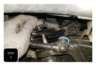
**Step 2** Apply some pressure to the differential with the jack and then unbolt both rear shocks at the frame and remove the upper bushing.
