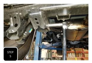
**Step 5** Loosen all 4 control arm mounting bolts, where the control arms bolt up to the brackets on the axle housing. NOTE: THIS WILL ALLOW THE AXLE TO DROP DOWN LOWER, MAKING ROOM FOR THE NEW SPACER ON TOP OF THE COIL SPRING.
