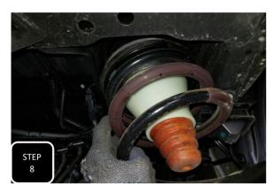
**Step 8** Re-install the springs back into the truck and make sure the bottom of the coil indexes properly with the coil seat on the axle.
