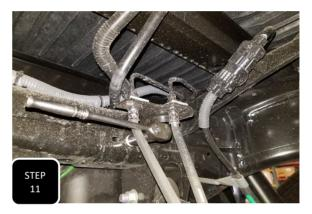
**Step 11** Re-attach the ABS line brackets and the brake line bracket using the factory bolts and tighten.
