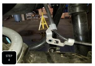
**Step 4** Unbolt both ABS line guide brackets at the axle and separate. **NOTE: THIS WILL ALLOW FOR MORE SLACK IN THE LINES DURING THE INSTALL.**
