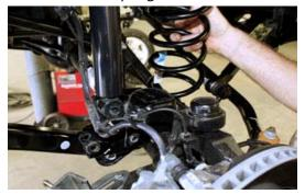
2. Remove bolt that holds brake lines to the frame, both sides.
