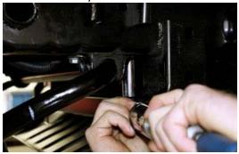
7. Install new Maxtrac Spacer, with bolt, nut, and washer. Install Rubber isolator.
