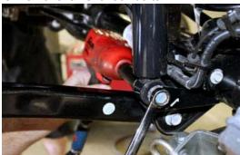
5. Remove Coil Springs and isolator.
