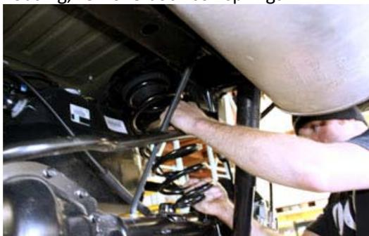
18. Set welded nut plate in thru top of the frame in coil bucket. Install rear spacer w/ the new 1/2" bolt and lock washer.
