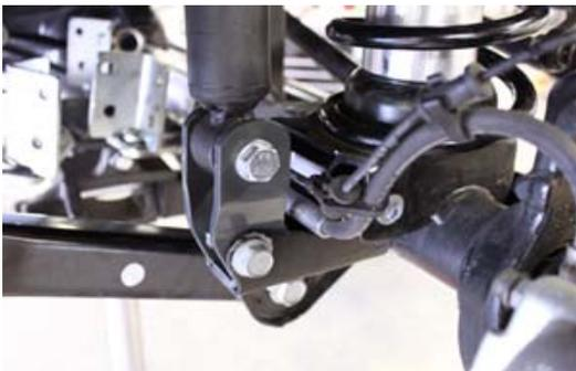
8. Locate bump stop spacer, center it on the front axle bump stop plate. Center punch, drill 11/32" hole & tap with self tapping bolt supplied in kit. Remove spacer & set in coil spring for installation.
