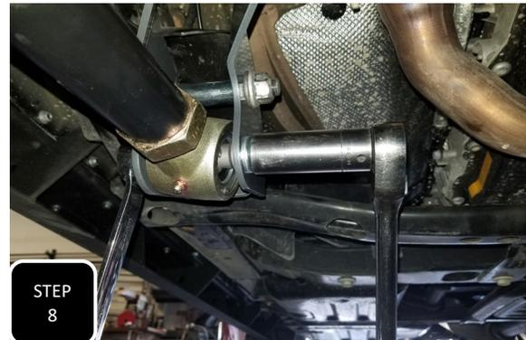
**Step 8** Tighten down both control arm bolts. The upper arm bolt should be torqued to 60 ft/lbs where as the lower control arm bolt should be torqued to 160 ft/lbs.
