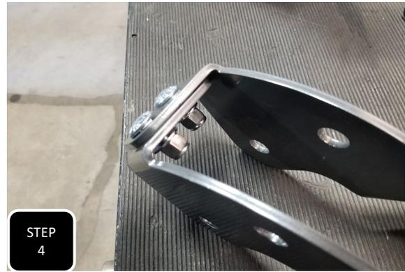
**Step 4** Loosely assemble the brackets for each side using the provided 3/8" carriage bolts. The square holed brackets will assemble on the outside forcing the carriage bolts to point toward the inside of the bracket.
