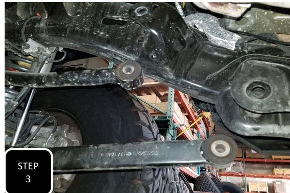
**Step 3** Remove the bolt attaching the lower control arm to the frame on the same side as the upper control arm you just unbolted and allow the axle to roll forward enough for the arms to come out of the mounting pockets.
