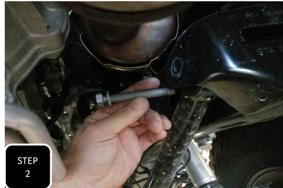
**Step 2** Working on one side at a time, remove the bolt attaching the upper control arm to the frame and keep the bolt for the install of the new bracket.
