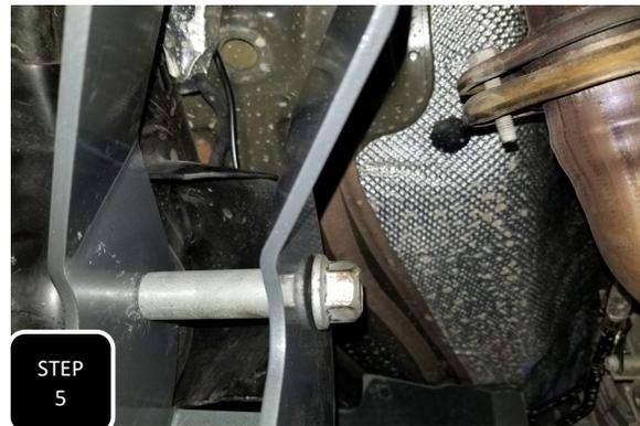
**Step 5** Locate the correct bracket assembly for the side of the truck that you are working on and loosely install it using the small tube/stock bolt up top and the large tube/stock bolt at the bottom. **NOTE: BOTH EARS OF THE NEW BRACKET WILL MOUNT INSIDE THE ORIGINAL POCKET OF THE UPPER MOUNT, BUT ONLY ONE IN AND ONE OUT FOR THE LOWER POCKET.**
