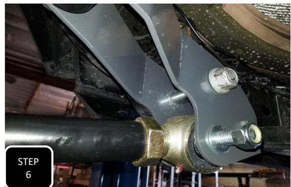
**Step 6** Loosely attach the upper and lower control arms to the new bracket using the provided hardware. The upper arm will go in the top hole if you have a 2.5" lift, the middle hole if you have a 3.5" lift, or the bottom hole if you have a 4.5" lift.
