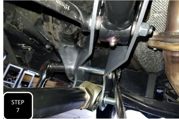
**Step 7** Once every thing is loosely installed, tighten down the bolts that attach the brackets to the frame and torque to factory specs.
