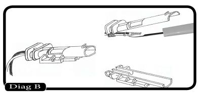
**STEP 7:** Insert the tool deep into the plug and depress the spring on the wire end. While the spring clip is depressed, lightly pull on the back side of the wire until the wire pulls out.
