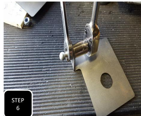
**Step 6** Attach the the mounting ball to the new plate using the provided M6-1.0 nylock nut and tighten. **NOTE: REFER TO NEXT PAGE FOR AMOUNT OF DROP AND MOUNTING HOLE TO USE.**
