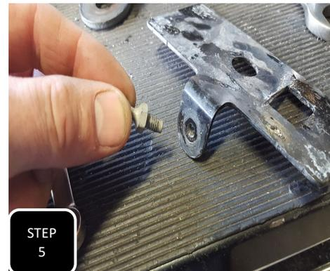
**Step 5** The rear sensor plate will need to be installed as soon as the axle is flipped and the U-bolts are ready to be installed. Loosen then remove the mounting ball from the original plate.
