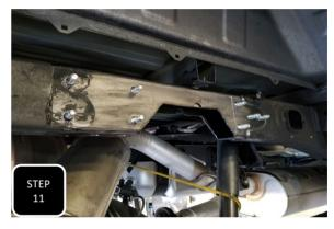
**Step 11** Slide the inner support plate, with the 8 bolts welded to it, into the frame and poke the bolts through the holes that you just drilled. **NOTE: THE PLATES ARE SIDE SPECIFIC AND THE TRIANGULATED END NEEDS TO FACE THE FRONT OF THE TRUCK.**
