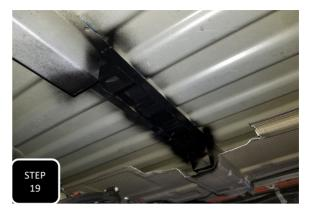
**Step 19** Clean up any and all sharp edges and then spray paint to prevent rust.
