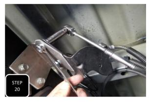
**Step 20** Install the bracket line relocation bracket to the frame using the factory bolts and then attach the factory bracket to the new bracket using the provided 8mm bolts, nuts, and washers.
