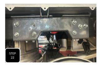
**Step 22** With the vehicle at ride height, position the frame support up, against the frame and align the bump stop with the center of the axle. Next, mark where the bed rib needs to be cut out and using a suitable cutting device, notch out the frame support. Modify the provided template to match your new notch and then proceed with the rest of the install.
