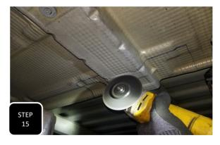
**Step 15** This marked section of heat shield will now need to be cut out using a suitable cutting device such as a cut off wheel.
