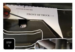
**Step 5** Bent with the writing outward, the template will line up with the outside of the passenger side of the frame and the inside of the driver's side frame. Using a small screw driver, scratch the under coat off along the inside of the notch cut out. Next, fold the template the other way and do the same with the outside of the driver's side frame and the inside of the passenger side frame.
