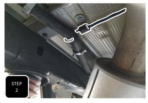
**Step 2** Separate the plastic guide clip attaching the wire harness on the inside of the passenger side of the frame, from the frame and hook it out of the way with a bungy cord or strap.
