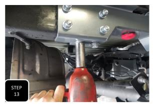
**Step 13** First install the bump stops onto both frame supports. Next, slide the frame support onto the frame and loosely start all of the mounting hardware. Once all of the hardware is started, then tighten down the side nuts first and the bottom bolts last.
