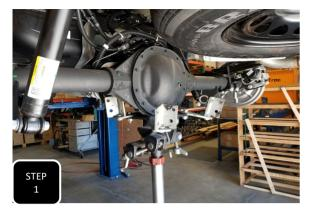
**Step 1** Jack up the rear of the truck and support under the frame, in front of the axle, with jack stands.
