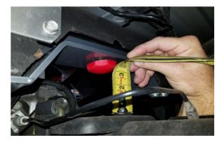
AT A 6" DROP, YOU WILL HAVE ABOUT A 3" GAP BETWEEN THE AXLE AND BUMP STOP AT RIDE HEIGHT.
