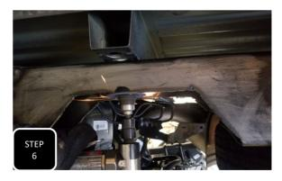
**Step 6** Using a suitable cutting devise such as a plasma cutter or a cut off wheel, cut out the notched section and clean up the edges with a sander. Test fit the C-notch and clearance as necessary until it fits flush to the frame.
