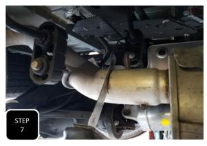
**Step 7** The factory exhaust will need to be cut off just before the axle. Start by spraying WD40 on all of the rubber bushings attaching the exhaust to the frame and then get the bushings started over the head of the hanger. Next, using a recipricating saw, completely cut throught the exhaust tubing just before the axle and then remove and disgard.
