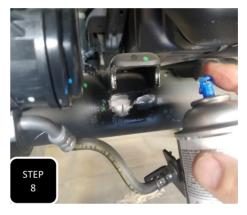
**Step 8** Clean up any sharp edges and spray paint the area for rust prevention.
