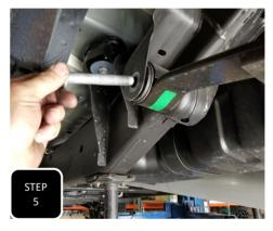
**Step 5** Loosen then remove the bolt attaching the spring to the frame at the front of the leaf spring and then remove the leaf spring.
