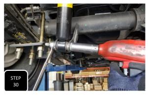
**Step 30** Install the new shorter shocks with the shaft of the shock attached at the frame and the body of the shock attached at the axle. **NOTE: IF YOU PURCHASED SHOCK EXTENDERS, NOW WOULD BE THE TIME TO INSTALL THEM ALONG WITH THE FACTORY SHOCKS. USE THE EXTENDER INSTRUCTIONS FOR INSTALL.**
