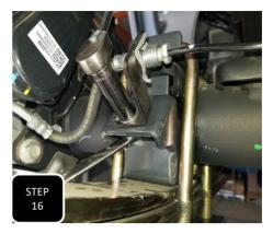
**Step 16** Locate the brake line mounting bracket still attached to the brake line and bend the guide tab to a flat position. Next, attach this bracket to the mounting bracket on the back side of the axle relocator using the provided M8 bolt, nut, and washer.
