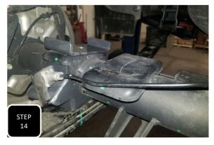
**Step 14** For 2020-2023 models, place the supplied 2 degree shim on the center pin with the thick end facing the rear of the truck. For 2024+ models, install the shim with the thick side facing the front of the truck. Next, place the axle relocator on top of the shim with the brake line mounting bracket facing rearward. Slightly loosen the U-bolts on the other side and then lower the axle into the relocator.
