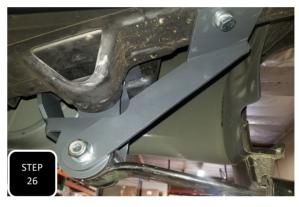
**Step 26** Insert the pass side, zinc plated nut plate into the hole in the outside of the frame, just back from the front leaf spring mount. **NOTE: THE NUT WILL LINE UP WITH THE SLOTTED HOLE IN THE BOTTOM OF THE FRAME.** Again, do not fully tighten the leaf spring bolt until the truck is on the ground at ride height.
