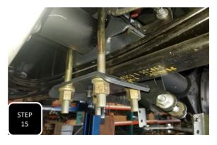
**Step 15** Place the U-bolt retainer plate on top of the original spring plate and run the new U-bolts downward though the provided spring perch under the leaf pack and tighten. **NOTE: THE U-BOLTS WILL INSTALL JUST LIKE THE FACTORY ONES DID. DO NOT TORQUE THE U-BOLTS DOWN AT THIS TIME.**
