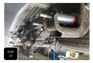
**Step 13** Jack up the axle and loosely re-install the leaf spring underneath the axle using the provided 16mm bolt at the front of the spring and the factory bolt at the shackle.
