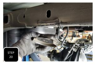
**Step 20** Once both cuts are made, it may help to hit the cut piece with a hammer until it breaks loose and then remove it from the frame. Next, clean up any sharp edges and spray paint for rust prevention.
