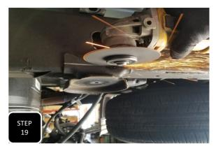
**Step 19** Unbolt the brake line guide bracket on the inside of the driver's side frame rail and support out of the way. Next, you will need to cut off the welded on bump stop plate using a suitable cutting device. Make a clean cut on each side of the frame rail.
