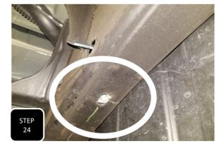
**Step 24** Insert the driver's side, zinc plated nut plate into the hole in the outside of the frame, just back from the front leaf spring mount. **NOTE: THE NUT WILL LINE UP WITH THE SLOTTED HOLE IN THE BOTTOM OF THE FRAME.**
