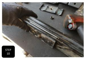
**Step 10** Slide the center pin through the factory 2 degree shim and install the pin down through the top of the leaf spring with the thick end of the shim facing the front of the truck. Then tighten the center pin. **NOTE: ONLY 2019 MODELS HAVE THIS 2 DEGREE SHIM.**
