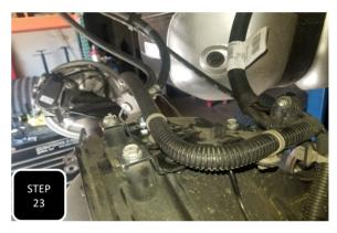
**Step 23** Locate the three "Z" shaped brake line brackets and loosely attach them to the factory bracket first using the provided hardware, and then to the diff using the factory hardware. The provided brackets are designed to push the factory bracket down and forward for more clearance between the diff and the bed.
