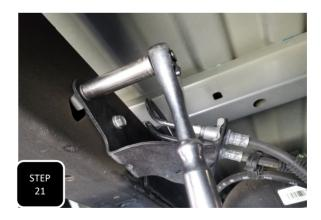
**Step 21** Once spray painted, re-install the brake line bracket using the factory bolts and tighten.
