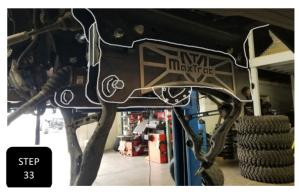
**Step 33** Loosely install both lower control arms using the factory cam bolts. **NOTE: DO NOT FULLY TIGHTEN THESE BOLTS AT THIS TIME.**
