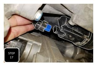
**Step 17** Locate the electrical plug on the front diff housing, slide the "red" safety clip out of the way, and then separate the plug.
