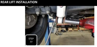
**Step 77** Support the rear axle with an adjustable jack and then unbolt both rear shocks at both ends and remove.
