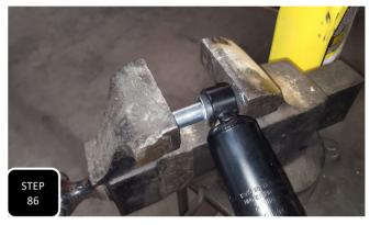
**Step 86** Locate your new longer rear shocks and shock hardware. Next, lube up the bushing on both ends of the shocks and using a bench vise, press the new shock sleeves in. **NOTE: IT HELPS THE PRESSING PROCESS TO PIVOT THE SHOCK UP AND DOWN WHILE CLOSING THE VISE.**
