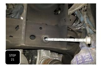
**Step 21** Next, remove the driver's side mounting bolt which can be accessed from the out side of the frame, in the middle of the strut tower.
