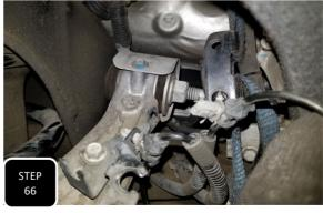
**Step 66** Separate the ABS sensor wire from both mounting points on the bracket at the upper control arm and then reroute the wire underneath the upper control arm instead of above it as it was from the factory.
