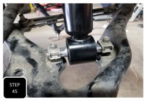
**Step 45** Use a flat head screw driver to pop the threaded clips off of the bar pin on the stock strut and then pop the clips onto the bar pin of the new strut.
