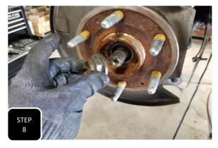
**Step 8** Loosen and remove the axle retainer nut. The axle should move freely in hub, if it does not, you will need to use an air hammer to break the corrosive bond and get it moving. **NOTE: IT IS NOT RECOMMENDED TO HIT THE AXLE WITH A HAMMER AS IT COULD DAMAGE THE THREADS.**
