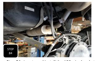
**Step 84** Locate and install the ABS wire bracket for the top of the differential. Attach it to the diff using the factory hardware and then attach the ABS line block to the bracket using the provided 1/4" hardware.
