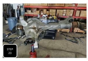
**Step 23** Slowely lower the differential making sure that there isn't anything else attached to it. Once the differential is clear, push it to a safe spot, out of your way, so that it does not get damaged.
