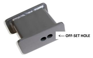
**Step 81** Install the new lift block and longer U-bolts. The lift block is angled and the short side must face the front of the truck. **NOTE: THE MAX TRAC LIFT BLOCK HAS TWO CENTER PIN HOLES. INSTALL THE CENTER PIN IN THE OFF-SET HOLE, WHICH WILL PUSH THE AXLE 1 INCH FORWARD AND MINIMIZE DRIVELINE PLUNGE.**
