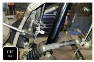
**Step 63** Attach the first brake pad sensor wire to the spindle using the factory M6 bolt. Next, attach the brake line guide bracket to the side of the spindle using the factory M6 bolt.
