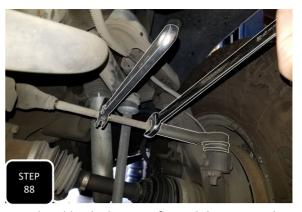
**Step 88** Install the new wheels and tires, then move the truck forward and back about 10 feet while moving the steering back and forth to settle the suspension. Next, adjust the vehicles tow alignment close to straight so that the vehicle is safe to drive to the alignment shop.
