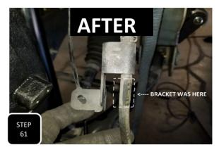
**Step 61** Locate the brake line mounting bracket in the middle of the brake line and slide it up the line about the same length as the height of the bracket.
