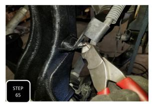
**Step 65** Attach the brake pad sensor wire to the brake line using two of the provided zip ties and then clip of the excess of unused zip tie.
