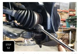
**Step 52** Install the hub assembly into the new steering knuckle using the factory bolts and torque to 120 ft/lbs.
