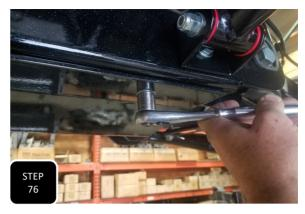
**Step 76** Attach the skid plate to the bottom of both subframes using the supplied M12 socket head screws on the front crossmember and the supplied 7/16" hardware at the rearward subframe then tighten. All bolts can get torqued to 45 ft/lbs.
