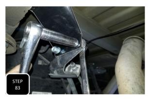
**Step 83** Locate the brake line bracket and install it between the frame and the factory brake line bracket on the inside of the driver's side frame rail. Attach it to the frame using the factory bolts and attach the factory brake bracket to this bracket using the provided M8 hardware. **NOTE: THE BRAKE LINE BRACKET IS THE LARGER "Z" SHAPED BRACKET.**
