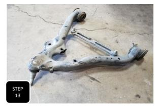
**Step 13** Unbolt both bolts attaching the lower control arm to the frame and remove the lower control arm.
