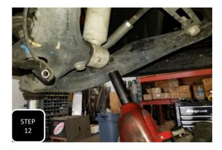
**Step 12** Unbolt the 3 nuts at the top of the strut and the 2 bolts at the bottom of the strut and then remove the strut.
