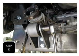
**Step 32** Loosely install the rear diff mounting ears using the provided 7/16" hardware to attach the mounts to the back side of the subframe and the provided M14-2.0 x 100 bolt at the diff bushing. First tighten the bolts attaching the mounting ears to the subframe and then tighten the diff bushing bolt. **NOTE: THE MOUNTING EAR WITH THE NOTCH CUT OUT OF IT GOES ON THE DRIVER'S SIDE OF THE DIFF BUSHING.**
