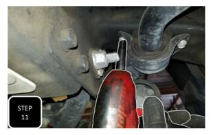
**Step 11** Unbolt the sway bar end links from each lower control arm and then unbolt all 4 frame mounting bolts and remove the entire sway bar.
