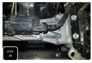
**Step 38** There is a wire guide clip for the front diff electrical plug located on the frame near where the steering shaft meets the steering rack. This clip needs to be separated from the frame to allow for extra slack in the line. Next, Plug the pig tail into the diff and engauge the red safety clip.
