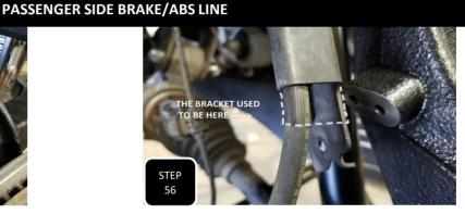
**Step 56** Attach the brake line guide bracket to the side of the spindle using the factory M6 bolt and tighten. Next, pull the brake line down through the mounting bracket to gain some slack between the brake caliper and mounting bracket.
