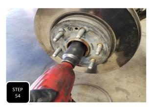
**Step 54** Install the axle nut and torque to factory specs.
