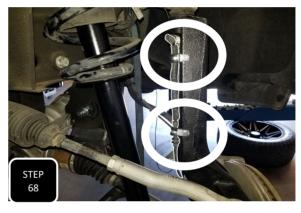
**Step 68** Separate the intermediate ABS line bracket from the rubber grommet on the line and then attach the ABS line to the front of the neck of the steering knuckle using the provided 3/8" loom clamps and M6 hardware.
