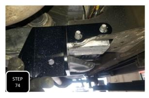
**Step 74** Locate the crossmember under the transfer case and remove the nuts from both mounting bolts on both sides. Next, Loosely install the supplied kicker bar brackets on the front side of the crossmember, push them upward so that the bottom of the backets contacts the bottom of the crossmember and then tighten.
