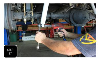
Step 87 Install the new longer shocks using the factory hardware and tighten. NOTE: MAX TRAC SHOCKS MUST BE MOUNTED WITH THE BODY AT THE AXLE AND THE SHAFT AT THE FRAME OR THEY WILL NOT WORK PROPERLY. FOX SHOCKS WILL MOUNT THE OPPOSITE, WITH THE BODY ON THE FRAME AND SHAFT AT THE AXLE.
