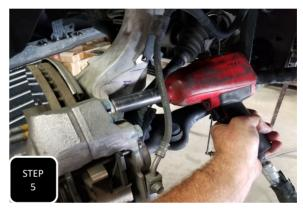
**Step 5** Unbolt the brake line guide bracket and then unbolt the brake caliper .
