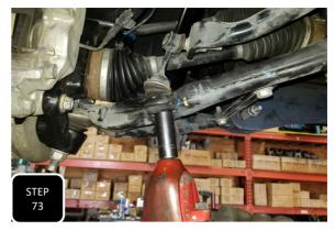
**Step 73** The sway bar will need to be flipped from its original position so that the middle of the bar swoops upward. Loosely attach the sway bar to the drop down brackets using the provided M10 hardware and attach the sway bar end links into the lower control arms using the factory nuts. Once everything is aligned, then fully tighten all connecting points.
