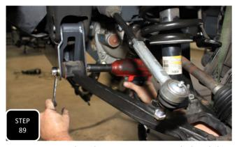
**Step 89** Now that the suspension is settled and the vehicle is sitting at ride height, go back and tighten all of the bolts that were left loose. **NOTE: TIGHTENING THE CONTROL ARM BUSHINGS WHILE THE TRUCK IS AT RIDE HEIGHT WILL PROLONG THE LIFE OF THE BUSHINGS.**
