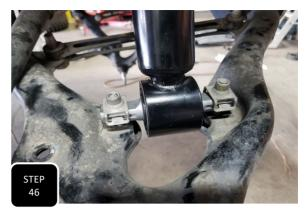
**Step 46** Loosely install the new strut assembly into the strut tower using the factory nuts. Next, swing up the lower control arm and loosely attach it to the bottom of the strut using the factory bolts.
