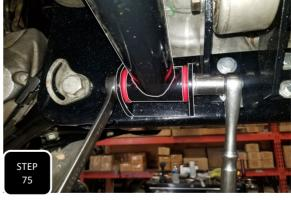
**Step 75** Locate the smaller, clevis looking kicker bar brackets and loosely install them onto the back of the rearward subframe using the supplied 3/8" hardware. Next, loosely install the kickerbars using the supplied 1/2" hardware. Once both kicker bars have been loosely installed, fully tighten both mounts and then lastly tighten all 4 kicker bar bolts. All 1/2" bolts get torqued to 60 ft/lbs, 3/8" bolts to 30 ft/lbs, & the M18 crossmember bolts to 150 ft/lbs.
