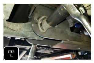
**Step 71** Snug up all 4 lower control arm mounting bolts, but do not fully tighten until the truck is on the ground at ride height.
