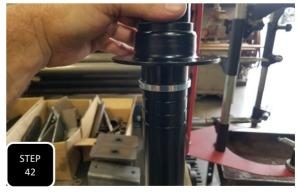
**Step 42** Once the retainer ring is set in the desired groove, install the retainer collar over the ring. Make sure that it slides completely over the clip. Next, install the new lower coil seat over the retainer collar. **NOTE: THE COIL SEAT NEEDS TO INSTALL LIKE A TOP HAT, NOT LIKE A BOWL. YOU SHOULD NOT BE ABLE TO SEE THE RETAINER COLLAR IF INSTALLED CORRECTLY.**
