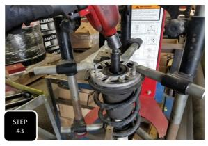
**Step 43** Using a suitable coil/strut compressor, compress the stock strut and remove the nut at the center of the top hat. Next, remove the strut from the middle. **NOTE: THE 3 STUD, TOP BOLT PATTERN IS NOT SYMETRICAL SO TAKE NOTE OF THE RELATIONSHIP BETWEEN THE TOP STUDS AND THE LOWER BAR PIN.**
