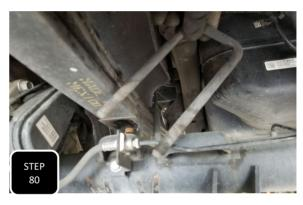
**Step 80** Working on one side at a time. Remove the factory spring plate and U-bolts, then lower the axle to make room for the lift block. **NOTE: SLIGHTLY LOOSEN THE U-BOLTS ON THE OTHER SIDE TO ALLOW EASIER MOVEMENT OF THE AXLE AND AN EASIER INSTALL OF THE BLOCK. "DO NOT REMOVE THE U-BOLTS ON THE OTHER SIDE"**
