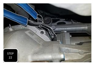
**Step 22** Lower the differential down a little bit and first disconnect the breather tube, then dis-engage all wire guide clips for the differential electrical plug.
