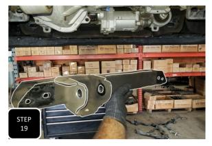
**Step 19** Unbolt the 4 bolts attaching the rearward control arm crossmember and remove the cross member.
