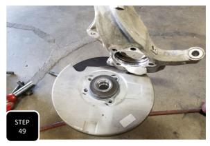
**Step 49** Remove the 4 bolts attaching the hub assembly to the steering knuckle and separate the two. **NOTE: IT WILL HELP TO HIT THE BACK OF THE HUB WITH A DEAD BLOW IF IT STICKS TO THE STEERING KNUCKLE.**
