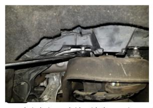
**Step 48** Locate the new, longer steering knuckles and install them on their designated side with the steering arm facing the front of the truck and the caliper mounting ears facing the rear of the truck. Use the factory hardware and torque to factory specs.
