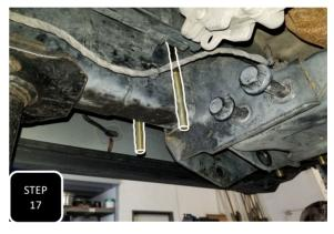
**Step 17** On both sides, slide the supplied U-bolt over the frame, just behind the cross member behind the factory radius arm bracket and allow it to hang vertically. **NOTE: 13-20 TRUCKS WILL UTILIZE BOTH SUPPLIED U-BOLTS. THE SUPPLIED NUT PLATE AND 1/2" X 9" BOLTS ARE ONLY FOR 2021+ MODELS.**
