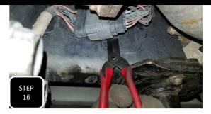
**Step 16** On the drivers side, unclip the wire guide from the inside of the frame and on the passenger side unclip the wire harness clip from the inside of the frame.
