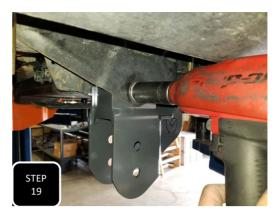
**Step 19** Loosely install the new radius arm bracket into the factory mount using the factory radius arm bolt in the main hole and the supplied hardware for the U-bolt. Push the bracket up tight against the frame and tighten the U-bolt first, then tighten the stock mounting bolt. Once tight, torque the factory bolt to 200 ft/lbs and the U-bolt to 100 ft/lbs.
