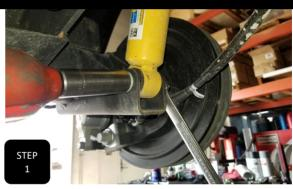
**Step 1** Jack up the rear of the truck and support under the frame with jack stands. Apply pressure to the rear diff with an adjustable jack and remove both rear shocks.
