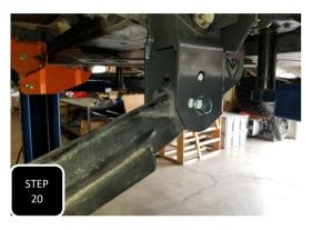
Install the radius arm into the: Upper hole for the 4" lift Lower hole for the 6" lift.
