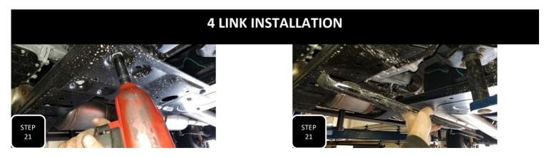
**Step 21** Unbolt and remove the skid plate under the transfer case and set aside to be re-installed later.
