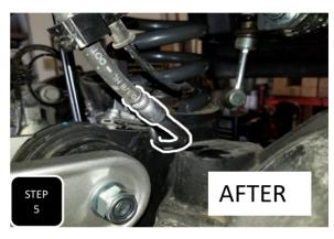
**Step 5** Locate where the brake line goes from soft line to hard line on the axle and gently bend the hardline upward so that it is at about a 45 degree angle to allow for more slack in the line.
