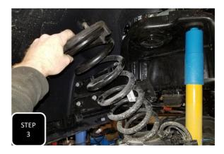
**Step 3** Move the jack to the driver's side of the axle and apply pressure. Then unbolt the drivers side shock from the axle and lower the axle so that you can remove the coil along with the rubber isolator.
