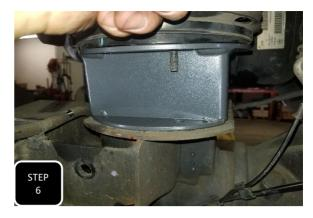
**Step 6** Remove the lower mounting nuts on both air bags, lower the axle and then install the air bag spacers under the air bags with the short side of the spacer facing the front of the truck. The round plate on the spacer will face up and attach to the air bag while the side of the spacer with the flat sides will bolt up to the axle.
