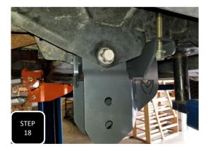
**Step 18** Slide the provided radius arm drop down bracket up into the factory mount and loosely attach using the factory bolt and the supplied U-bolt hardware.
