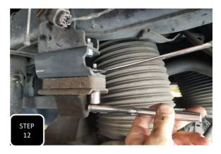
**Step 12** Unbolt the factory bump stops along with the 1" spacers. Next, install the bump stop extension brackets with the notched edge facing the back of the truck and the open end facing inward using the provided bolts and washers. Next, attach the factory bump stops along with the factory 1" spacer to the new bracket using the factory bolts and provided nuts/washers. Once everything is loosely attached, tighten it up.
