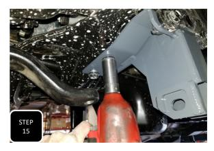
**Step 15** Install the new trac bar bracket using the original bolts along with the provided M14-2.0 nylock nuts. Make sure all the bolts are started in there threaded holes, then first, get all of the verticle bolts to a hand tight, then fully tighten the two horizontal bolts, and lastly tighten down the vertical bolts to factory spec.
