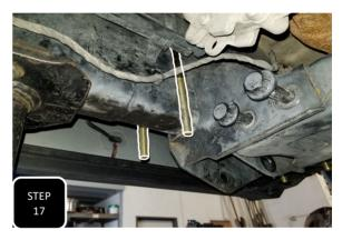
**Step 17** For the passenger side, slide the supplied U-bolt over the frame, just behind the cross member behind the factory radius arm bracket and allow it to hang vertically. **NOTE: 19-20 TRUCKS WILL UTILIZE BOTH SUPPLIED U-BOLTS. THE SUPPLIED NUT PLATE AND 1/2" X 9" BOLTS ARE ONLY FOR 2021+ MODELS.**
