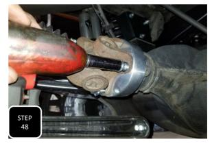
**Step 48** Insert the provided spacer, ensuring that the centering guides seat properly and then loosely install the provided M12-1.75 x 60 flange bolts.
