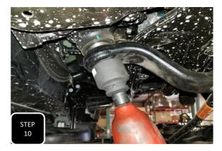
**Step 10** Apply a conservative amount of thread locker to the threads of the pitman arm nut then install the new, drop down pitman arm facing the same direction as the original one came off and torque to factory specs.
