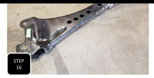
**Step 16** Working on one side at a time, remove the previously loosened radius arm bolts and then remove the radius arm.
