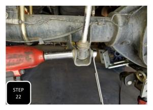
**Step 22** Install the new shocks and tighten. Max Trac shocks need to be installed with the shaft of the shock at the frame and the body at the axle. Fox shocks get installed opposite of that.
