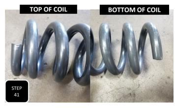
**Step 41** Place the rubber isolator on top of the new coil and install the coil. Make sure the nipple on the isolator aligns with the hole in the coil bucket then jack up the axle so that pressure is applied and re-attach the shock. **NOTE: THE COIL NEEDS TO BE INSTALLED WITH THE FLATTER SIDE FACING UPWARD AND THE PART # RIGHT SIDE UP.**
