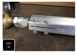
**Step 30** Get all 4 link arms in front of you with all of the Max Trac logos facing in the same direction and the two holed pinch seem facing up. Loosely install the provided M8 socket head bolts with the head of the bolt on the same side as the top of the Max Trac logo.
