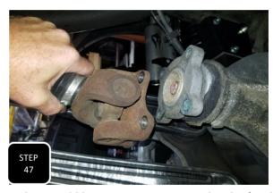
**Step 47** For Ram 2500 models, locate the front drive shaft spacer that would have come in your rear box kit for the 6" or 8" lift kit (907235 or 907255) Remove the 4 bolts mounting the drive shaft to the drive flange on the front pinion and separate.
