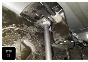
**Step 23** Loosely install the radius arm drop down bracket into the original mount using the factory bolt and then loosely attach the provided  $1/2-13 \times 9$ " bolts, washers, and lock washers to the nut plate on top of the frame. Push the bracket up tight to the frame and torque the factory bolt to factory specs and the 1/2" bolts to 90 ft/lbs.
