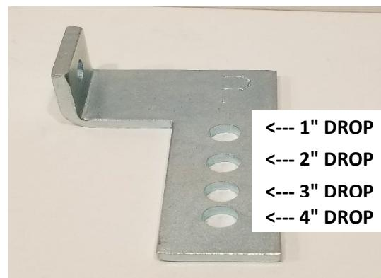
**Step 12** Attach the ball to the appropriate hole in the new sensor plate using the provided M6 nut and washer. The top hole is for 1" drop, 2nd down for 2", 3rd down for 3" and 4th down for 4" drop.
