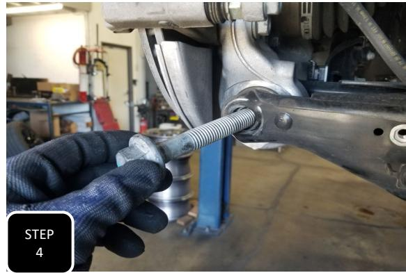
**Step 4** Unbolt the bolt attaching the lower control arm to the spindle and remove the bolt.
