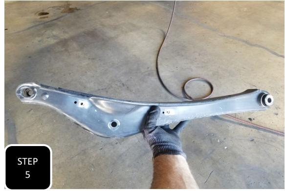
**Step 5** Remove the cam bolt attaching the lower control arm to the frame and then remove the lower control arm.
