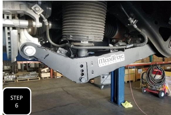
**Step 6** Locate the appropriate control arm for the side that you are working on and loosely install the the cam bolt at the frame. NOTE: The aluminum logo plate and brake line mounting brackets should be facing the rear of the truck.
