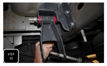
**Step 10** If installing the hangers in the 2 & 4 holes, you will need to bend the bed seem, directly above the spring hanger, for additional clearance.
