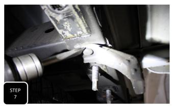
**Step 7** Next, you will need to chissel off the remainder of the heads using a pneumatic hammer with a chissel attachment and then finally punch out the body of the rivet using a pneumatic hammer with a punch attachment. Older models will have one more rivet attaching a support bracket to the bottom of the frame. This bracket will be welded on newer models and needs to be cut off.
