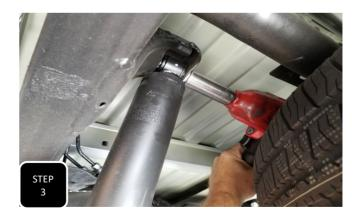
**Step 3** Jack up the jack slightly to apply pressure to the axle then unbolt both shocks at both ends and remove.
