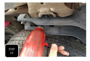
**Step 12** Jack the axle up and loosely attach the leaf spring to the shackle using the factory bolt facing from the inside, outward. Do not fully tighten any of the spring or shackle bolts until the truck is back on the ground at ride height. Next, re-install the trucks trailer hitch.
