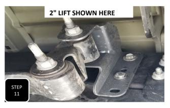
**Step 11** Attach the hanger with the shackle pre-assembled into it. The shackle can be installed with the open end facing either direction. The hanger will get attached using 3 of the provided 7/16" bolts and re-using the one factory bolt. **NOTE: THE SHACKLE CANNOT BE INSTALL AFTER THE HANGER IS INSTALLED.**
