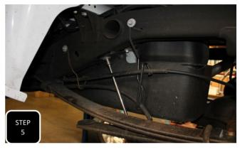
**Step 5** Working on one side at a time, remove the U-bolts and lower the axle away from the leaf spring. Next, pull the leaf spring/shackle out, around, and under the shackle mounting hanger. Now re-attach the leaf spring to the axle and torque the U-bolts to 100 ft/lbs. **REPEAT THIS STEP WITH THE OTHER LEAF SPRING.**
