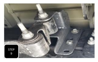
**Step 9** Before installing the hanger, attach the shackle to the hanger using the factory bolt, oriented from the inside out.
