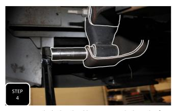
**Step 4** Unbolt the shackle mounting bolt at the frame on both sides and remove.
