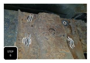
**Step 6** With the leaf springs now out of the way, you will need to remove the rear shackle hanger by making multiple cuts into the head of each of the 3 mounting rivets using a 4.5" cut off wheel. The bolt at the upper hole can just be un-bolted and saved for re-installation.
