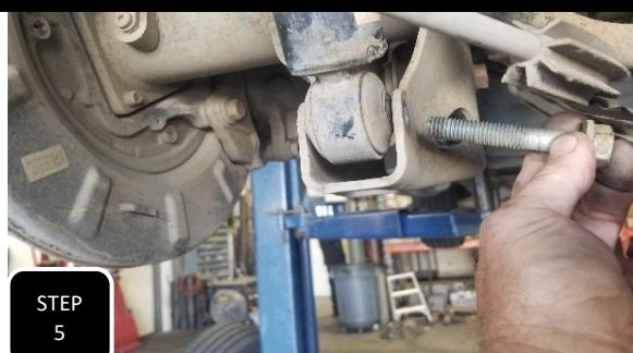
**Step 5** First, apply pressure to the diff with the adjustable jack. Next, unbolt both lower shock bolts at the axle and remove the bolts.
