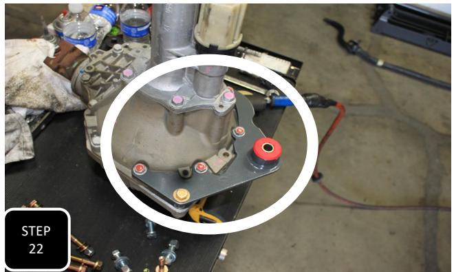
**Step 22** Take the differential and stand it upright on the driver's side axle flange. The breather port will leak a little if at a high point or a lot if at a low point. Place a vacuum cap over the breather for no fluid loss. Locate the provided dorsal fin diff bracket and line it up with the front side of the diff to see which bolts need to be removed.
