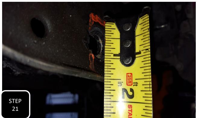
**Step 21** Moving over to the rearward lower control arm mount on the passenger side, Mark a vertical line, 3 inches from the inner edge of the frame where the original cross member was attached. Next, mark a horizontal line 1.5 inches up from the bottom. **NOTE: THIS SECTION BEING MARKED AND REMOVED IS ON THE FRONT SIDE OF THE CROSSMEMBER. THE SIDE FACING THE FRONT OF THE TRUCK.**
