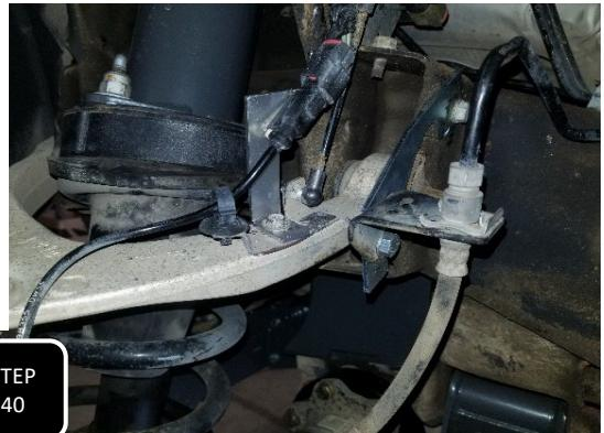
**Step 40** Using the provided loom clamp and factory 6 mm bolt, guide and attach the ABS line up the back side of the neck of the steering knuckle. Next, Locate the provided ABS line brackets and attach the bracket to the upper control arm using the factory 6 mm bolt, and then attach the ABS line plug to the bracket by pressing the clip and guide into the
