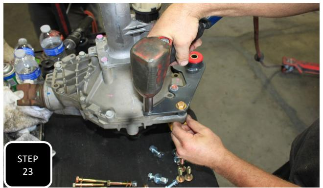
**Step 23** Remove the 4 bolts that the bracket aligns with and then install the bracket using the 4 provided M10-1.5 x 60 bolts and the 1 provided 7/16-14 x 3" bolt, nut, & washer then tighten. **NOTE: THE BRACKET WILL ONLY FIT ONE WAY AND ALWAYS TAKE CAUTION WHEN INSTALLING A STEEL BOLT INTO ALUMINUM THREADS.**
