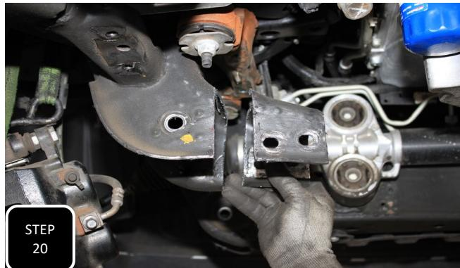
**Step 20** Working with the rearward lower control arm mount on the driver's side, mark a vertical line, 3 inches in from the inner edge where the original cross member was attached. Extend this mark straight up, across, and back down the front of the mount and then using a suitable cutting device, cut this section of the mount off.
