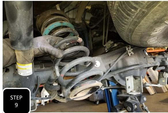
**Step 9** Lower down the axle and remove both coil springs. **NOTE: MAKE SURE TO SAVE THE RUBBER ISOLATORS FOR RE-INSTALLATION.**
