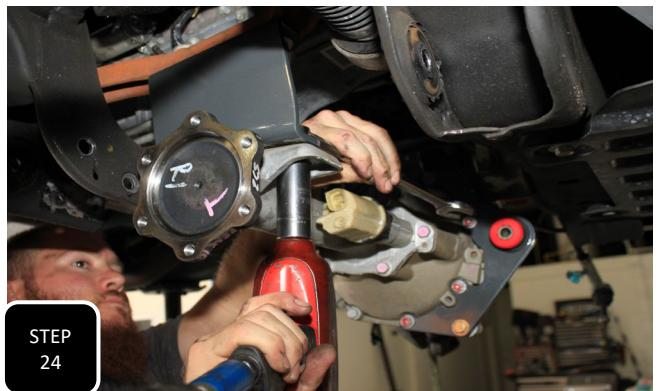
**Step 24** Place the differential back onto the adjustable jack and align it with the recently install diff drop brackets. Next, loosely attach the diff using the provided 1/2" bolts on the driver's side and 9/16" bolts on the passenger side. **NOTE: THE DIFF WILL GET FULLY TIGHTENED WHEN THE WHOLE FRONT END IS BACK TOGETHER.**
