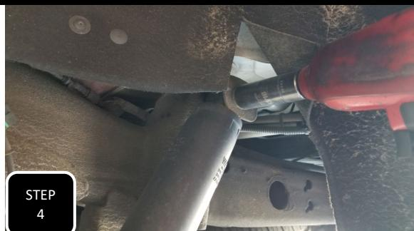
**Step 4** First, apply pressure to the diff with the adjustable jack. Next, to access the upper shock mount more easily, cut a slit in the wheel well liner and remove the upper mounting bolt of the shock.
