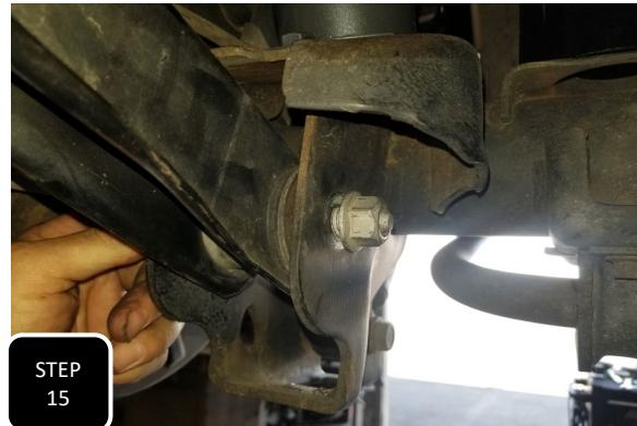
**Step 15** Loosely re-attach the lower control arm to the axle and only snug up the nuts. **NOTE: THESE BOLTS WILL GET FULLY TIGHTENED WHEN THE TRUCK IS BACK ON THE GROUND AT RIDE HEIGHT.**
