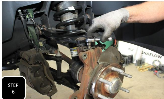
**Step 6** Unbolt the ABS sensor from the hub assembly and then the guide bracket from the top of the spindle. Support the ABS sensor out of the way so that it does not get damaged during the install.
