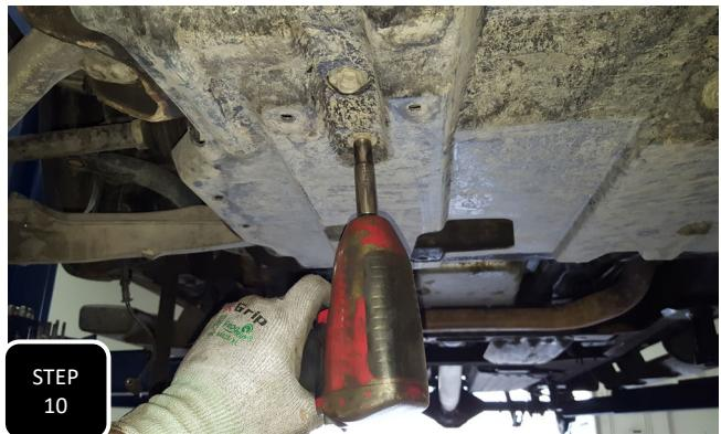
**Step 10** Unbolt and discard the plastic skid plate that covers from the bumper to the rear cross member of the lower control arms.
