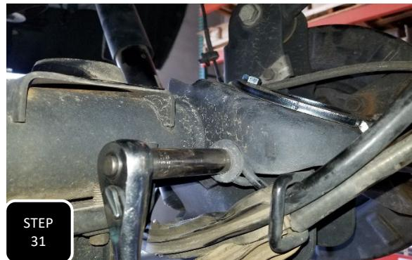
**Step 31** Jump on the rear bumper a few times to settle the suspension and then tighten all of the control arm/ trac bar bolts that were left loose to factory specs. Next, re-attach the E-brake cable guide bracket to the driver's side lower control arm and tighten.
