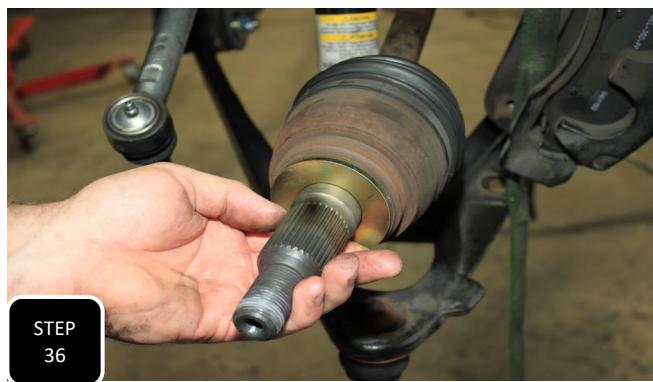
**Step 36** Slide the outer CV spacer onto the end of both axles with the chamfered I.D. side facing inward. The outer CV spacer is the 2 3/4" gold ring with a chamfered I.D. on one side.
