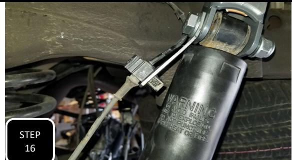
**Step 16** Loosely install the provided shock extenders with the logo facing outward, using the factory shock bolt. Next, attach the shock to the extender using the provided 14mm bolt, nut and washer and fully tighten both bolts. **NOTE: ON THE DRIVER'S SIDE, YOU WILL ATTACH THE PROVIDED ABS LINE BRACKET TO THE SHOCK MOUNTING BOLT AT THE FRONT OF THE EXTENDER WITH THE BRACKET POINTED STRAIGHT DOWN.**
