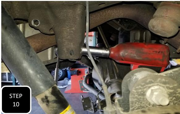
**Step 10** Unbolt the trac bar from the mount on the frame and separate.
