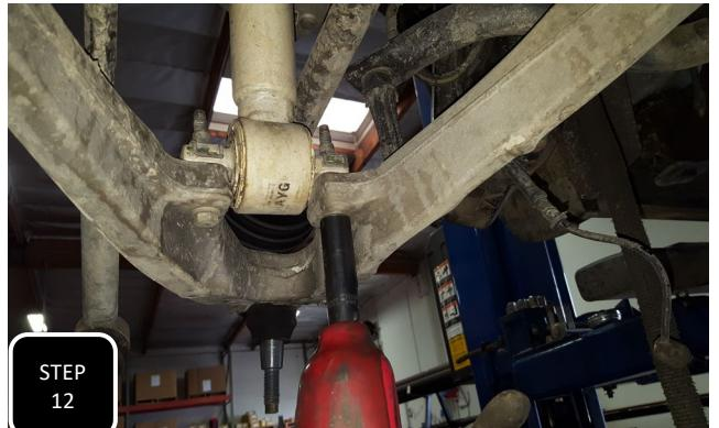
**Step 12** Remove the 3 nuts attaching the strut to the frame and the two bolts attaching the strut to the lower control arm, then remove the strut.
