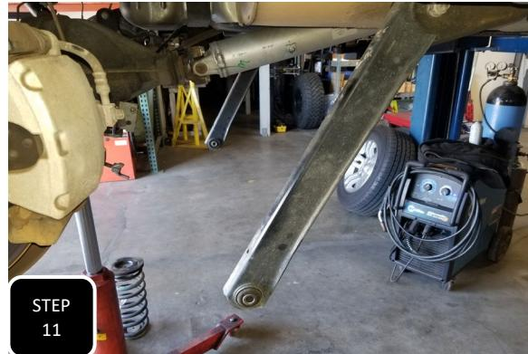
**Step 11** Make sure the adjustable jack under the diff has a provision to keep the diff from rotating, then unbolt both lower link arms from the axle, loosen the bolts at the frame, and allow them to both drop down, away from the axle. **NOTE: IF THE PINION IS NOT SUPPORTED, THE DIFF WILL WANT TO ROTATE DOWN.**
