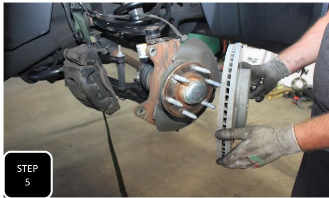
**Step 5** Unbolt the rotor retainer bolt and then remove the rotor. **NOTE: THE ROTOR SHOULD JUST POP OFF. IF IT DOES NOT JUST POP OFF, YOU WILL NEED TO HIT THE WHEEL MOUNTING SURFACE OF THE ROTOR WITH A HAMMER UNTIL THE RUSTY BOND IS BROKEN AND THE ROTOR POPS OFF.**
