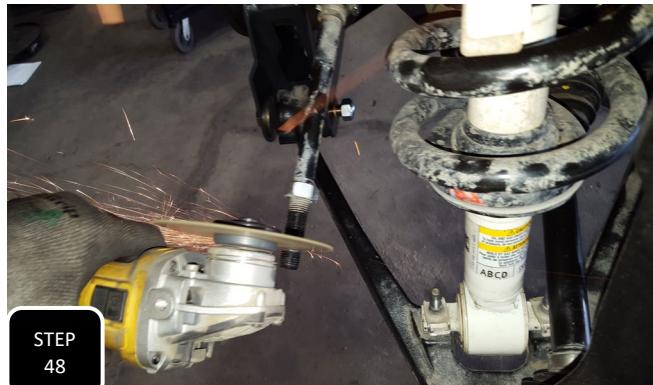
**Step 48** Mark a line  $9/16"$  in from the threaded end of the inner tie rod and cut this section off. **NOTE: MAKE SURE TO CLEAN UP THE END SO THAT THE OUTER TIE ROD CAN THREAD BACK ON PROPERLY.**
