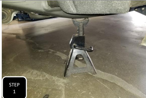
**Step 1** Jack up the rear of the truck and support under the frame rails with jack stands. Keep an adjustable jack under the diff for height adjustment.
