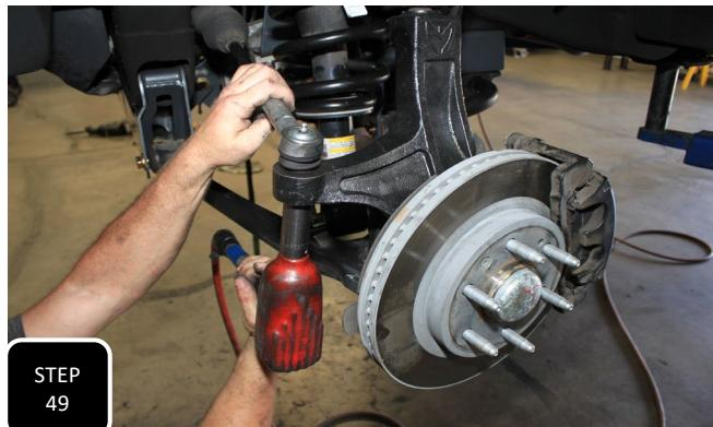
**Step 49** Once both ends are trimmed down, thread them back together and attach the tie rod to the steering knuckle using the factory nut.
