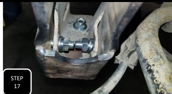
**Step 17** Loosely install the provided shock extenders, using the provided 1/2" bolts, lock washers and jam nuts through the original shock mounting holes, from the outside inward. You will then install the provided 1/2" bolts through the bottom hole and attach using the provided nylock nuts.
