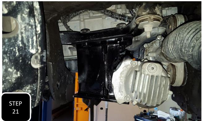
**Step 21** Locate and install the passenger side diff drop and attach it to the factory mount using the factory nuts, then tighten. **NOTE: THE SHORT SIDE OF THE MOUNT WILL FACE THE REAR OF THE TRUCK**
