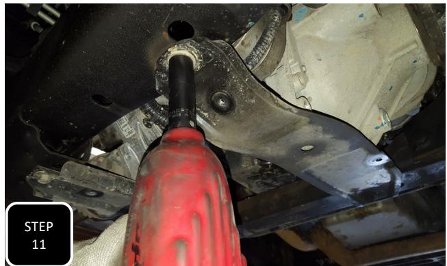
**Step 11** Remove and discard the two metal skid plates under the front diff and the steering rack.
