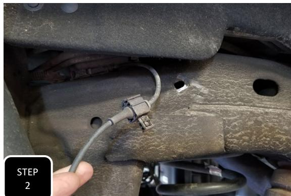
**Step 2** Separate the ABS guide clip, on each side, from the frame to allow for more slack during the install.
