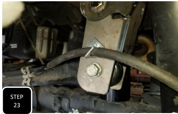
**Step 23** Slide the E-brake guide bracket onto the E-brake cable near the trac bar bracket on the passenger side and then attach this bracket to the small hole on the back of the trac bar bracket using the provided 8mm bolt nut and washers. **NOTE: DO NOT FULLY TIGHTEN THIS BRACKET. ONLY SNUG IT UP AS IT WILL NEED TO PIVOT AS THE SUSPENSION CYCLES.**
