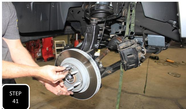
**Step 41** Install the rotor and secure the factory retainer screw.
