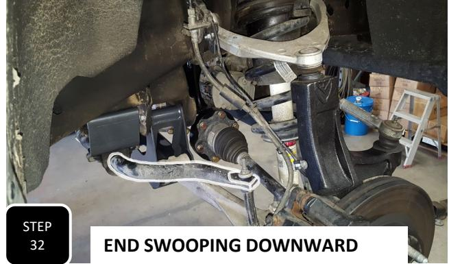
**Step 32** The ends of the sway bar originally swooped upward. The sway bar will now get re-installed with the ends swooping downward, the opposite of how they were. Use the factory bolts along with the provided nuts and washers to attach the sway bar to the drop down brackets and tighten.
