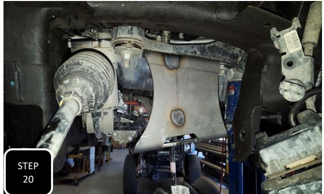
**Step 20** Locate the driver's side diff drop and install it to the factory mount using the factory hardware. The driver's side bracket has the tab that extends past the bracket and an extra hole for the guide nipple in the factory mount. **NOTE: THE SHORT SIDE OF THE MOUNT WILL FACE THE REAR OF THE TRUCK.**
