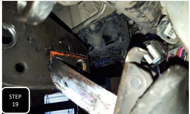
**Step 19** Using a suitable cutting device, cut along both of your lines and remove the rectangular section that was created. Spray paint all raw edges for rust prevention.
