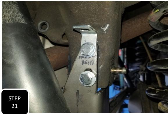
**Step 21** Re-install the bracket using the provided zinc plated crush tube and 14mm hardware. Next, install the provided 7/16" bolts, nuts, and washers through the two side holes. You will also be attaching the provided pass side ABS line bracket to the upper bolt with the "D" shaped hole facing upward, then tighten all 3 bolts.
