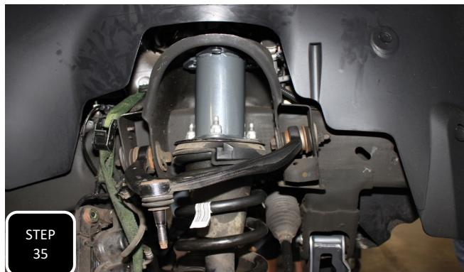
**Step 35** Fully tighten the upper mounting nuts and the lower mounting bolts for both struts.
