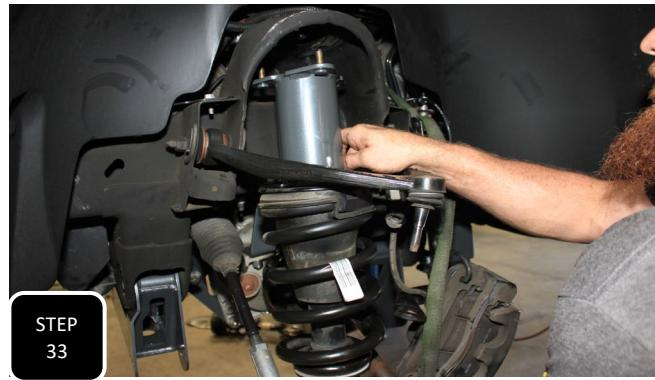
**Step 33** Locate the two struts and attach the strut spacer to the top using the factory nuts. Next, loosely install both sides using the provided nuts. **NOTE: THE SPACERS WILL ONLY FIT ONE WAY AND DO NOT FULLY TIGHTEN THE NUTS AT THE FRAME AT THIS TIME.**
