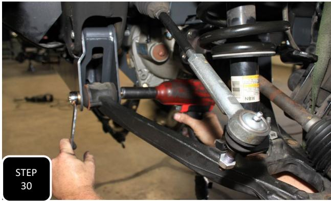
**Step 30** Now that the suspension is settled and the vehicle is sitting at ride height, go back and tighten all of the bolts that were left loose. **NOTE: TIGHTENING THE CONTROL ARM BUSHINGS AND DIFFERENTIAL WHILE THE TRUCK IS AT RIDE HEIGHT WILL ENSURE THE DIFF IS CENTERED AND PROLONG THE LIFE OF THE BUSHINGS.**
