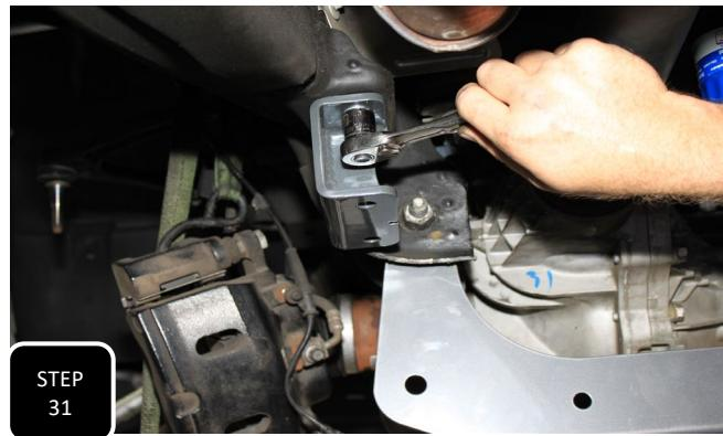
**Step 31** Install the sway bar drop down brackets using the supplied M10 bolts and washers. The open end of the bracket will face the inside of the truck and the bracket needs to swoop towards the rear of the truck.
