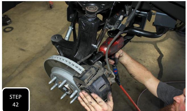
**Step 42** Unbolt the factory bracket that attaches the brakeline to the frame to gain extra slack in the line. Next, attach the brake caliper to the steering knuckle using the factory bolts and tighten.
