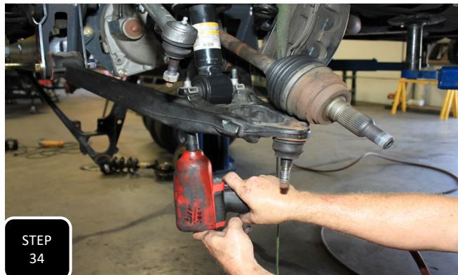
**Step 34** Loosely attach both lower control arms using the provided 5/8" hardware and then swing the arms up and loosely attach them to the bottom of the strut using the factory hardware. **NOTE: DO NOT FULLY TIGHTEN THE LOWER CONTROL ARM BUSHINGS UNTIL THE TRUCK IS BACK ON THE GROUND AT RIDE HEIGHT.**
