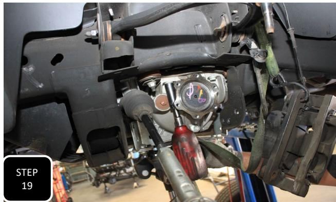
**Step 19** Support the differential with an adjustable jack and then remove all 4 mounting bolts. Slowly lower the diff down making sure that there is nothing else attached to it that could get damaged. **NOTE: YOU WILL NEED TO UNPLUG THE 3 PLUGS AT THE STEERING RACK TO ACCESS ONE OF THE DIFF BOLTS.**
