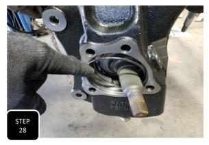
**Step 28** Remove the "O" ring that is in the hub bore of the factory steering knuckle and install it in the new steering knuckle. **NOTE: APPLY SOME WD-40 OR OTHER LUBE ON THE "O" RING TO EASE THE INSTALL OF THE HUB ASSEMBLY.**
