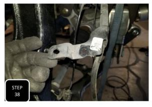
**Step 38** The tab on the brake line mounting bracket that originally mounted the brake pad sensor wire needs to be bent so that it is now straight, not at 90 degrees from the main bracket.
