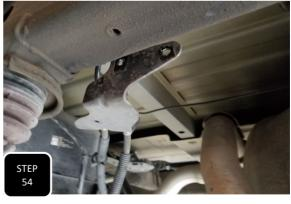
**Step 54** Remove both mounting bolts for the brake line bracket located on the inside of the driver's side frame.
