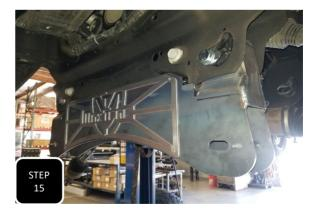
**Step 15** Loosely install the front cross member using the provided M18-2.5 x 120 bolts and the logo plate facing the front of the truck. **NOTE: DO NOT FULLY TIGHTEN THESE BOLTS AT THIS TIME.**
