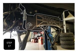
**Step 17** Loosely install both lower control arms using the factory cam bolts. **NOTE: DO NOT FULLY TIGHTEN THESE BOLTS AT THIS TIME.**
