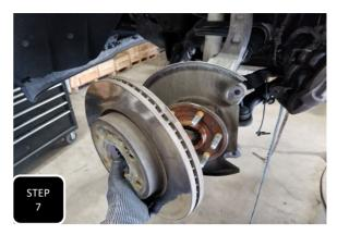
**Step 7** Unbolt the rotor retainer screw and then remove the brake rotor. **NOTE: IF THE ROTOR DOES NOT JUST POP OFF THEN YOU WILL NEED TO HIT THE SURFACE THAT THE WHEEL MOUNTS TO, WITH HAMMER, IN DIFFERENT SPOTS UNTIL THE CORROSIVE BOND IS BROKEN.**
