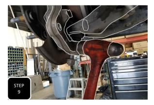
**Step 9** Loosen the lower ball joint nut, but do not remove it. Hit the side of the spindle, right at the ball joint, with a hammer to break it loose. The nut will catch the spindle, then remove the spindle.
