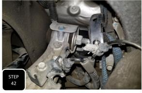
**Step 42** Separate the ABS sensor wire from both mounting points on the bracket at the upper control arm and then reroute the wire underneath the upper control arm instead of above it as it was from the factory.
