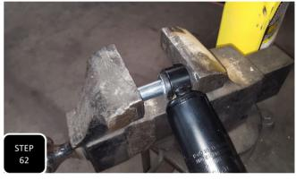
**Step 62** Locate your new longer rear shocks and shock hardware. Next, lube up the bushing on both ends of the shocks and using a bench vise, press the new shock sleeves in. **NOTE: IT HELPS THE PRESSING PROCESS TO PIVOT THE SHOCK UP AND DOWN WHILE CLOSING THE VISE.**
