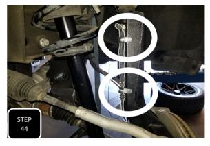
**Step 44** Separate the intermediate ABS line bracket from the rubber grommet on the line and then attach the ABS line to the front of the neck of the steering knuckle using the provided 3/8" loom clamps and M6 hardware.
