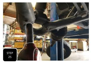
Step 25 Fully tighten the upper nuts and lower bolts for both struts.
