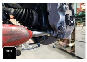
**Step 31** Install the brake caliper using the factory bolts and torque to factory specs.
