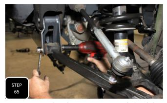
**Step 65** Now that the suspension is settled and the vehicle is sitting at ride height, go back and tighten all of the bolts that were left loose. **NOTE: TIGHTENING THE CONTROL ARM BUSHINGS WHILE THE TRUCK IS AT RIDE HEIGHT WILL PROLONG THE LIFE OF THE BUSHINGS.**
