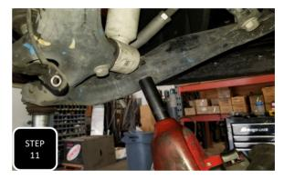
**Step 11** Unbolt the 3 nuts at the top of the strut and the 2 bolts at the bottom of the strut and then remove the strut.
