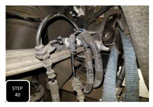
**Step 40** Unclip the brake pad wire from the mount at the upper control arm and then flip the clip up-side down and reinstall it back into the same hole.
