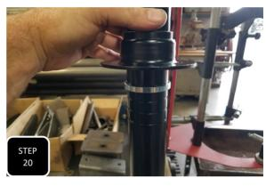
**Step 20** Once the retainer ring is set in the desired groove, install the retainer collar over the ring. Make sure that it slides completely over the clip. Next, install the new lower coil seat over the retainer collar. **NOTE: THE COIL SEAT NEEDS TO INSTALL LIKE A TOP HAT, NOT LIKE A BOWL. YOU SHOULD NOT BE ABLE TO SEE THE RETAINER COLLAR IF INSTALLED CORRECTLY.**
