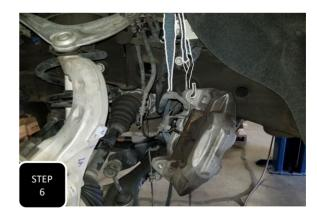
**Step 6** Remove the brake caliper and support it up, out of the way. **NOTE: NEVER ALLOW THE CALIPER TO HANG BY THE BRAKE LINE.**
