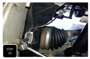
**Step 33** Unclip the ABS line from the mounting bracket at the upper control arm to gain slack in the line. Next, install the ABS sensor in the mounting hole at the front of the steering knuckle and attach it using the factory M6 bolt.
