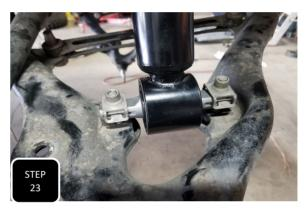
**Step 23** Use a flat head screw driver to pop the threaded clips off of the bar pin on the stock strut and then pop the clips onto the bar pin of the new strut.
