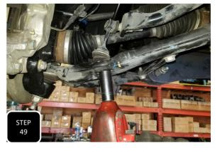
**Step 49** The sway bar will need to be flipped from its original position so that the middle of the bar swoops upward. Loosely attach the sway bar to the drop down brackets using the provided M10 hardware and attach the sway bar end links into the lower control arms using the factory nuts. Once everything is aligned, then fully tighten all connecting points.
