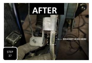
**Step 37** Locate the brake line mounting bracket in the middle of the brake line and slide it up the line about the same length as the height of the bracket.
