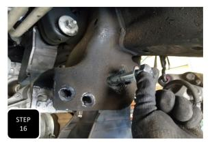
**Step 16** Loosely install the rear subframe using the provided M18-2.5 x 120 bolts. The side with all of the extra holes in it will need to face the rear of the truck. **NOTE: DO NOT FULLY TIGHTEN THESE BOLTS AT THIS TIME.**
