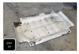
**Step 14** If your truck is equipped with one, remove the aluminum skid plate located below the lower control arm mounts and discard it.
