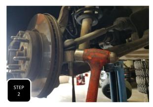
**Step 2** Loosen the tie rod at the spindle and break loose by hitting the side of the spindle, at the steering arm, with a hammer. **NOTE: NEVER HIT THE TIE ROD ON THE THREADS.**
