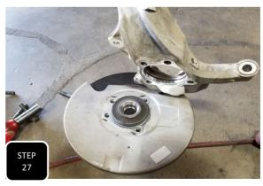
**Step 27** Remove the 4 bolts attaching the hub assembly to the steering knuckle and separate the two. **NOTE: IT WILL HELP TO HIT THE BACK OF THE HUB WITH A DEAD BLOW IF IT STICKS TO THE STEERING KNUCKLE.**
