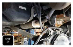
**Step 60** Locate and install the ABS wire bracket for the top of the differential. Attach it to the diff using the factory hardware and then attach the ABS line block to the bracket using the provided 1/4" hardware.
