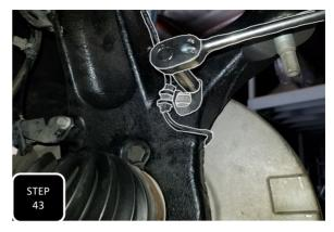
**Step 43** Attach the ABS sensor to the steering knuckle using the factory M6 bolt. Next, attach the lower wire guide bracket to the back of the steering arm on the knuckle using the factory M6 bolt.
