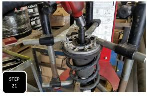
**Step 21** Using a suitable coil/strut compressor, compress the stock strut and remove the nut at the center of the top hat. Next, remove the strut from the middle. **NOTE: THE 3 STUD, TOP BOLT PATTERN IS NOT SYMETRICAL SO TAKE NOTE OF THE RELATIONSHIP BETWEEN THE TOP STUDS AND THE LOWER BAR PIN.**
