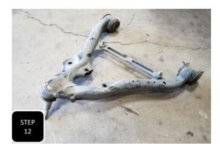
**Step 12** Unbolt both bolts attaching the lower control arm to the frame and remove the lower control arm.
