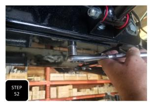
**Step 52** Attach the skid plate to the bottom of both subframes using the supplied M12 socket head screws on the front crossmember and the supplied 7/16" hardware at the rearward subframe then tighten. All bolts can get torqued to 45 ft/lbs.
