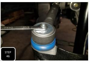
**Step 46** Locate the new, shorter outer tie rod end and thread it onto the inner tie rod end until it is able to connect to the steering knuckle when the steering knuckle is positioned with the rotor parallel to the frame. Next, install the grease fitting and add a little bit of grease to the joint. Lastly, tighten up the rod end to the steering knuckle using the provided nut.
