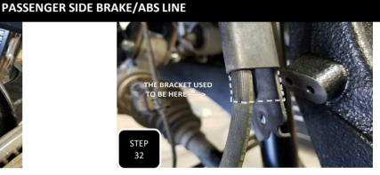
**Step 32** Attach the brake line guide bracket to the side of the spindle using the factory M6 bolt and tighten. Next, pull the brake line down through the mounting bracket to gain some slack between the brake caliper and mounting bracket.
