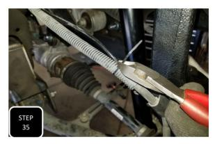
**Step 35** Using two of the provided zip ties, attach the remainder of the ABS line to the brake line and then trim off the tail of the un-used zip tie.
