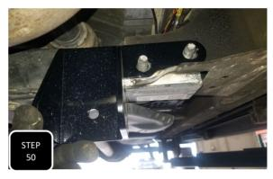
**Step 50** Locate the crossmember under the transfer case and remove the nuts from both mounting bolts on both sides. Next, Loosely install the supplied kicker bar brackets on the front side of the crossmember, push them upward so that the bottom of the backets contacts the bottom of the crossmember and then tighten.
