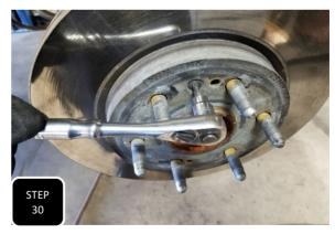
**Step 30** Install the brake rotor onto the wheel studs and secure it using the factory retainer screw.
