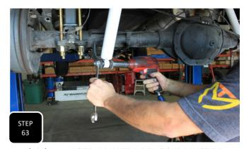
Step 63 Install the new longer shocks using the factory hardware and tighten. NOTE: MAX TRAC SHOCKS MUST BE MOUNTED WITH THE BODY AT THE AXLE AND THE SHAFT AT THE FRAME OR THEY WILL NOT WORK PROPERLY. FOX SHOCKS WILL MOUNT THE OPPOSITE, WITH THE BODY ON THE FRAME AND SHAFT AT THE AXLE.
