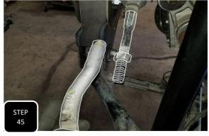
**Step 45** Loosely install the outer tie rod into the steering knuckle to keep the tie rod from rotating while you loosen the jam nut. Break the jam nut loose and then completely unthread and remove the outer tie rod end.
