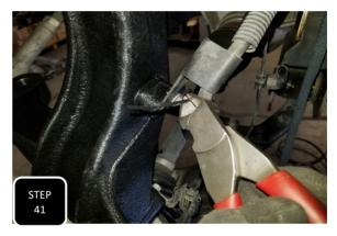
**Step 41** Attach the brake pad sensor wire to the brake line using two of the provided zip ties and then clip of the excess of unused zip tie.
