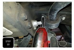
**Step 10** Unbolt the sway bar end links from each lower control arm and then unbolt all 4 frame mounting bolts and remove the entire sway bar.
