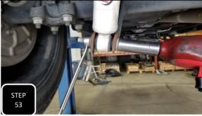
**Step 53** Support the rear axle with an adjustable jack and then unbolt both rear shocks at both ends and remove.
