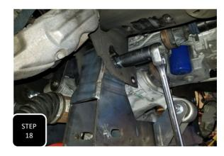
**Step 18** Fully tighten all 4 bolts that attach the subframes to the frame and torque to 170 ft/lbs.
