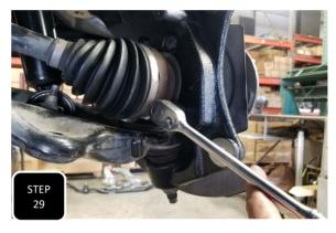
**Step 29** Install the hub assembly into the the new steering knuckle using the factory bolts and torque to 120 ft/lbs.
