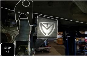
**Step 48** Locate the two sway bar drop down brackets and install them sloped side at the frame and "MT" logo facing outward, using the factory hardware.
