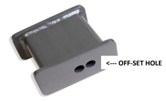
**Step 57** Install the new lift block and longer U-bolts. The lift block is angled and the short side must face the front of the truck. **NOTE: THE MAX TRAC LIFT BLOCK HAS TWO CENTER PIN HOLES. INSTALL THE CENTER PIN IN THE OFF-SET HOLE, WHICH WILL PUSH THE AXLE 1 INCH FORWARD AND MINIMIZE DRIVELINE PLUNGE.**
