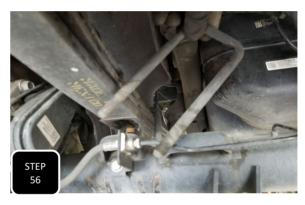
**Step 56** Working on one side at a time. Remove the factory spring plate and U-bolts, then lower the axle to make room for the lift block. **NOTE: SLIGHTLY LOOSEN THE U-BOLTS ON THE OTHER SIDE TO ALLOW EASIER MOVEMENT OF THE AXLE AND AN EASIER INSTALL OF THE BLOCK. "DO NOT REMOVE THE U-BOLTS ON THE OTHER SIDE"**
