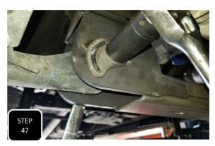
**Step 47** Snug up all 4 lower control arm mounting bolts, but do not fully tighten until the truck is on the ground at ride height.
