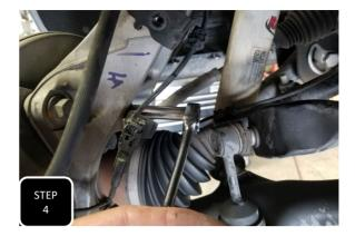
**Step 4** Unbolt any and all other ABS wire guide brackets from the spindle and save the hardware for re-installation.
