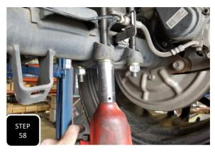
**Step 58** Loosely tighten the U-bolts and then install the lift block and U-bolts on the other side. Once both blocks have been installed, torque the U-bolts to 100 ft/lbs.
