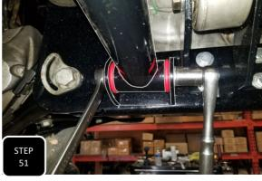
**Step 51** Locate the smaller, clevis looking kicker bar brackets and loosely install them onto the back of the rearward subframe using the supplied 3/8" hardware. Next, loosely install the kickerbars using the supplied 1/2" hardware. Once both kicker bars have been loosely installed, fully tighten both mounts and then lastly tighten all 4 kicker bar bolts. All 1/2" bolts get torqued to 60 ft/lbs, 3/8" bolts to 30 ft/lbs, & the M18 crossmember bolts to 150 ft/lbs.
