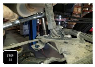
**Step 55** Unbolt the two bolts that attach the ABS wiring to the top of the differntial and allow the wiring to hang loose until the lift blocks are installed.
