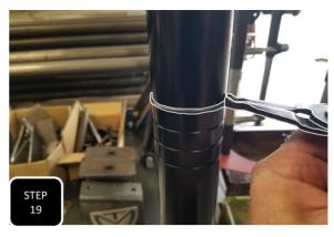
**Step 19** Locate the new lift strut and using a set of retainer ring pliars, install the snap ring into the groove of the desired lift height. The lowest groove is for a 7" lift, the second groove from the bottom is for an 8" lift, the third groove from the bottom is for a 9" lift and the top groove is for a 10" lift.
