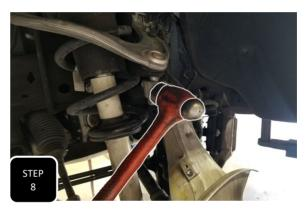
**Step 8** Loosen the upper ball joint nut, but do not remove it. Hit the side of the spindle, right at the ball joint, with a hammer to break it loose. The nut will catch the spindle.
