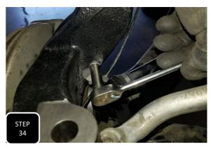
**Step 34** Remove the higher up guide bracket from the ABS line and then attach the lower down bracket (the bracket that is near the ABS sensor) to the back side of the steering arm using the factory M6 bolt. **NOTE: STEER THE SPINDLE BACK AND FORTH TO ENSURE THAT THERE IS ENOUGH SLACK IN BOTH THE ABS LINE AND BRAKE LINE, THAT THEY DO NOT GET TIGHT AT ANY POINT.**
