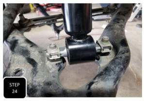
**Step 24** Loosely install the new strut assembly into the strut tower using the factory nuts. Next, swing up the lower control arm and loosely attach it to the bottom of the strut using the factory bolts.
