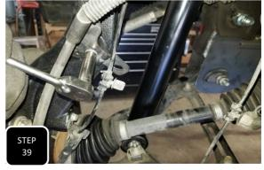
**Step 39** Attach the first brake pad sensor wire to the spindle using the factory M6 bolt. Next, attach the brake line guide bracket to the side of the spindle using the factory M6 bolt.
