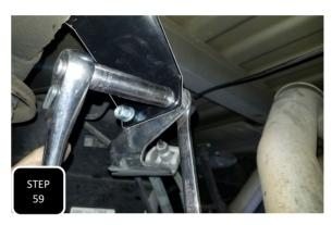
**Step 59** Locate the brake line bracket and install it between the frame and the factory brake line bracket on the inside of the driver's side frame rail. Attach it to the frame using the factory bolts and attach the factory brake bracket to this bracket using the provided M8 hardware. **NOTE: THE BRAKE LINE BRACKET IS THE LARGER "Z" SHAPED BRACKET.**
