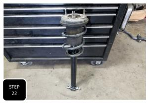
**Step 22** While the stock spring is still compressed, install the new lift strut along with the factory bump stop and tighten using the provided nylock nut. **NOTE: MAKE SURE TO CLOCK THE LOWER BAR PIN THE SAME AS IT WAS WHEN YOU REMOVED THE FACTORY STRUT FROM THE ASSEMBLY.**
