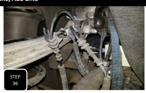
**Step 36** Separate the brake pad sensor wire guide bracket from the brake line guide bracket by detaching where the two brackets clip together. Next, separate the brake pad sensor wire from the bracket at the upper control arm.
