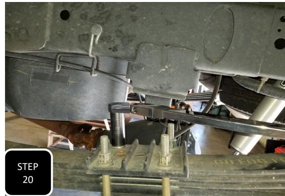
**Step 20** Jack up the rear axle to seat both the block and spacer, install the U-bolts, and torque them to 100 ft/lbs. Next, tight both new bolts from the spacer to the axle as well as both studs attaching the spacer to the air bag.
