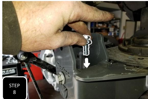
**Step 8** Slide the new trac bar bracket over the factory trac bar bracket on the axle and loosely install the factory bolt through the original trac bar mounting hole with the provided crush tube in the middle. Next, install one of the provided 3/8" bolts and washers through the inside, bottom of the bracket. **NOTE: DO NOT FULLY TIGHTEN EITHER OF THESE BOLTS AT THIS TIME.**
