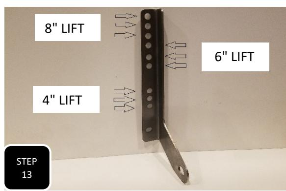
**Step 13** There are 9 mounting holes on the new sensor bracket. The 3 lowest holes are for a 1.5" rear lift, the 3 middle holes are for a 3.5" rear lift, and the 3 upper holes are for a 5.5" rear lift. Install the factory mounting ball into the desired hole using the provided M6 nut and washer then attach the sensor rod to it. **NOTE: THE MIDDLE HOLE OF EACH SET OF HOLES IS THE STARTING HOLE AND THE ABOVE OR BELOW HOLES WILL LIFT OR LOWER THE REAR OF THE TRUCK BY ABOUT 1/2".**
