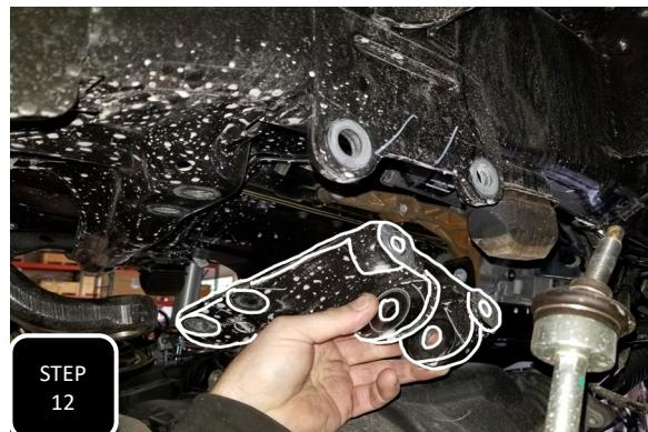
**Step 12** Remove the 5 bolts attaching the trac bar bracket to the frame and then remove the factory trac bar bracket.
