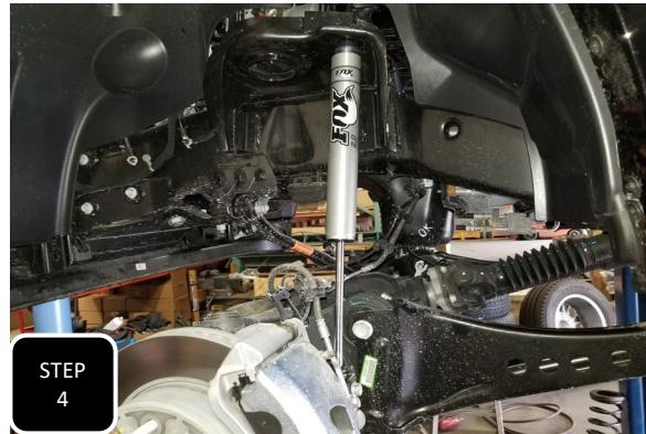
**Step 4** Completely remove the driver's side shock and loosely install the new shock as support for the axle while you are installing the lift. Next, repeat steps 3-4 on the passenger side and then move the jack back to the driver's side.
