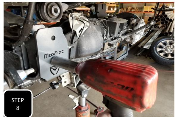
**Step 8** Tighten down the 3/8" bolt at the bottom of the trac bar bracket. The easiest way to hold the head of the bolt tight is to wedge a flat head screw driver down against the head. Next, tighten down the bolt in the original trac bar mounting hole.
