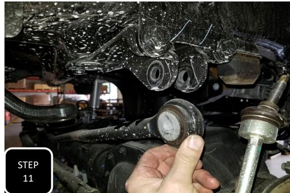
**Step 11** Remove the bolt attaching the trac bar to the bracket on the frame and separate. Allow the trac bar to rest on the axle.
