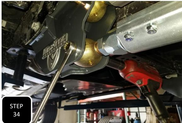
**Step 34** Tighten down the frame side bolts of the links completely and the axle side only hand tight. The axle side will get fully tightened when the truck is back on the ground at ride height.
