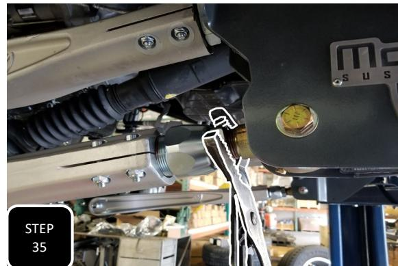
**Step 35** Tighten down all 4 of the M8 pinch bolts and then cinch down the two jam nuts on the rod ends.
