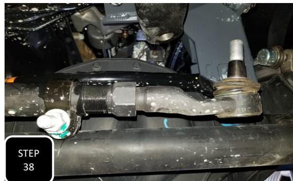
**Step 38** Loosen the clamp on the tie rod and adjust it out until you are able to rotate the rod end 180 degrees and then adjust it back in. **NOTE: THERE IS A PIN INSIDE THE TIE ROD THAT PREVENTS YOU FROM ROTATING THE END UNTIL YOU UNSCREW IT FAR ENOUGH TO DISENGAGE IT FROM THE PIN.**
