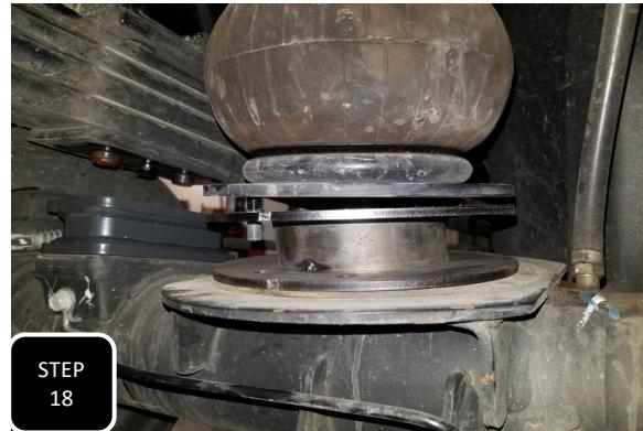
**Step 18** Install the lift block and the air bag spacer. The airbag spacer is off-set and when installed properly, the upper plate should off-set towards the rear of the truck with the ovalized holes facing the rear of the truck.
