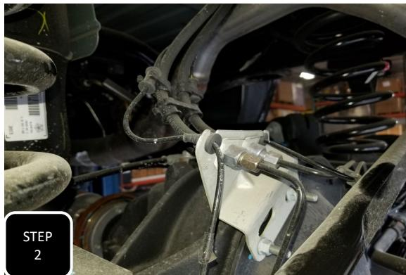
**Step 2** Using a crescent wrench or channel locks, grab the brake line bracket on the diff and bend it backwards to gain slack in the brake lines.
