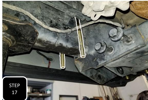
**Step 17** For the passenger side, slide the supplied U-bolt over the frame, just behind the cross member behind the factory radius arm bracket and allow it to hang vertically. **NOTE: 19-20 TRUCKS WILL UTILIZE BOTH SUPPLIED U-BOLTS. THE SUPPLIED NUT PLATE AND 1/2" X 9" BOLTS ARE ONLY FOR 2021+ MODELS.**
