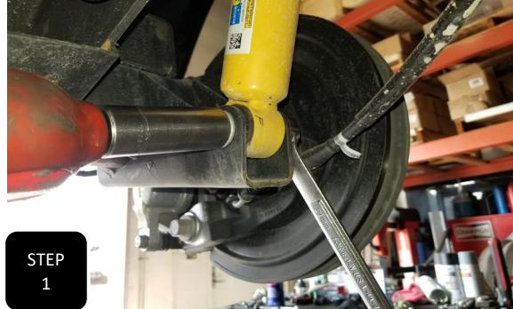
**Step 1** Jack up the rear of the truck and support under the frame with jack stands. Apply pressure to the rear diff with an adjustable jack and remove both rear shocks.
