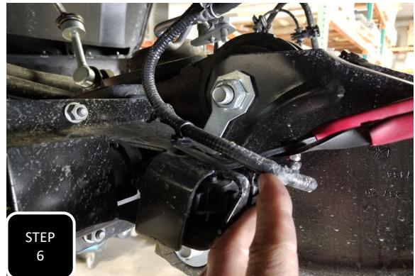
**Step 6** Unbolt the brake line bracket on both axles and unclip the wiring harness for the 4wd module.
