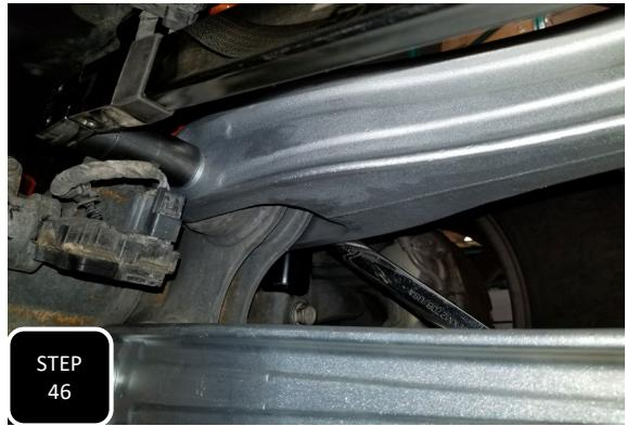
**Step 46** Re-install the wheels and tires then lower the truck to the ground. Once at ride height, tighten down the trac bar to the bracket and the links to the axle. All 5 bolts will get torqued to 200ft/lbs. **NOTE: IF INSTALLING THE RADIUS ARM KIT YOU WILL ALSO TIGHTEN THE BOLT AT THE FRAME BRACKET NOW.**
