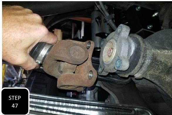
**Step 47** For Ram 2500 models, locate the front drive shaft spacer that would have come in your rear box kit for the 6" or 8" lift kit (907235 or 907255) Remove the 4 bolts mounting the drive shaft to the drive flange on the front pinion and separate.
