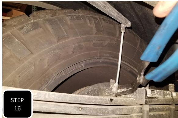
**Step 16** Unbolt both air bag bolts on the side you are working on and then disconnect the sensor rod from the spring plate by popping the socket off of the mounting ball.
