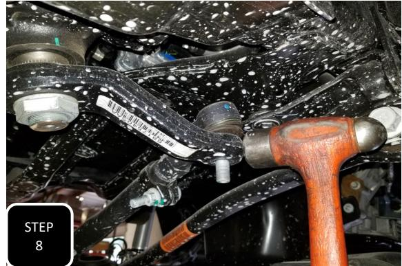
**Step 8** Remove the nut attaching the drag link to the pitman arm then break the drag link loose by hitting the side of the pitman arm with a hammer, right at the joint, then separate. **NOTE: NEVER HIT THE THREADS OF THE ROD END.**
