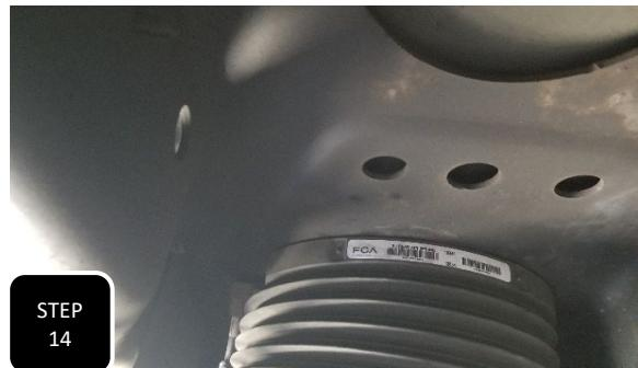
**Step 14** Install the wheels/tires and lower the vehicle down to the ground, but with the lift still holding the weight of the vehicle. First, ensure that the top of the air bag is properly aligned in the guide hole of the frame and then, second, turn the ignition on and allow the air bags to fill up before lowering the lift completely to the ground.
