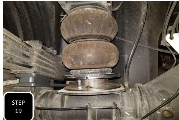
**Step 19** Before jacking up the axle and seating the block/air bag spacer, insert the new mounting bolts into the bottom plate from the top down and get the nut started on factory stud. **NOTE: WITH THE 1.5" REAR LIFT, THERE WILL NOT BE ROOM TO INSERT THE NEW BOLT WHEN THE STUD IS COMPLETELY INSERTED.**
