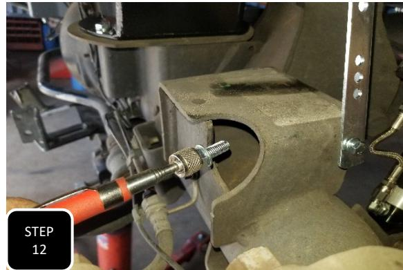
**Step 12** Unbolt the sensor rod ball from the mount on the axle and install the provided sensor brackets using the M6 bolt/washer at the original hole and the provided M8 bolt, nut & washer at the blank hole around the corner from the original bolt. **NOTE: USING A MAGNET WILL EASE THE PROCESS OF INSTALLING THE BOLT IN THE BLOCK ON THE AXLE.**
