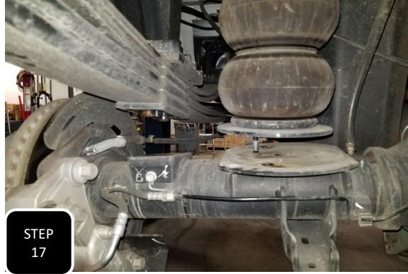
**Step 17** One side at a time, loosen both U-bolts, remove the U-bolts, and lower the axle to make room for the lift block.
