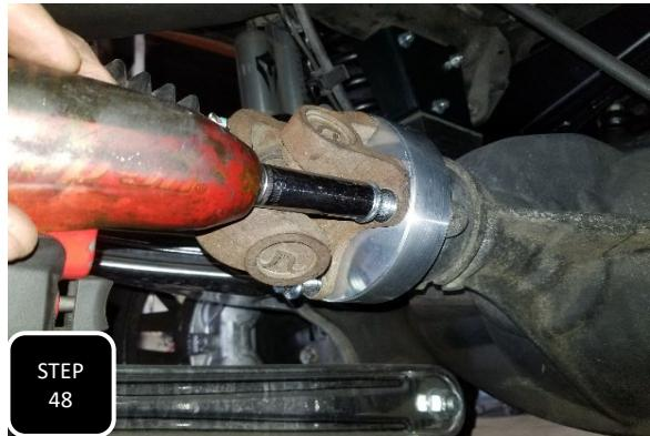
**Step 48** Insert the provided spacer, ensuring that the centering guides seat properly and then loosely install the provided M12-1.75 x 60 flange bolts.
