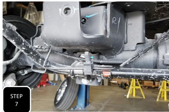
**Step 7** Disengage the guide clip attaching the brake line to the bottom of the trac bar bracket and pull down a bit so it is out of the way.
