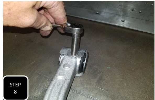
Step 8 Remove the small dust shield around the end of the control arm then locate the new control arm that is shaped just like the one that you took off and install the dust shield on the new control arm using the factory bolts.
