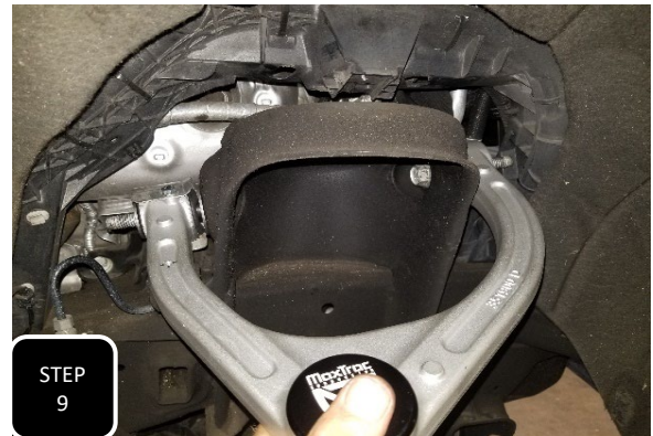
Step 9 Loosely install the new control arm using the factory bolts. NOTE: DO NOT FULLY TIGHTEN THE BOLTS UNTIL THE TRUCK IS ON THE GROUND AT RIDE HEIGHT.
