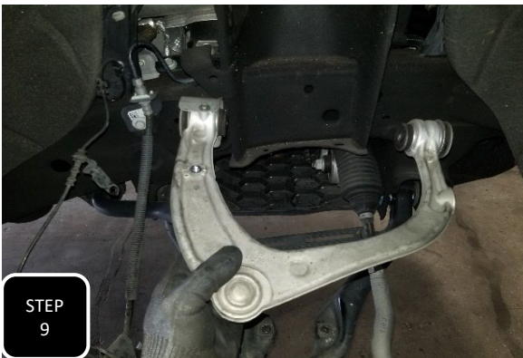
Step 9 Loosely install the new control arm using the factory bolts. NOTE: DO NOT FULLY TIGHTEN THE BOLTS UNTIL THE TRUCK IS ON THE GROUND AT RIDE HEIGHT.
