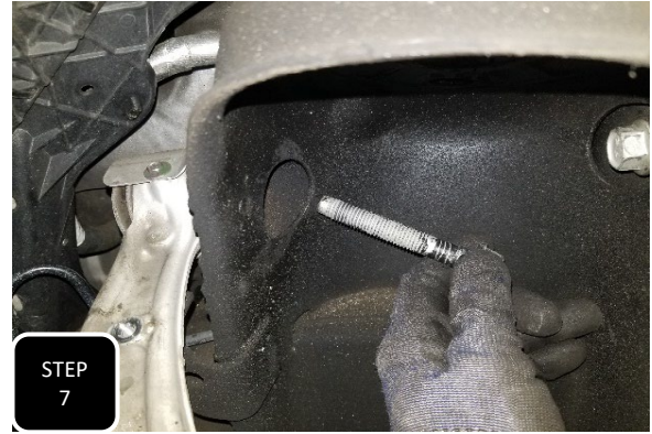
Step 7 Loosen and remove both frame mounting bolts for the upper control arm and then remove the control arm.
