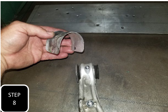
Step 8 Remove the small dust shield around the end of the control arm then locate the new control arm that is shaped just like the one that you took off and install the dust shield on the new control arm using the factory bolts.
